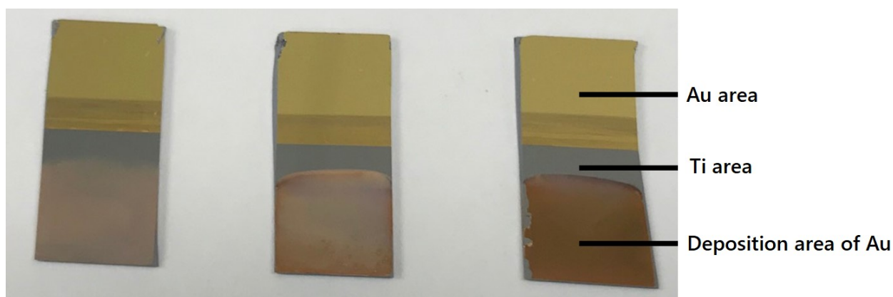
Fig. S10 Photographic images of MHAuNPs deposited at (left) -0.3 V, (middle) -0.6 V, and (right) -0.9 V for 1000 s on Ti/Si substrates.
