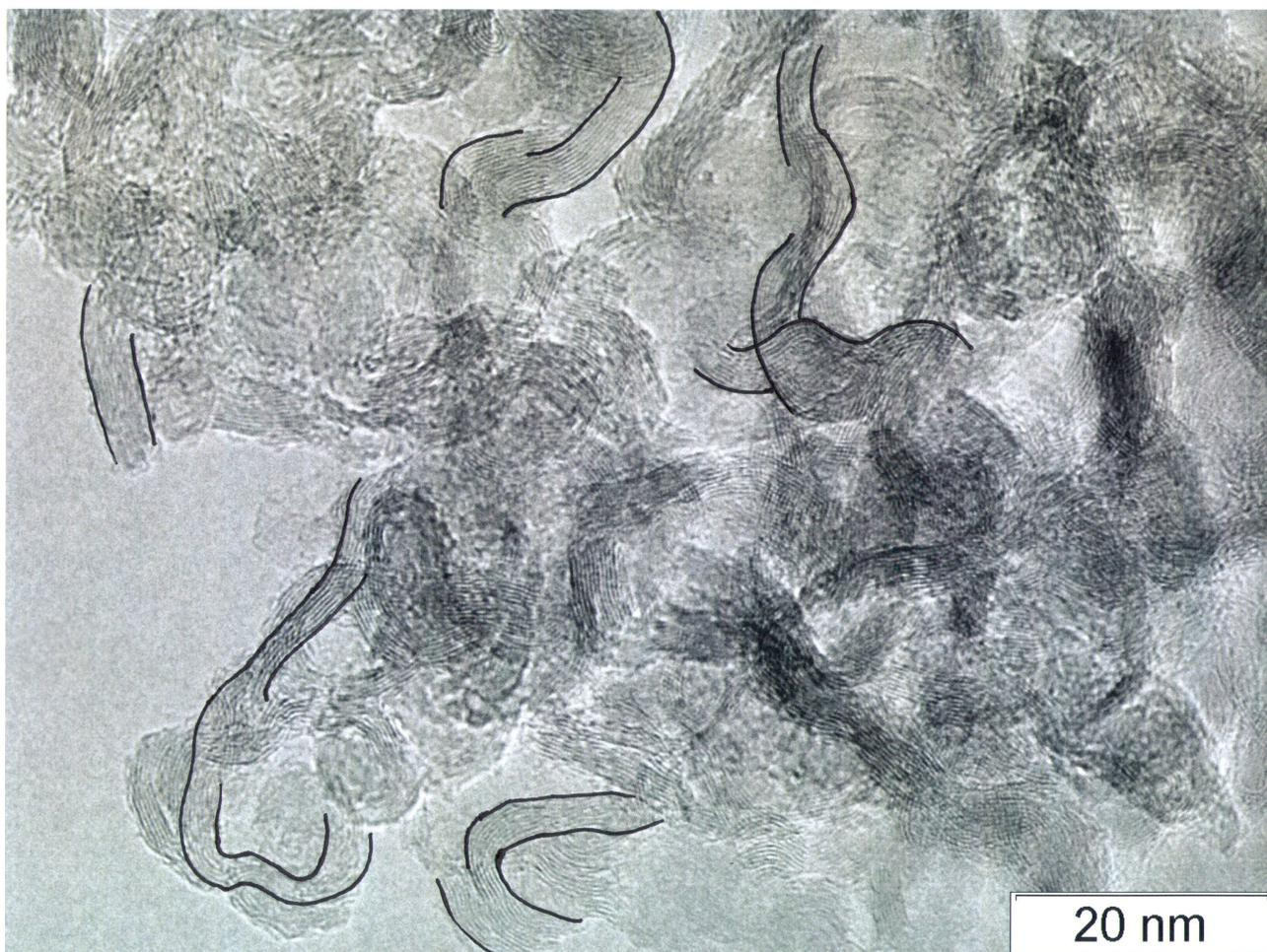
Figure 4. Elongated conductive structures in TATB products, circled in black color.
