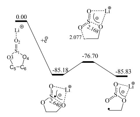
Figure S1. Gibbs free energy profile of Li<sup>+</sup>(ES) with SMD-B3PW91/6311++G(d,p)
