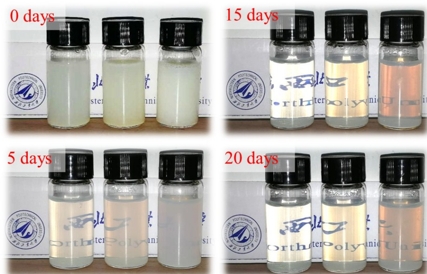
Fig. S6. Status of 10 mg photocatalysts dispersing in 10 mL water after natural sedimentation for different days. (left: CN, middle: CN2, right: CN4).
