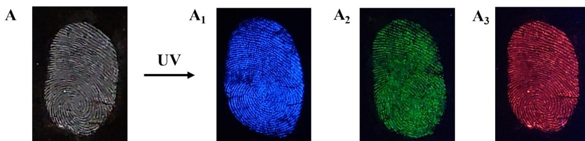
**Fig. S7** Images of latent fingerprints on glass slide by depositing the phosphors under day-light (A) and UV light:
