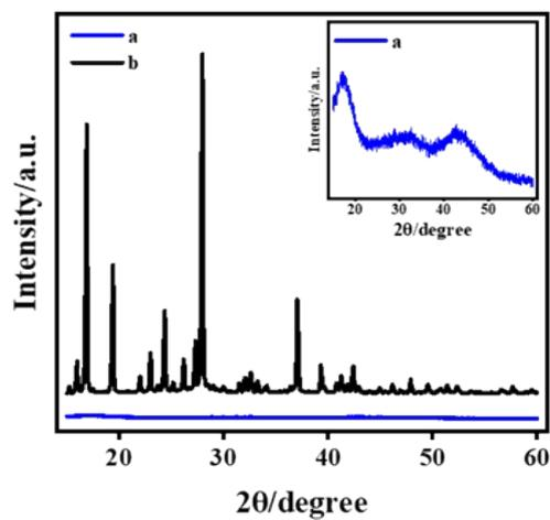
**Fig. S2.** X-ray diffraction spectra of DPA-Ce (a) and DPA (b). Insert: The individual spectra of DPA-Ce.
