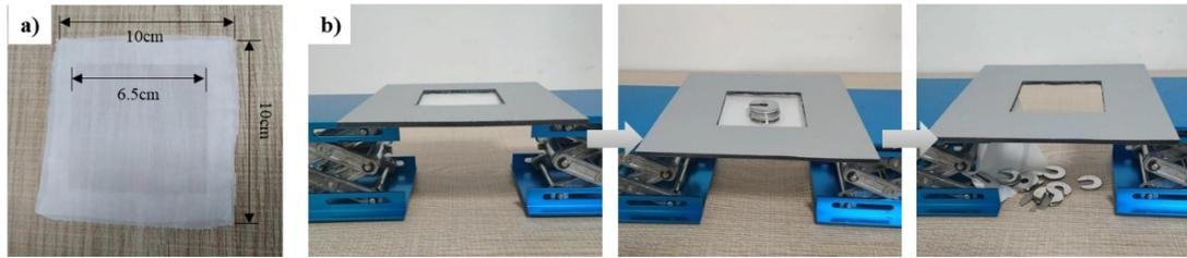
**Figure S8.** a) The test sample model. b) The procedure of bonding force test. The nanofiber composite sample was stick to hand board. The weight is gradually added to sample until the nanofibers are separated from the substrate.
