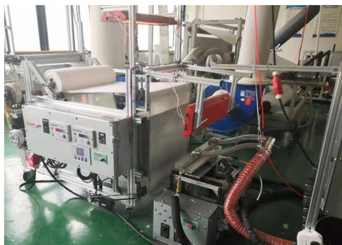
**Figure S1.** The digital image of the continuous production setup for blowspinning
