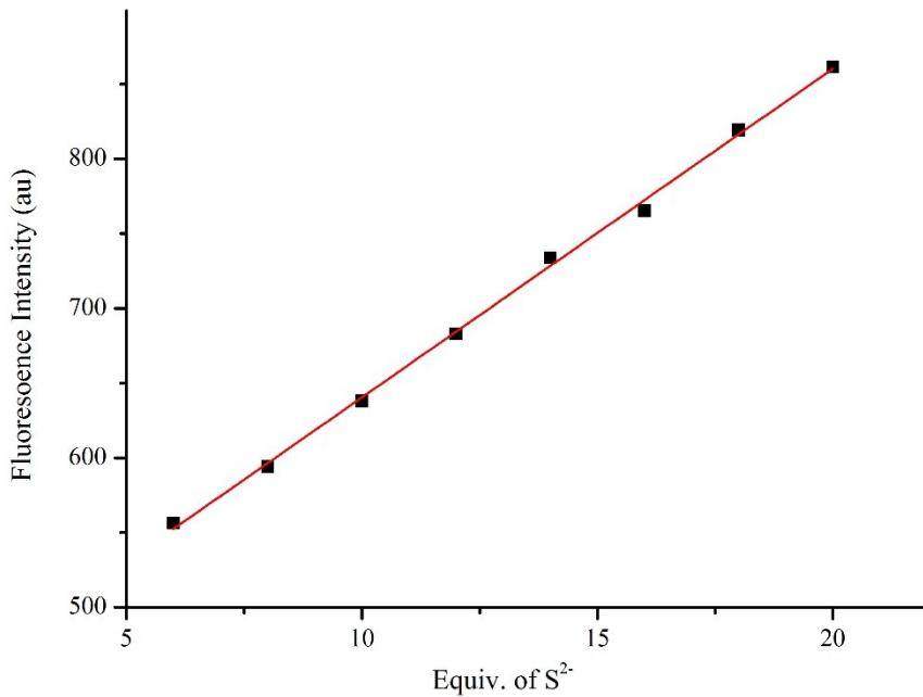
**Fig. S9.** Plot of the intensity at 344 nm for a mixture of DQT-Cd<sup>2+</sup> and S<sup>2-</sup> in CH<sub>3</sub>OH/HEPES (9:1 v/v, pH=7.30) buffer system in the range 6~20 equiv. Linear Equation: Y=21.99×X+420.56, R<sup>2</sup>=0.9983. The detection limit of DQT-Cd<sup>2+</sup> for S<sup>2-</sup> is 11.50 μM.
