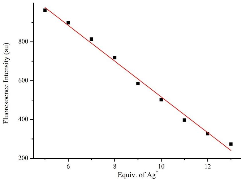
**Fig. S6.** Plot of the intensity at 344 nm for a mixture of probe **DQT** and  $\text{Ag}^+$  in  $\text{CH}_3\text{OH}/\text{HEPES}$  (9:1 v/v, pH=7.30) buffer system in the range 5~13 equiv. Linear Equation:  $Y=-91.99\times X+1436.26$ ,  $R^2=0.9916$ . The calculated detection limit of **DQT** for  $\text{Ag}^+$  is  $0.42 \mu\text{M}$ .
