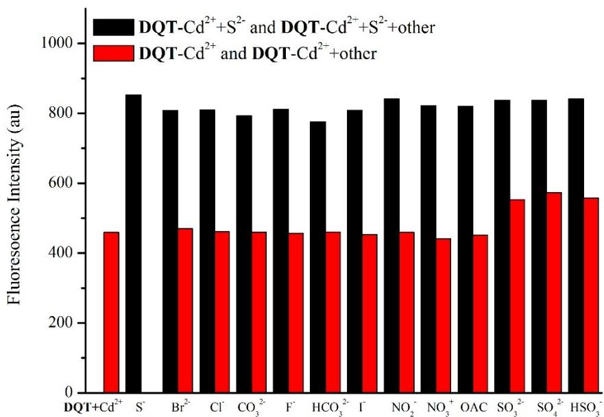
**Fig. S8.** Fluorescence intensity of DQT-Cd<sup>2+</sup> (10 μM) with selected anions (20 equiv.) in the absence (red bars) or presence (black bars) of S<sup>2-</sup> (20 equiv.).
