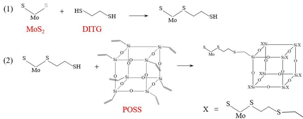
**Fig. S1.** Schematic diagram of the function of DITG in the synthesis of MoS<sub>2</sub>-POSS nanohybrid.
