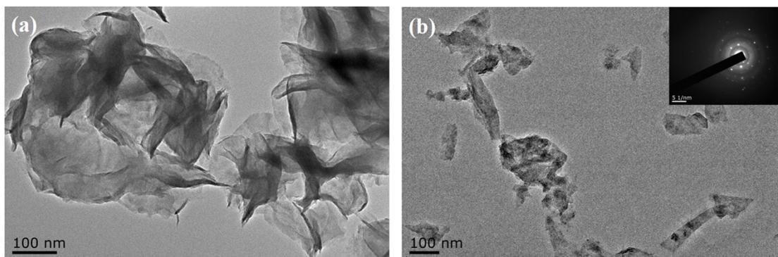
**Fig. S3.** TEM images of (a) bulk MoS<sub>2</sub>, and (b) exfoliated MoS<sub>2</sub>. The inserted picture: selected area electron diffraction (SAED) pattern.
