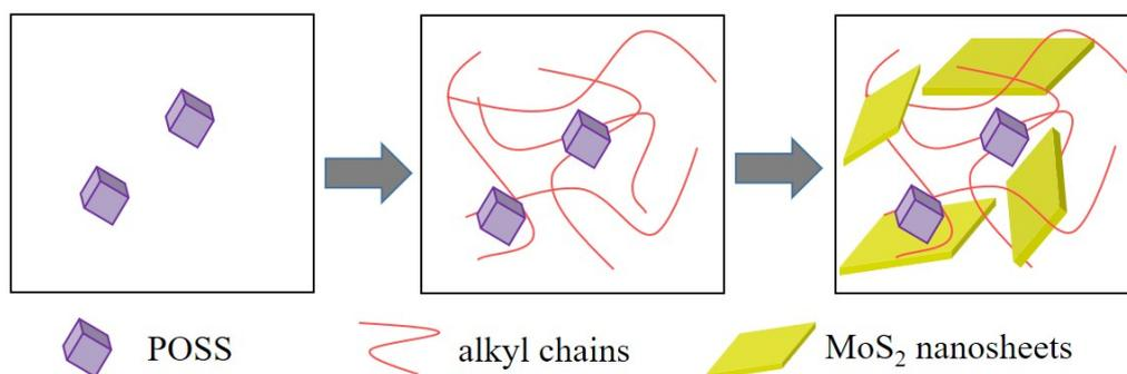
**Fig. S2.** Schematic diagram of formation of porous MoS<sub>2</sub>-POSS nanohybrid.
