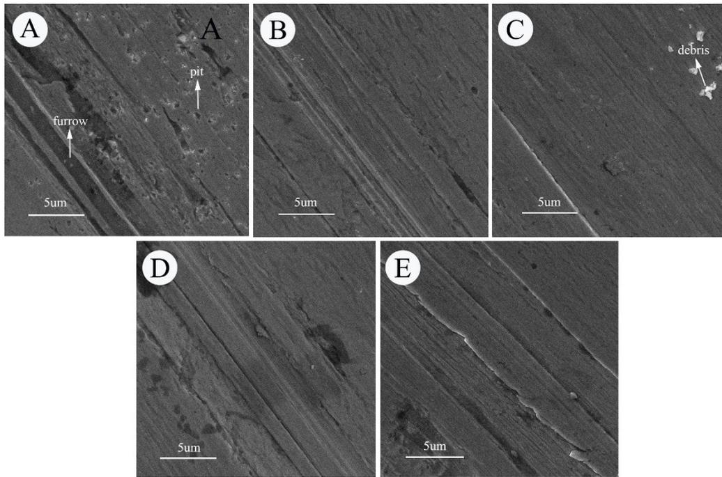
**Fig. S4.** SEM images of the worn surface on the pin lubricated with LP containing: (a) 0.20wt%, (b) 0.40wt%, (c) 0.60wt%, (d) 0.80wt%, and (e) 1.00wt% POSS.
