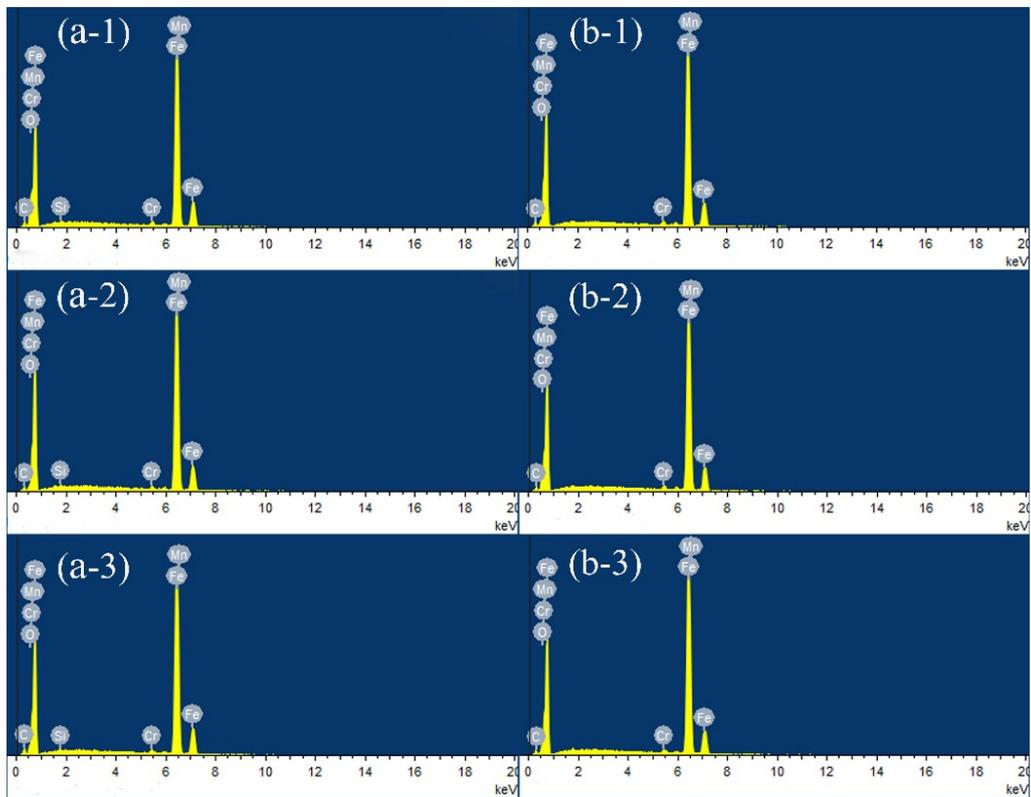
**Fig. S5.** EDS spectra of wear scars for the steel pin lubricated by LP containing (a-1) 0.20wt% POSS, (a-2) 0.60wt% POSS, (a-3) 1.00wt% POSS, (b-1) 0.20wt% MoS<sub>2</sub>, (b-2) 0.60wt% MoS<sub>2</sub>, (b-3) 1.00wt% MoS<sub>2</sub>, respectively.
