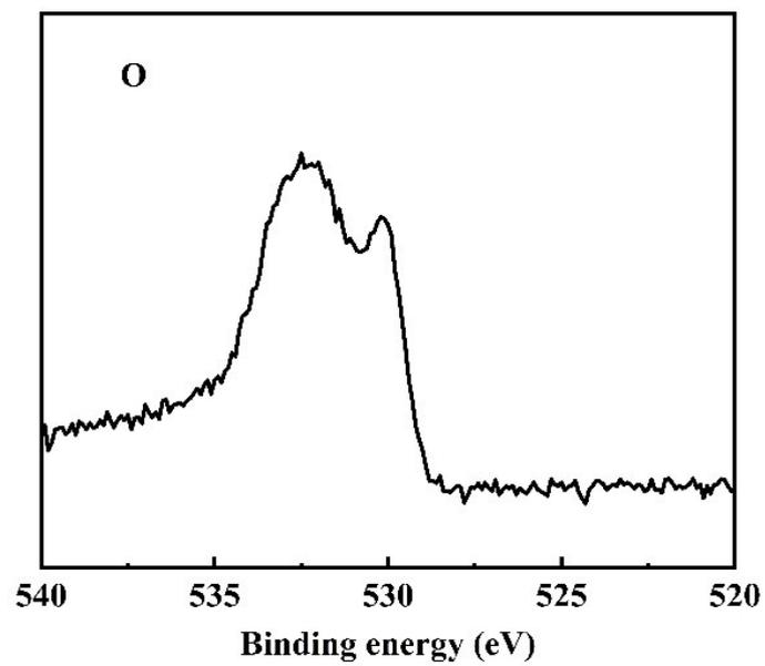
Fig. S2 XPS spectrum of O element of Ag/graphene
