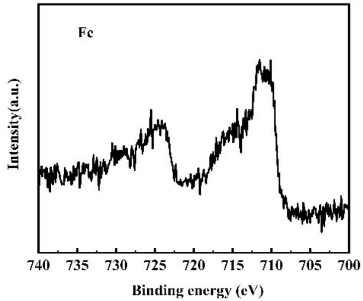
Fig. S1 XPS spectrum of Fe element of Ag/graphene
