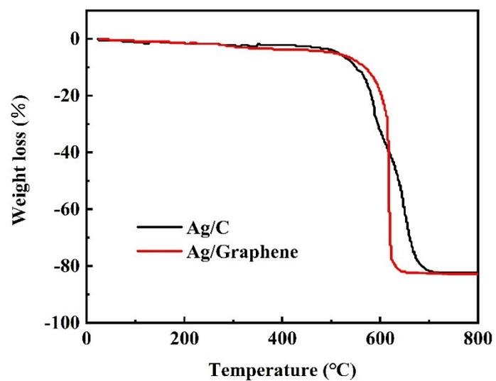
Fig. S3 TG curves of Ag/graphene and Ag/C samples
