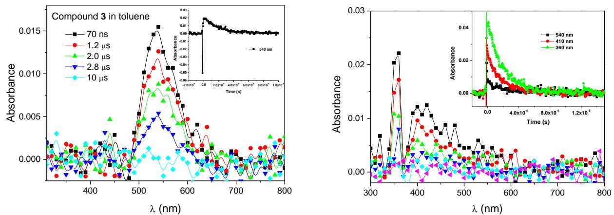
**Fig. S9.** Laser flash photolysis spectra of the dye **3** ( $A = 0.53$  at 355 nm; 2.5 mL) in toluene recorded after irradiation with laser pulses of 355 nm (plot on the left) and in the presence of **B6** (200  $\mu$ L 0.05 M) (plot on the right). Delay times: 2.0  $\mu$ s 2.8  $\mu$ s 4.0  $\mu$ s 6.0  $\mu$ s and 10.0  $\mu$ s.
