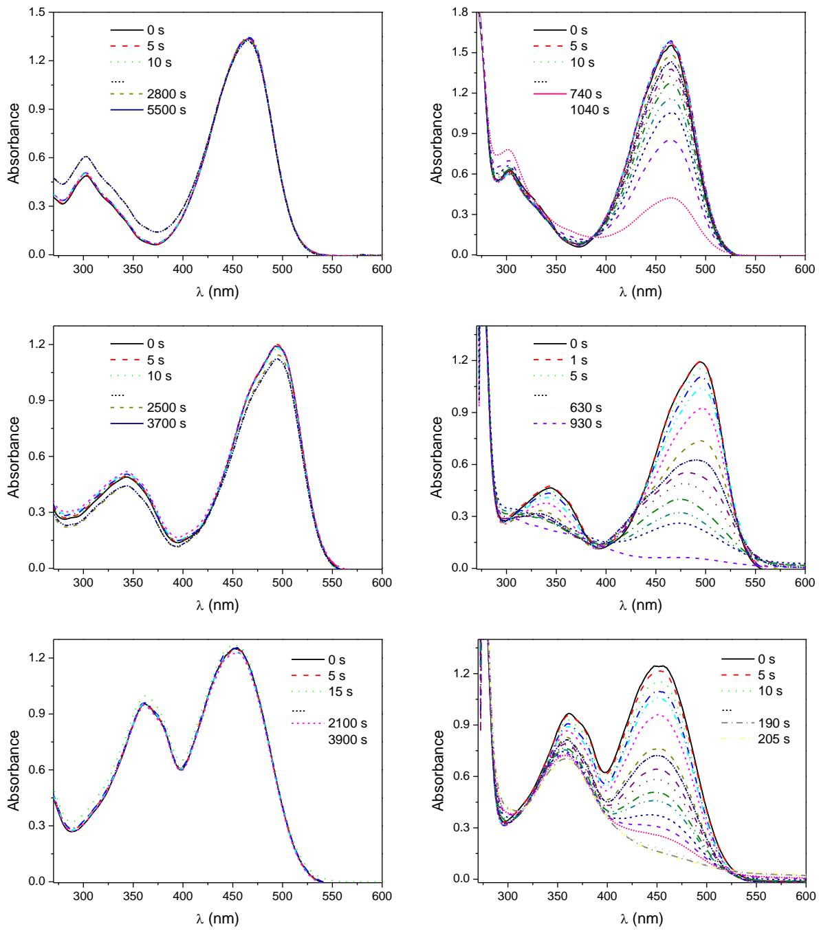
**Fig. S6.** UV-Vis absorption spectra recorded at different irradiation times of the oxazolone derivatives (left panel) and the dye-borate (right panel) in EtOAc upon exposure to the DPSS laser 473 nm; under air; **B6** concentration was 0.0016 M for **1** and 0.029 M for **2** and **3**. From the top: dye **1**, dye **2** and dye **3**.
