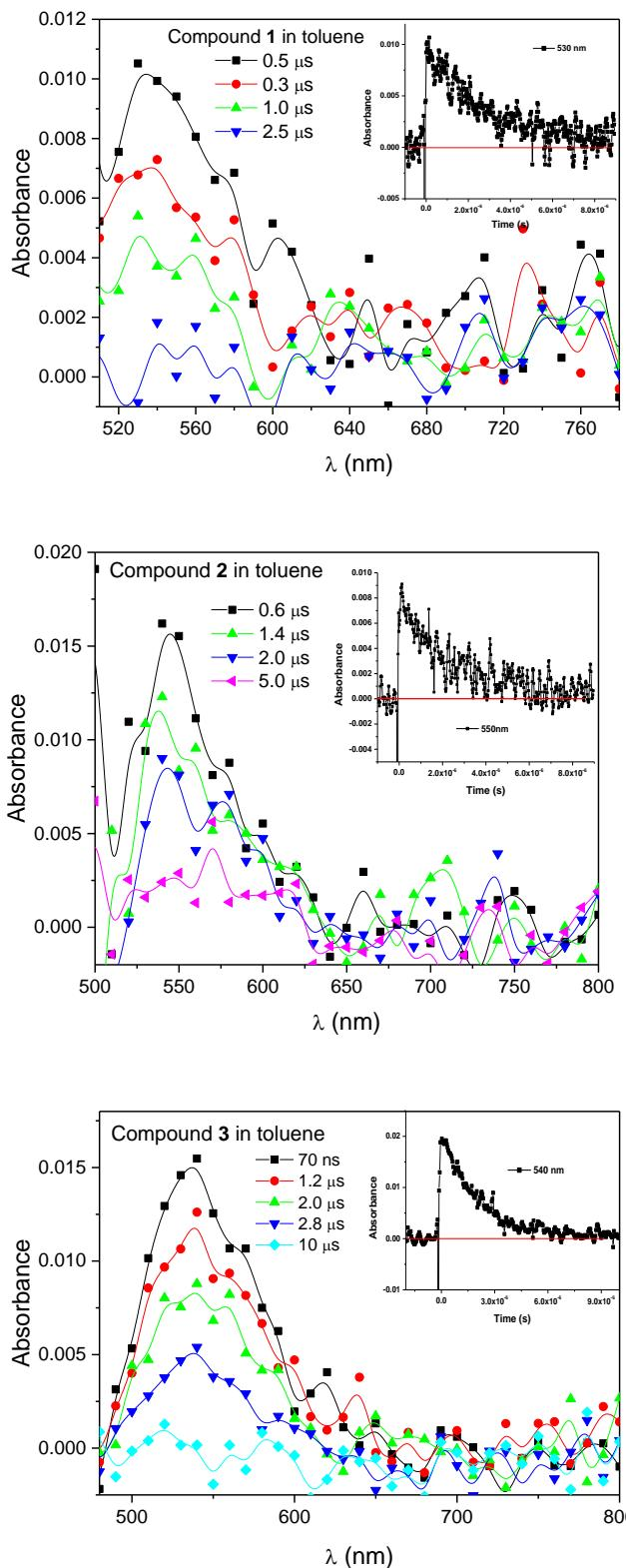
**Fig. S8.** Laser flash photolysis spectra of the dyes in toluene recorded after irradiation with laser pulses of 355 nm. Delay times shown in legends.
