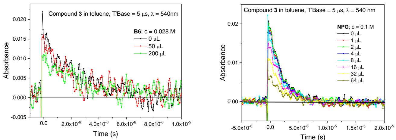
**Fig. S11.** Kinetic curves for the decay of absorbance (540 nm) of **3** in toluene in the presence of the electron donors marked in Figure.
