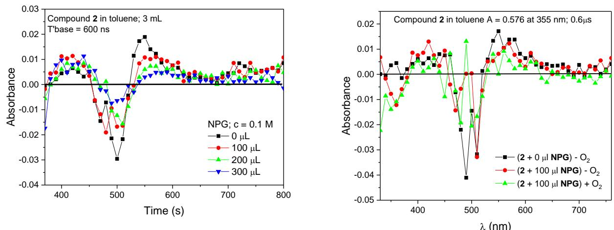
**Fig. S10.** Laser flash photolysis spectra of the dyes **2** and **3** ( $A = 0.5$  at 355 nm; 3 mL) in toluene recorded after irradiation with laser pulses of 355 nm in the presence of N-phenylglycine (**NPG**) (0.1 M) or trimethylammonium phenyltriethylborate (**B6**) (0.028 M). Delay times marked in Figure.
