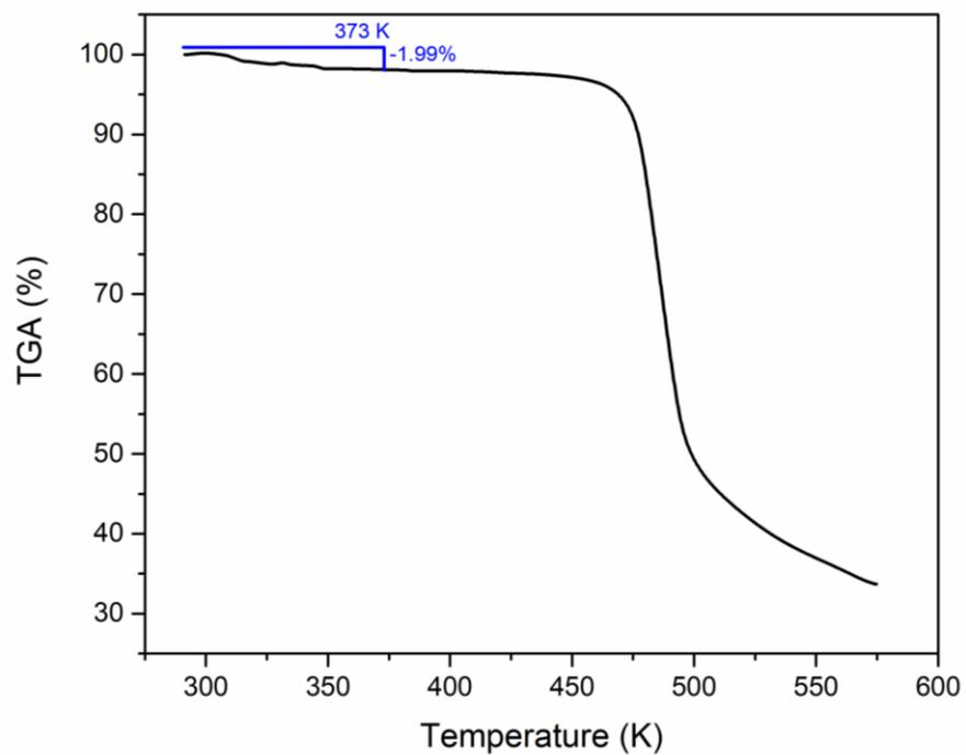
**Figure S4.** TGA of **2** showing the loss of 1.99% of mass up to 100 °C due to evaporation of residual traces of solvents.
