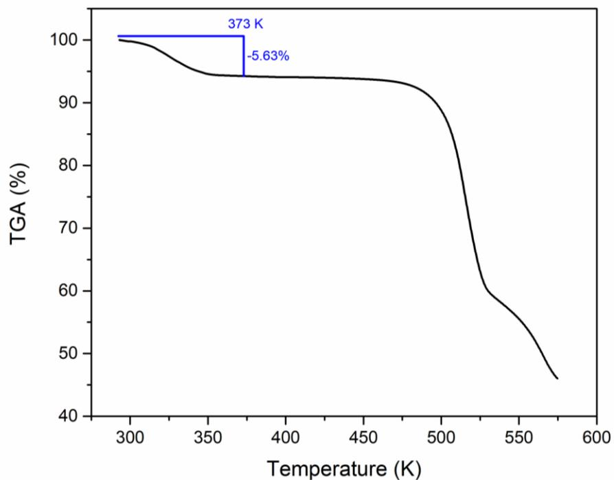
**Figure S3.** TGA of **1** showing the loss of 5.63% of mass up to 100 °C due to evaporation of residual traces of solvents.
