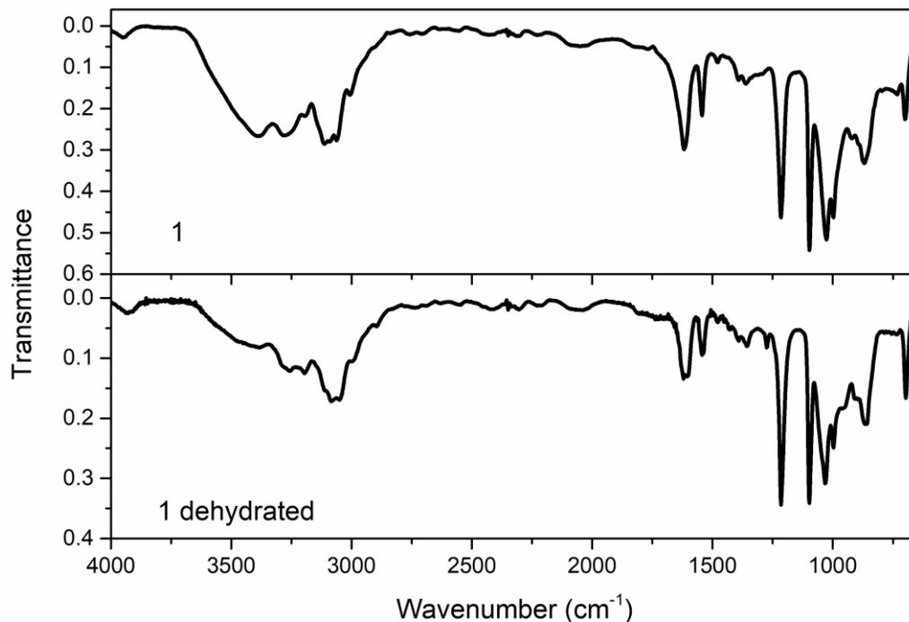
**Figure S1.** IR spectrum of as received (top) and dehydrated (down) sample of **1** recorded using ATR technique at room temperature.
