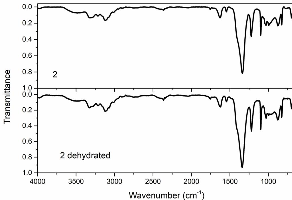
**Figure S2.** IR spectrum of as received (top) and dehydrated (down) sample of **2** recorded using ATR technique at room temperature.
