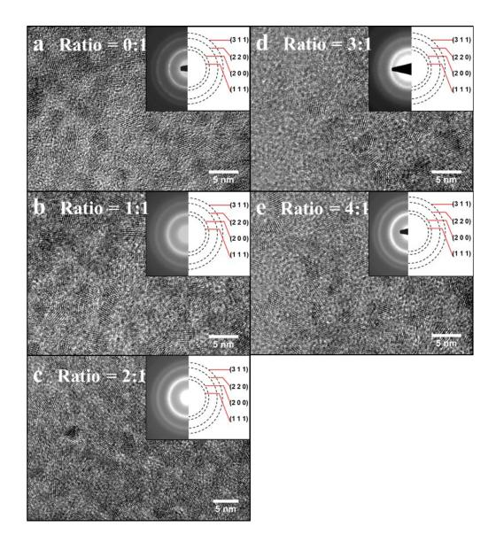
**Fig. S1** TEM images of ceria NPs produced using of reactants ratios (LiOAc and Ce(NO<sub>3</sub>)<sub>3</sub>) of (a) 0:1, (b) 1:1, (c) 2:1, (d) 3:1, and (e) 4:1. (insets) Indexed corresponding SAED patterns.
