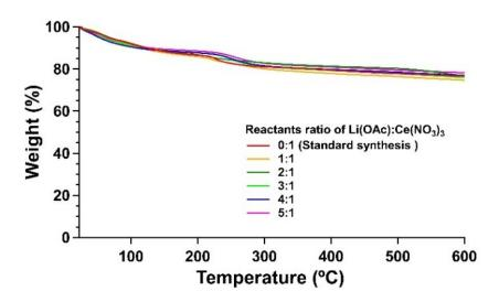
**Fig. S2** TGA results for ceria NPs produced using LiOAc and Ce(NO<sub>3</sub>)<sub>3</sub> reactants with ratios of 0:1, 1:1, 2:1, 3:1, 4:1, and 5:1.
