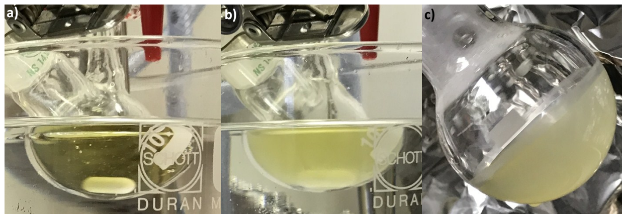
Figure S35: After addition of 1,3-propanediol to the Ti(IV) acetylacetonate solution (a), 12 hours after 1,3-propanediol addition (b), and after removal of isopropanol and ethanol (c). In contrast to the Ta(V) solutions, the Ti(IV) solution turns turbid over time at room temperature.
