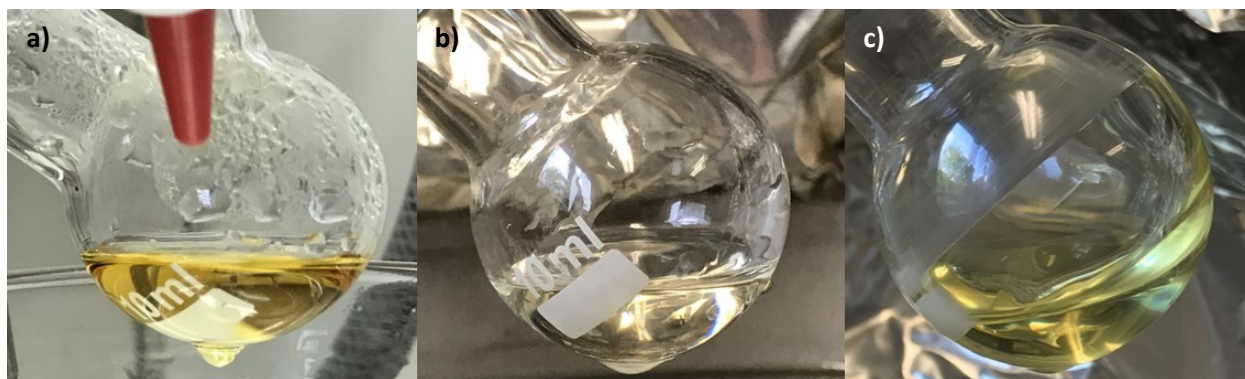
Figure S25: Final solution products from method based on Calzada and González with acetylacetone (a), the proposed method with acetylacetone (b), and the proposed method with benzoylacetone (c). (a) has an enhanced color when compared to (b) – this may be caused by light scattering from nanoparticle formation by alcoholysis in (a). (c) appears redshifted relative to (b).
