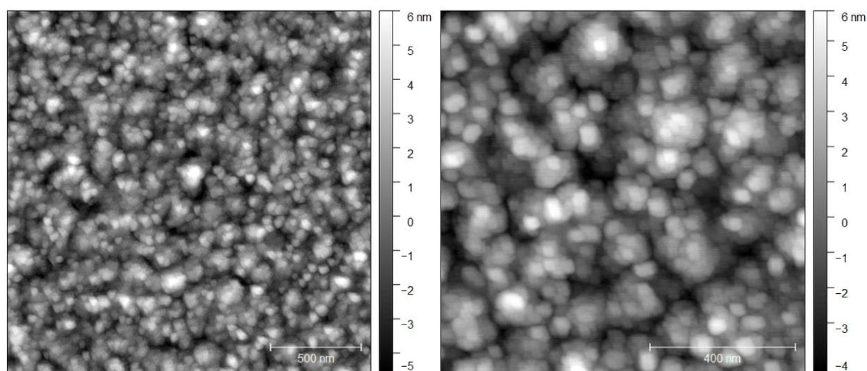
**Figure S5.** AFM images of  $\text{Sb}_2\text{Te}_3$  - *Substrate Annealing* (2) films.
