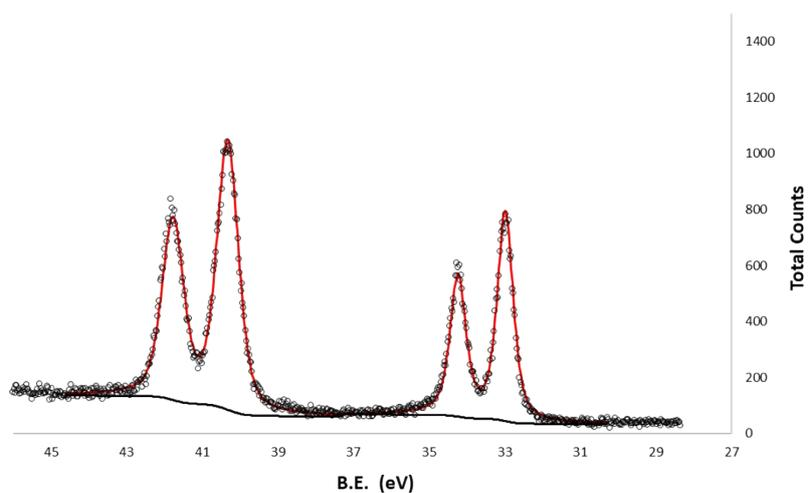
**Figure S19.** Te and Sb 4d XPS of  $\text{Sb}_2\text{Te}_3$  - *Substrate Annealing* (3). Te  $4d_{5/2}$ : 40.3 eV ( $\Delta = 1.5$  eV); Sb  $4d_{5/2}$ : 33.0 eV, ( $\Delta = 1.3$  eV).
