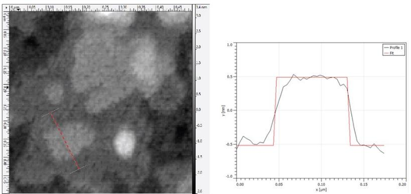
**Figure S8.** Selected surface profile of  $\text{Sb}_2\text{Te}_3$  - *Post-Growth Annealing* (3); Step height: 1 nm.
