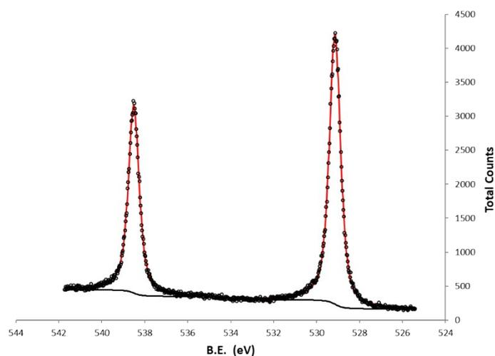
**Figure S21.** Sb 3d XPS of  $\text{Sb}_2\text{Te}_3$  - *Post-Growth Annealing* (3). Sb  $3d_{5/2}$ : 529.1 eV ( $\Delta = 9.35$  eV).
