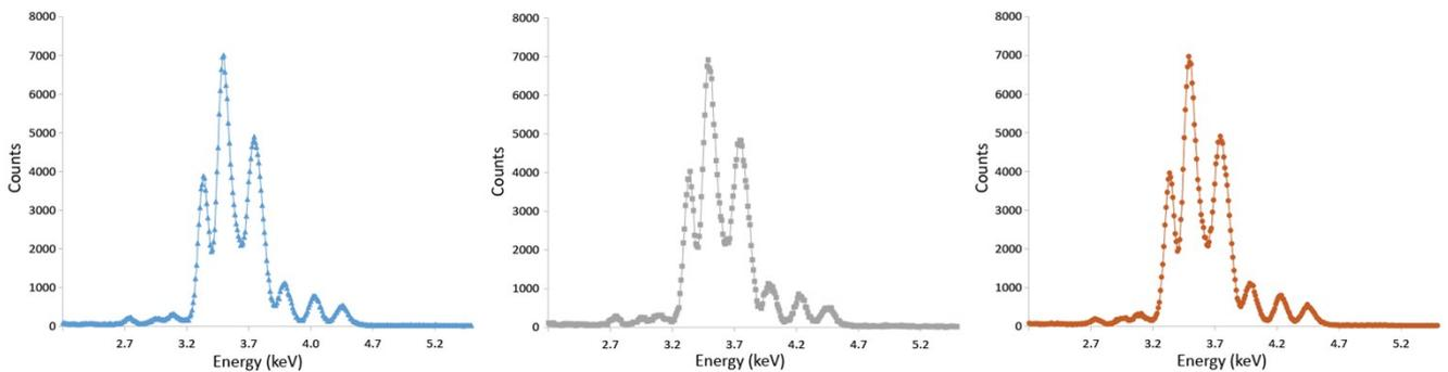
**Figure S12.** TXRF Spectra of  $\text{Sb}_2\text{Te}_3$  - *As Deposited* (1) (blue, left),  $\text{Sb}_2\text{Te}_3$  - *Substrate Annealing* (2) (grey, middle), and of  $\text{Sb}_2\text{Te}_3$  - *Post-Growth Annealing* (3) (red, right).
