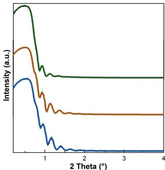
**Figure S23.** XRR measurements of  $\text{Sb}_2\text{Te}_3$  - *As Deposited* (1) (black, top),  $\text{Sb}_2\text{Te}_3$  - *Substrate Annealing* (2) (red, middle), and of  $\text{Sb}_2\text{Te}_3$  - *Post-Growth Annealing* (3) (blue, bottom).
