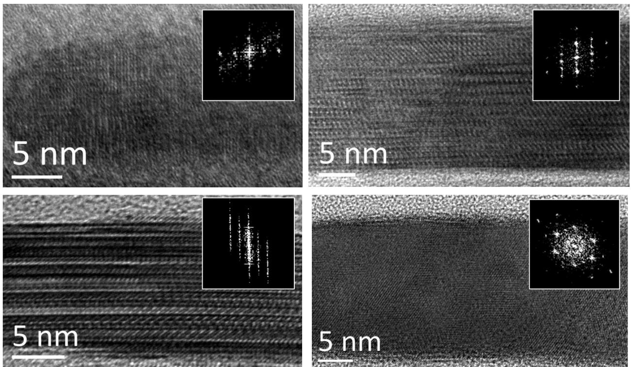
**Figure S10.** TEM images and related FFTs of  $\text{Sb}_2\text{Te}_3$  - *Substrate Annealing* (2) films: examples of the variability in the crystallographic orientations of some different grains.
