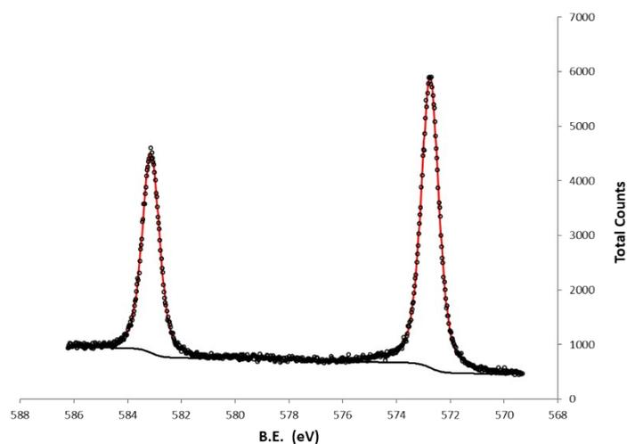
**Figure S20.** Te 3d XPS of  $\text{Sb}_2\text{Te}_3$  - *Post-Growth Annealing* (3). Te  $3d_{5/2}$ : 572.7 eV ( $\Delta = 10.4$  eV).
