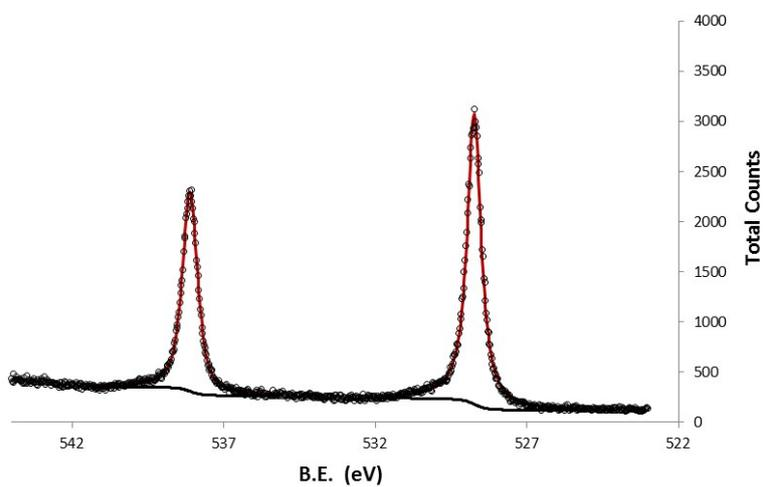
**Figure S15.** Sb 3d XPS of  $\text{Sb}_2\text{Te}_3$  - As Deposited (1). Sb  $3d_{5/2}$ : 529.0 eV ( $\Delta = 9.35$  eV).
