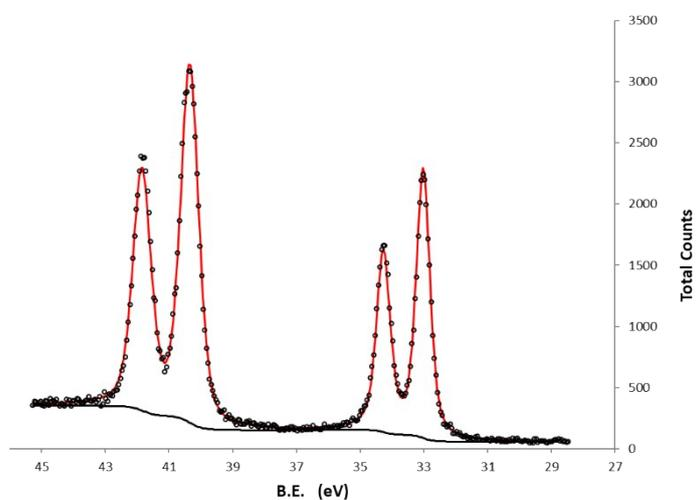
**Figure S22.** Te and Sb 4d XPS of  $\text{Sb}_2\text{Te}_3$  - *Post-Growth Annealing* (3). Te  $4d_{5/2}$ : 40.3 eV ( $\Delta = 1.5$  eV); Sb  $4d_{5/2}$ : 33.0 eV, ( $\Delta = 1.2$  eV).
