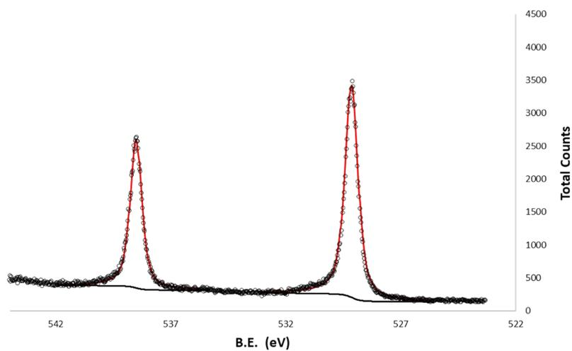
**Figure S18.** Sb 3d XPS of  $\text{Sb}_2\text{Te}_3$  - *Substrate Annealing* (3). Sb  $3d_{5/2}$ : 529.1 eV ( $\Delta = 9.4$  eV).
