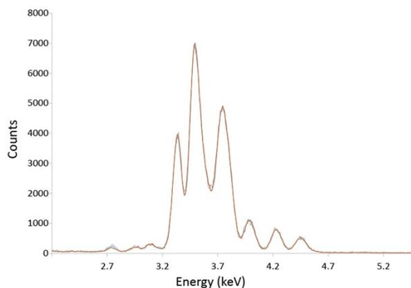
**Figure S13.** Overlap of the TXRF Spectra shown in Figure S12 indicating the same elemental composition in 1, 2, 3.
