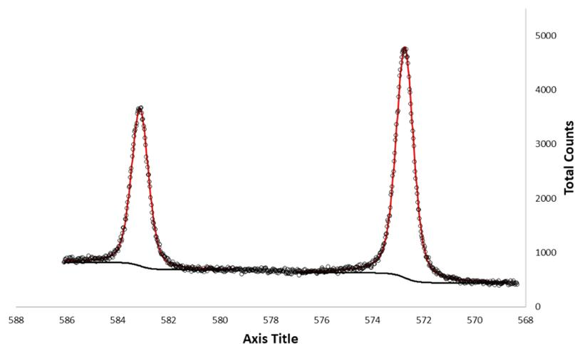
**Figure S17.** Te 3d XPS of  $\text{Sb}_2\text{Te}_3$  - *Substrate Annealing* (3). Te  $3d_{5/2}$ : 572.7 eV ( $\Delta = 10.4$  eV).
