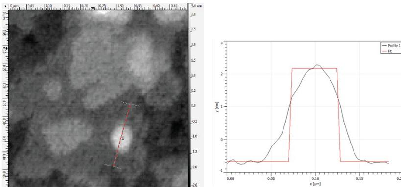
**Figure S7.** Selected surface profile of  $\text{Sb}_2\text{Te}_3$  - *Post-Growth Annealing* (3); Step height: 3 nm.
