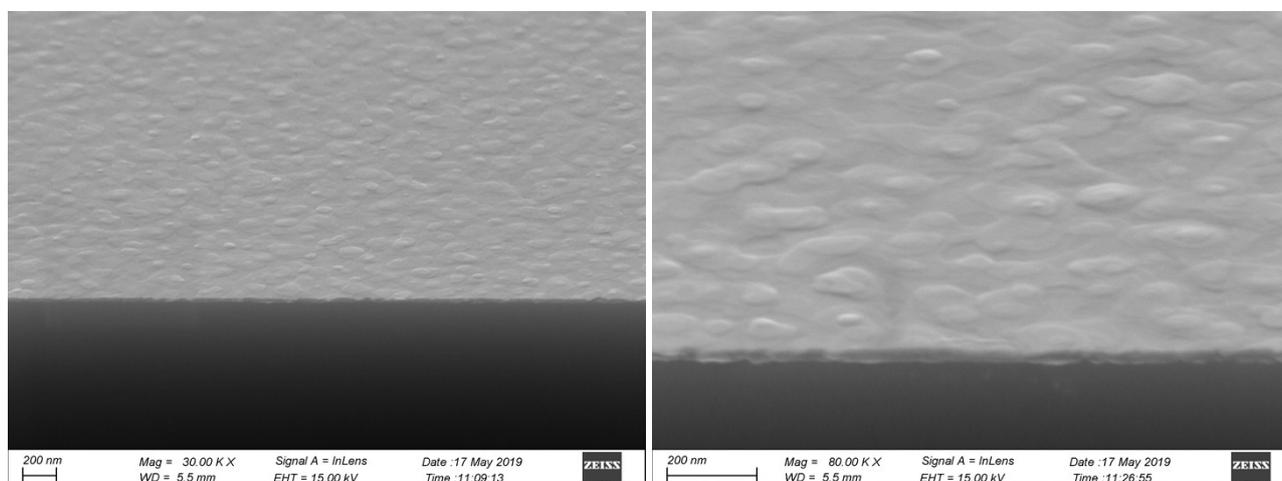
**Figure S3.** Tilted cross-section SEM images of  $\text{Sb}_2\text{Te}_3$  - *Post-Growth Annealing (3)* films.
