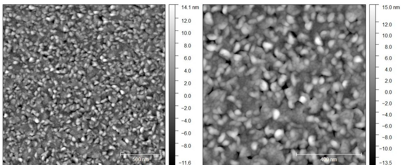
**Figure S4.** AFM images of  $\text{Sb}_2\text{Te}_3$  - *As Deposited* (1) films.
