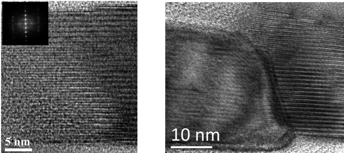
**Figure S11.** High resolution TEM images of  $\text{Sb}_2\text{Te}_3$  - *Post-Growth Annealing* (3) film. Left: the quintuple stack of the  $\text{Sb}_2\text{Te}_3$  rhombohedral crystalline structure (R -3m space group); the stacking period, measured from the FFT in the inset, is 1 nm. Right: the boundary between two grains.
