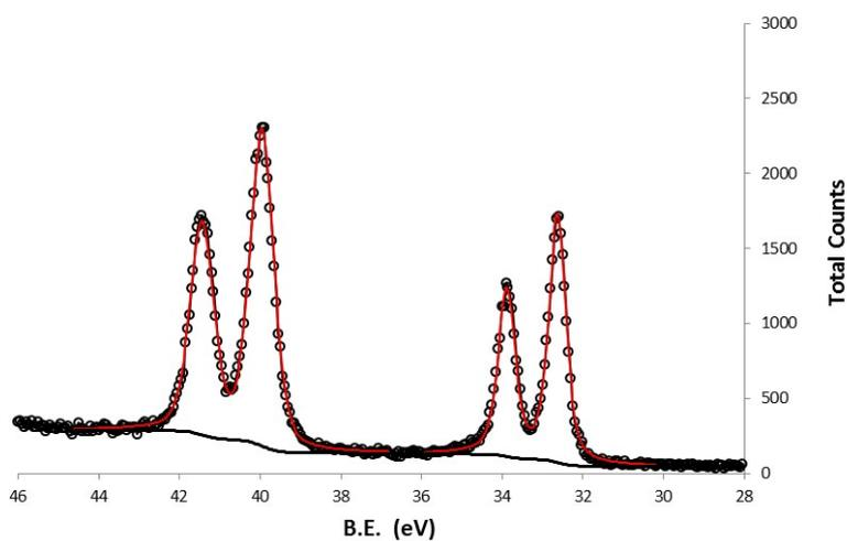
**Figure S16.** Te and Sb 4d XPS of  $\text{Sb}_2\text{Te}_3$  - As Deposited (1). Te  $4d_{5/2}$ : 40.2 eV ( $\Delta = 1.5$  eV); Sb  $4d_{5/2}$ : 32.9 eV, ( $\Delta = 1.2$  eV).
