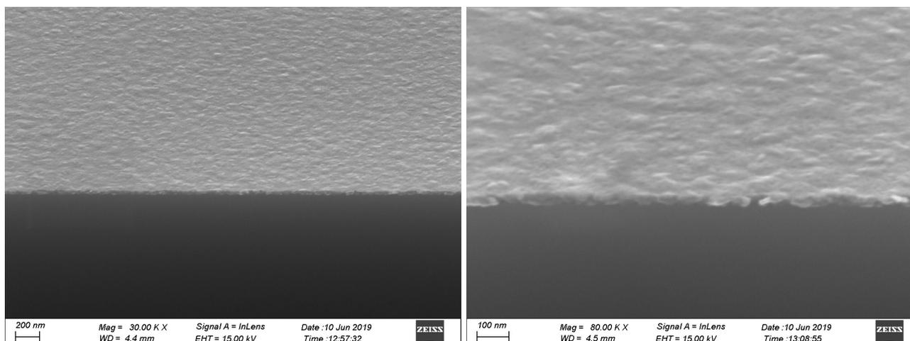
**Figure S2.** Tilted cross-section SEM images of  $\text{Sb}_2\text{Te}_3$  - *Substrate Annealing (2)* films.
