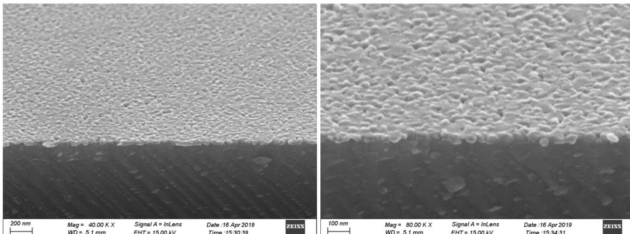
**Figure S1.** Tilted cross-section SEM images of  $\text{Sb}_2\text{Te}_3$  - *As Deposited (1)* films.
