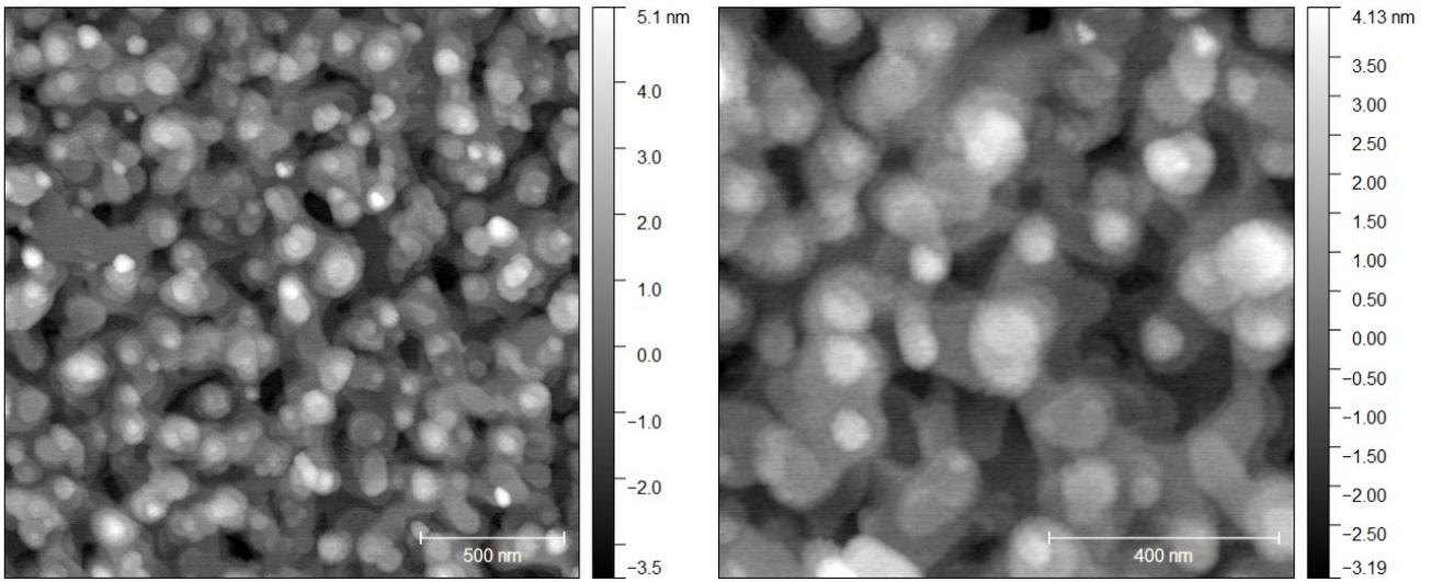
**Figure S6.** AFM images of  $\text{Sb}_2\text{Te}_3$  - *Post-Growth Annealing* (3) films.
