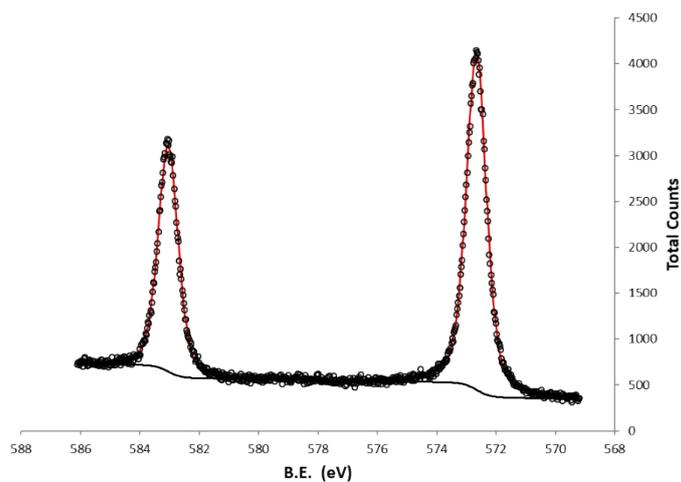
**Figure S14.** Te 3d XPS of  $\text{Sb}_2\text{Te}_3$  - As Deposited (1). Te  $3d_{5/2}$ : 572.6 eV ( $\Delta = 10.4$  eV).
