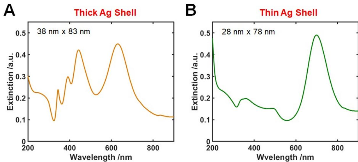
**Fig. S3** UV-Vis extinction spectra of Ag@AuNRs with thick Ag shell in water (**A**) and Ag@AuNRs with thin Ag shell dispersed in water (**B**).
