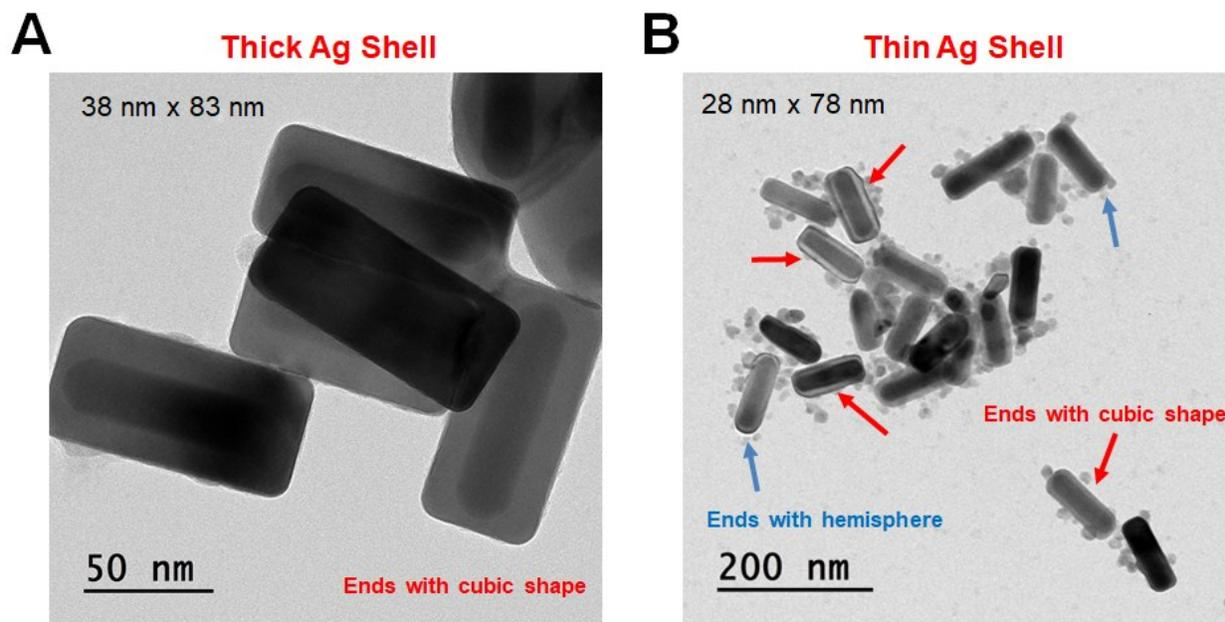
**Fig. S1 (A)** TEM image of single Ag@AuNRs with thick shell thickness, and they had a cubic shape at the ends. **(B)** TEM image of single Ag@AuNRs with thin shell thickness. Some of thin Ag@AuNRs have a cubic shape at the ends (indicated by red-arrow), whereas some of thin Ag@AuNRs have a shape of hemisphere at the ends (indicated by blue-arrow). But, from a TEM analysis using many particles, we found that a majority of thin Ag@AuNRs had the cubic shape at their ends.
