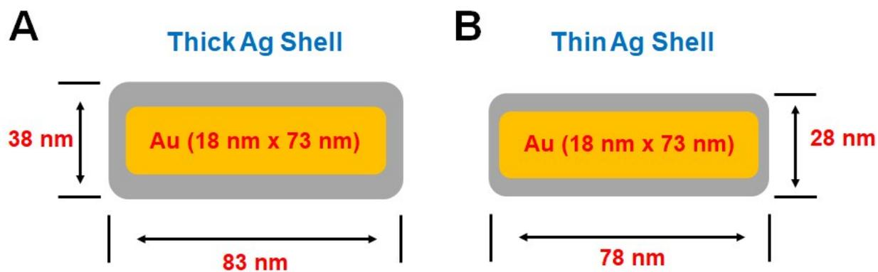
**Fig. S2** Schematics to show the size and dimensions of Ag@AuNRs with two different Ag shell thickness. **(A)** Dimension of Ag@AuNR with thick Ag shell thickness at the same size of AuNR core. **(B)** Dimension of Ag@AuNR with thin shell thickness at the same size of AuNR core.
