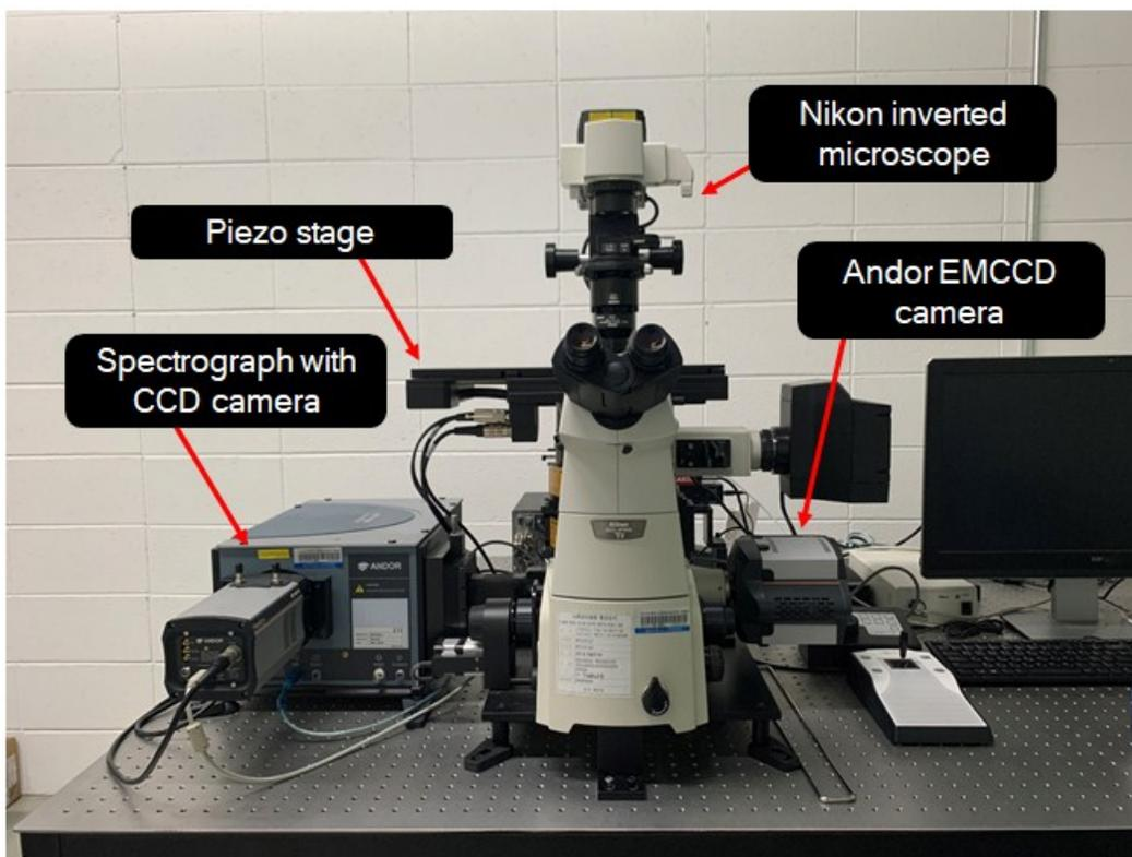
**Fig. S4** A photograph to show the experimental setup for single particle DF microscopy and spectroscopy.
