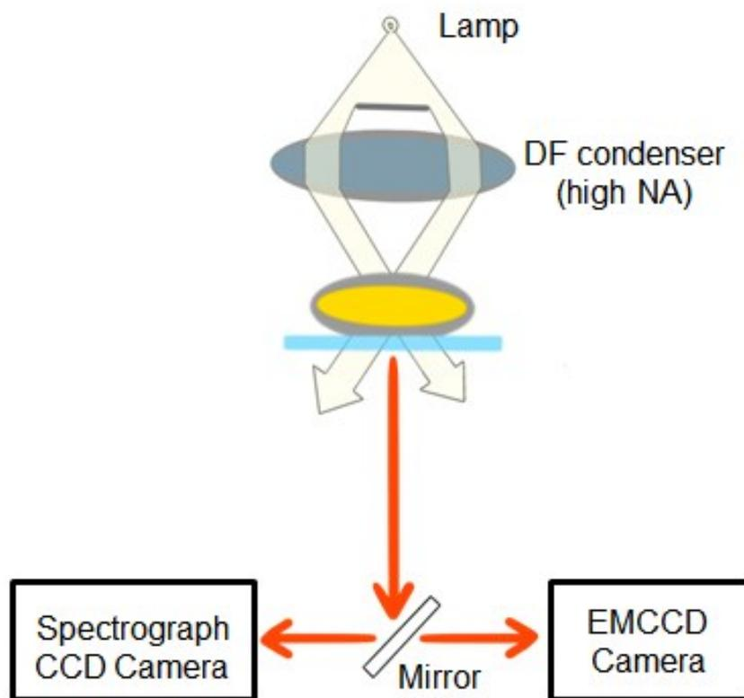
**Fig. S5** Schematic depicting the working principle of scattering-based DF microscopy and spectroscopy.
