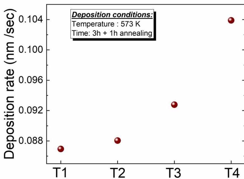
S1. Deposition rates of the  $\text{CoSb}_3$  doped Te thin films (T1, T2, T3, and T4)
