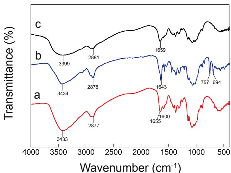
**Figure S3.** FTIR spectra of (a) CsNFs, (b) CsNFs after the fifth run of recycling test, and (c) chitosan powder.
