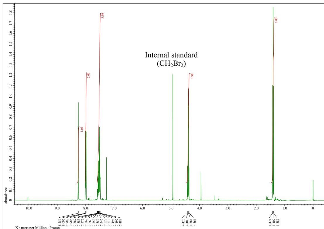
**Figure S5.** <sup>1</sup>H NMR spectrum of crude reaction product of a gram-scale reaction (Scheme 2).
