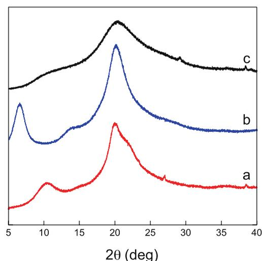
**Figure S2.** XRD patterns of (a) CsNFs, (b) CsNFs after the fifth run of recycling test, and (c) chitosan powder.
