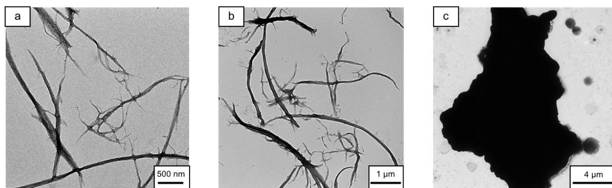
**Figure S1.** TEM images of (a) chitosan nanofibers (CsNFs), (b) CsNFs after the fifth run of recycling test, and (c) chitosan powder.
