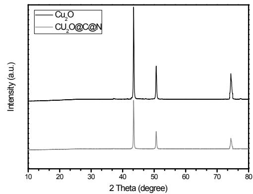
Figure S3. XRD pattern of Cu<sub>2</sub>O microspheres and Cu<sub>2</sub>O@C@N ( before template etching to remove Cu ).
