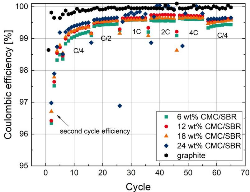
Figure S4: Coulombic efficiencies of Si/C graphite blend anodes in dependence of the binder and C-rate in CCCV cycling setup.
