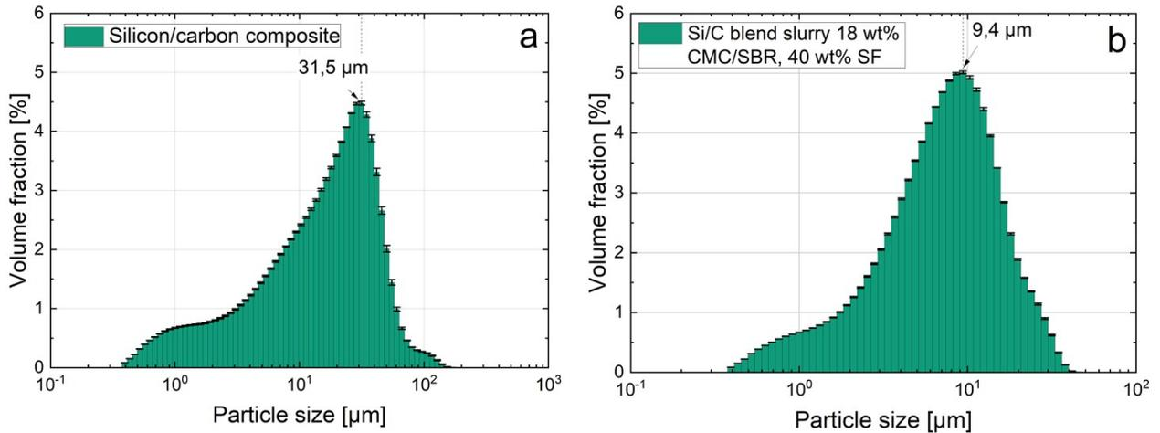
Figure S3 Particle size distribution of a) the Si/C composite after ball milling and b) a slurry containing 18 wt% CMC/SBR binder and 40 wt% solid fraction after the three roll process.
