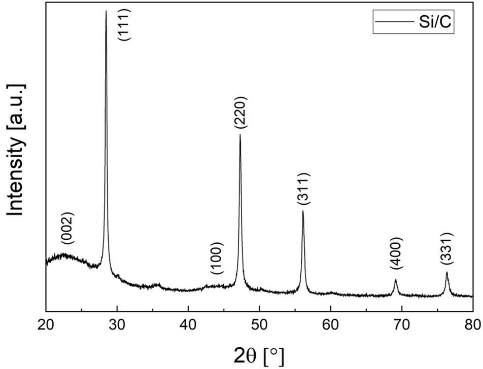
Figure S2: XRD pattern of Si/C anode material. The peaks refer to the reflection planes of the carbon and the silicon crystal.
