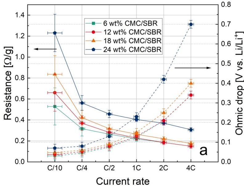
Figure S5: Ohmic drop of Si/C graphite blend anode based lithium metal cells between CC charge and CC discharge and corresponding internal resistance.
