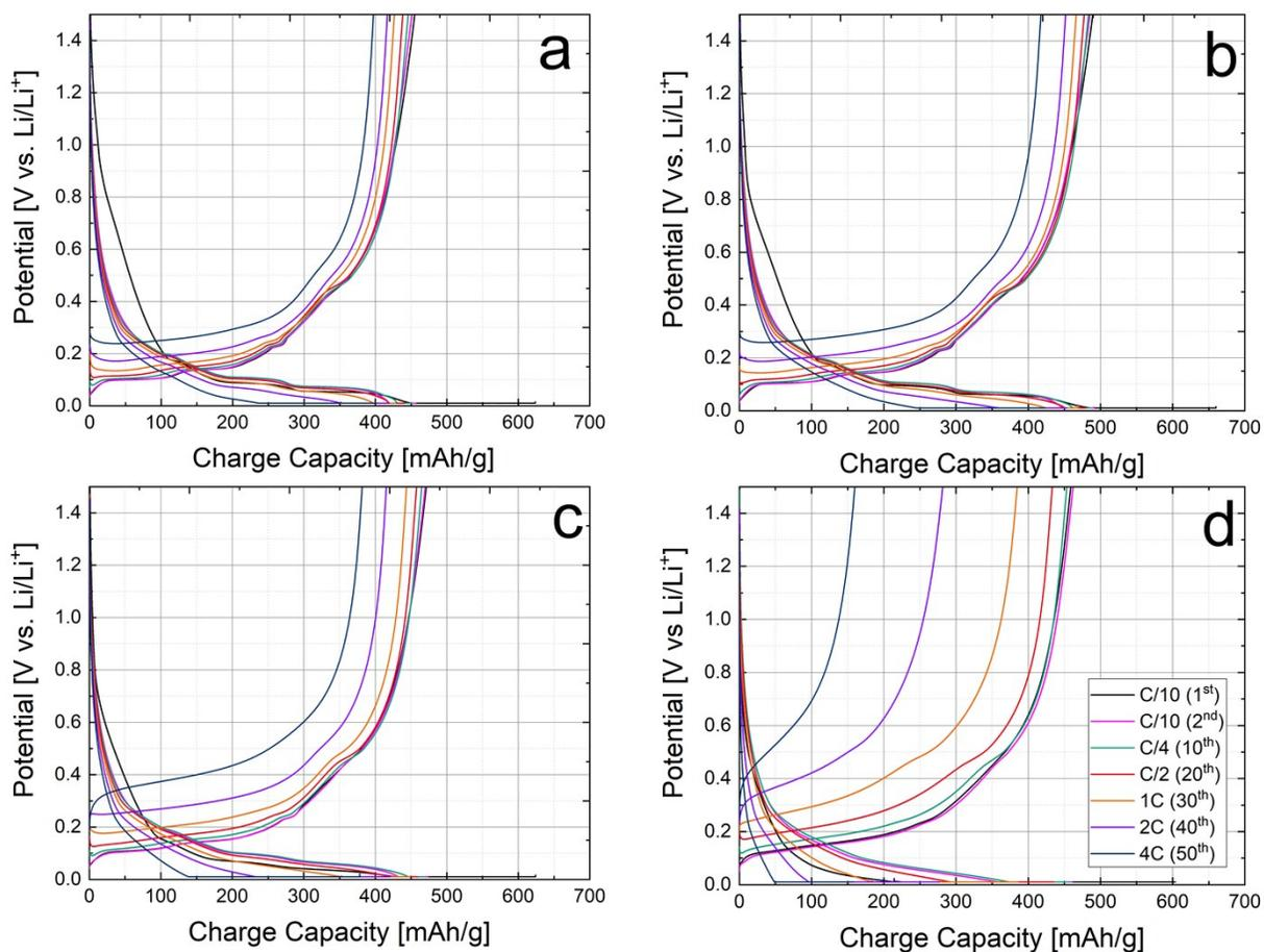
Figure S6: Voltage profile of Si/C Graphite blend anodes with a) 6 wt%, b) 12 wt%, c) 18 wt% and d) 24 wt% CMC/SBR binder in dependence of the current rate. Legend is the same for d-a. Number of the cycle is given in parentheses.
