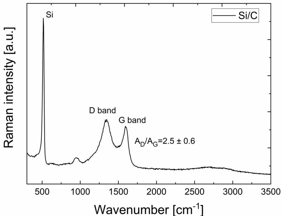
Figure S1: Raman spectra of Si/C anode material in the range between 300 and 3500 cm<sup>-1</sup>.
