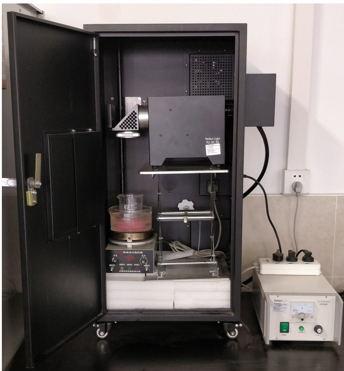
Fig. S2. A photo of the photocatalysis reaction setup.
