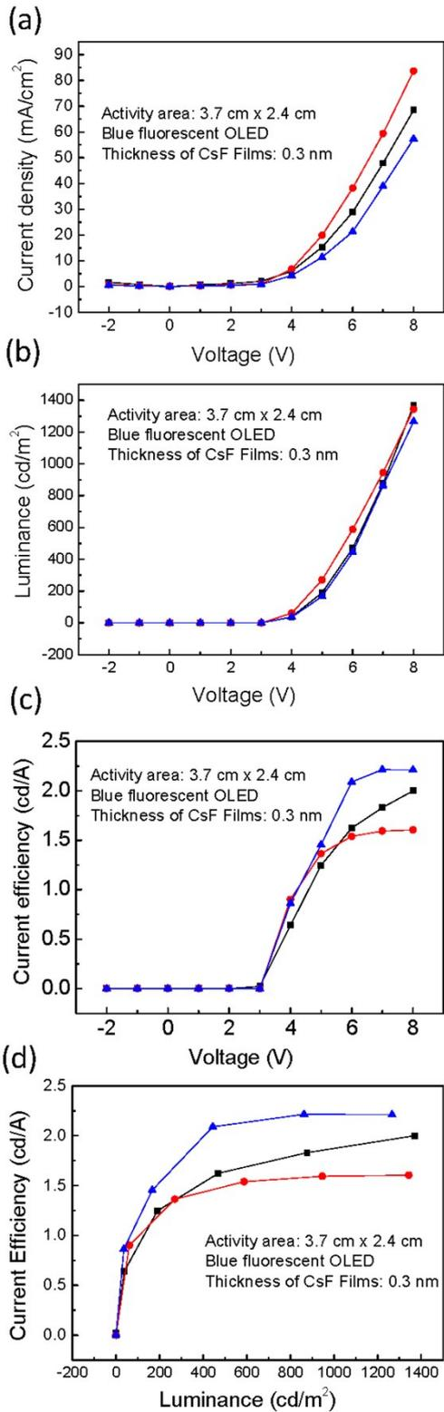
Figure S10 The current density versus voltage, the luminance versus voltage, current efficiency versus voltage, and the current efficiency versus luminance of blue OLED devices with 0.3 nm CsF.
