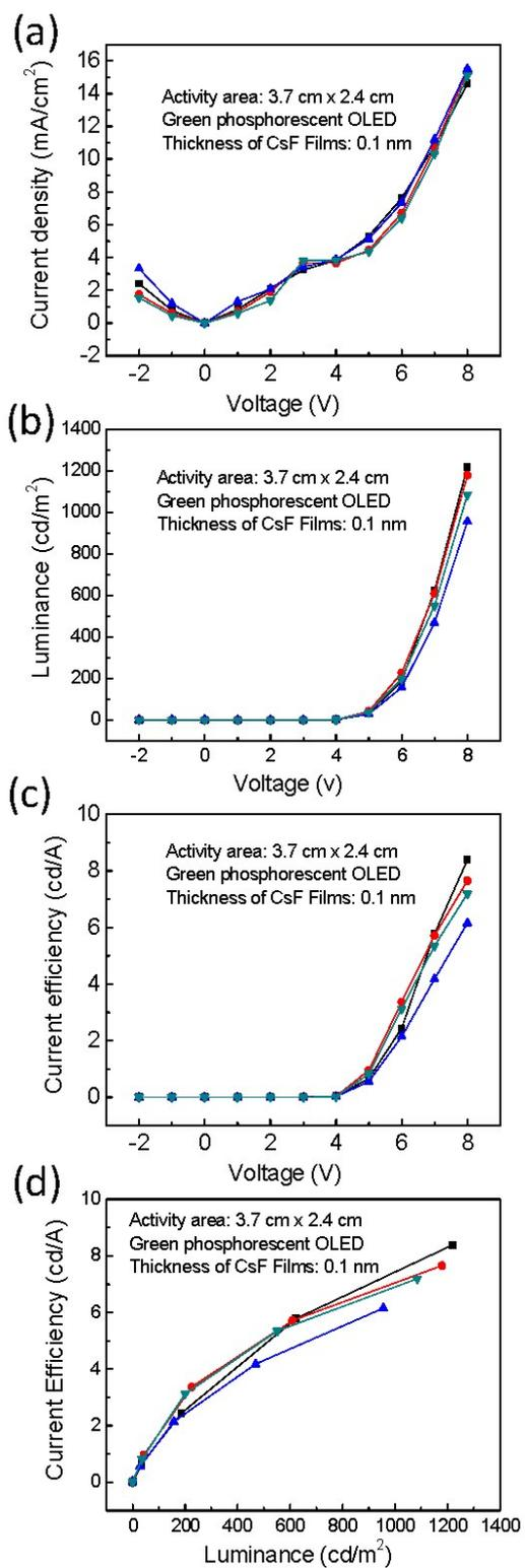
Figure S2 The current density versus voltage, the luminance versus voltage, current efficiency versus voltage, and the current efficiency versus luminance of green OLED devices with 0.1 nm CsF.
