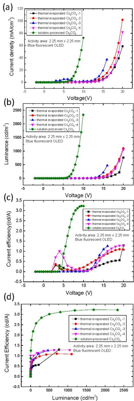
Figure S17 The current density versus voltage, (b) the luminance versus voltage, (c) current efficiency versus voltage, and (d) the current efficiency versus luminance of OLED devices with  $\text{Cs}_2\text{CO}_3$  as the interfacial layer.
