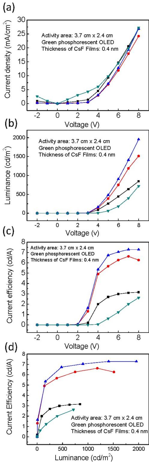
Figure S5 The current density versus voltage, the luminance versus voltage, current efficiency versus voltage, and the current efficiency versus luminance of green OLED devices with 0.4 nm CsF.
