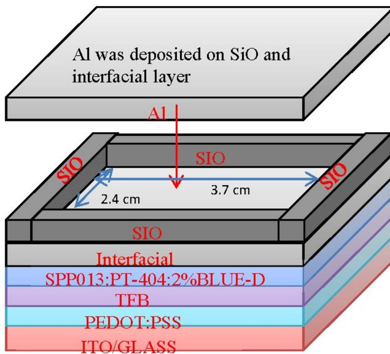
Figure S1 A layer of SiO was added to define the active area (3.7 cm x 2.4 cm) of the large-area OLEDs.
