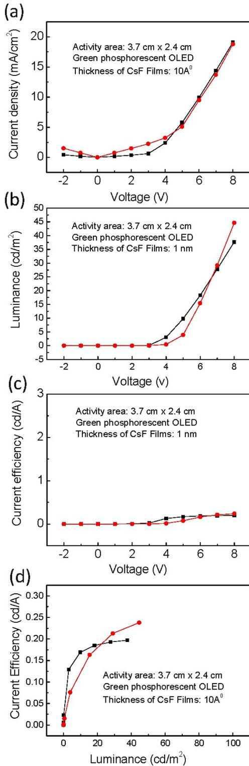
Figure S6 The current density versus voltage, the luminance versus voltage, current efficiency versus voltage, and the current efficiency versus luminance of green OLED devices with 1 nm CsF.
