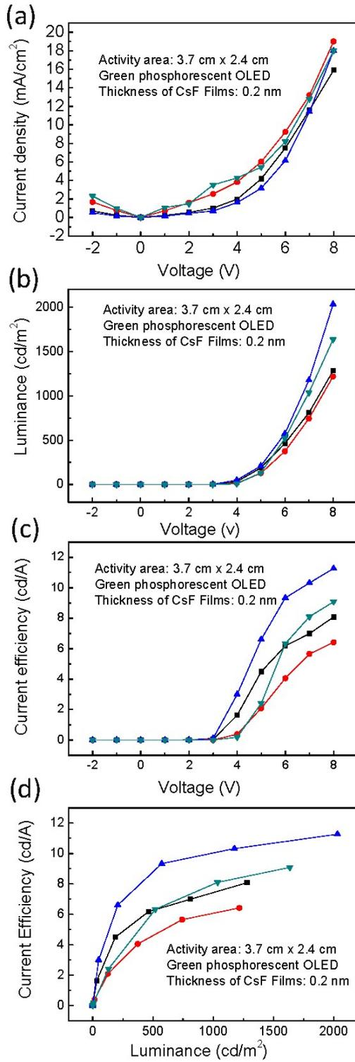
Figure S3 The current density versus voltage, the luminance versus voltage, current efficiency versus voltage, and the current efficiency versus luminance of green OLED devices with 0.2 nm CsF.
