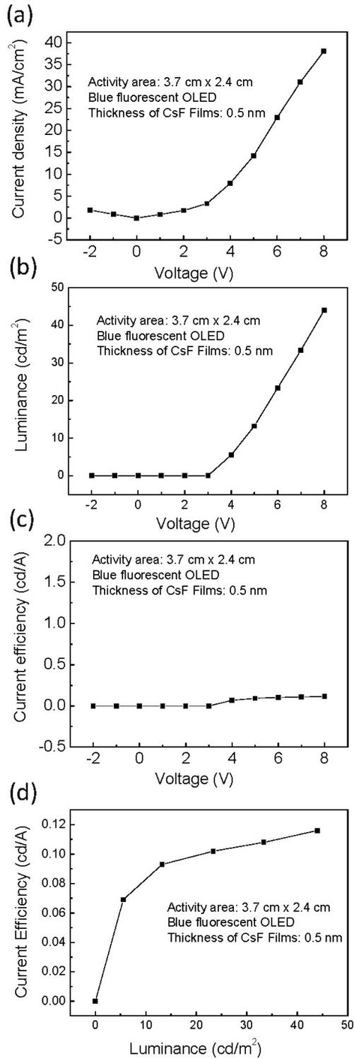
Figure S12 The current density versus voltage, the luminance versus voltage, current efficiency versus voltage, and the current efficiency versus luminance of blue OLED devices with 0.5 nmCsF.
