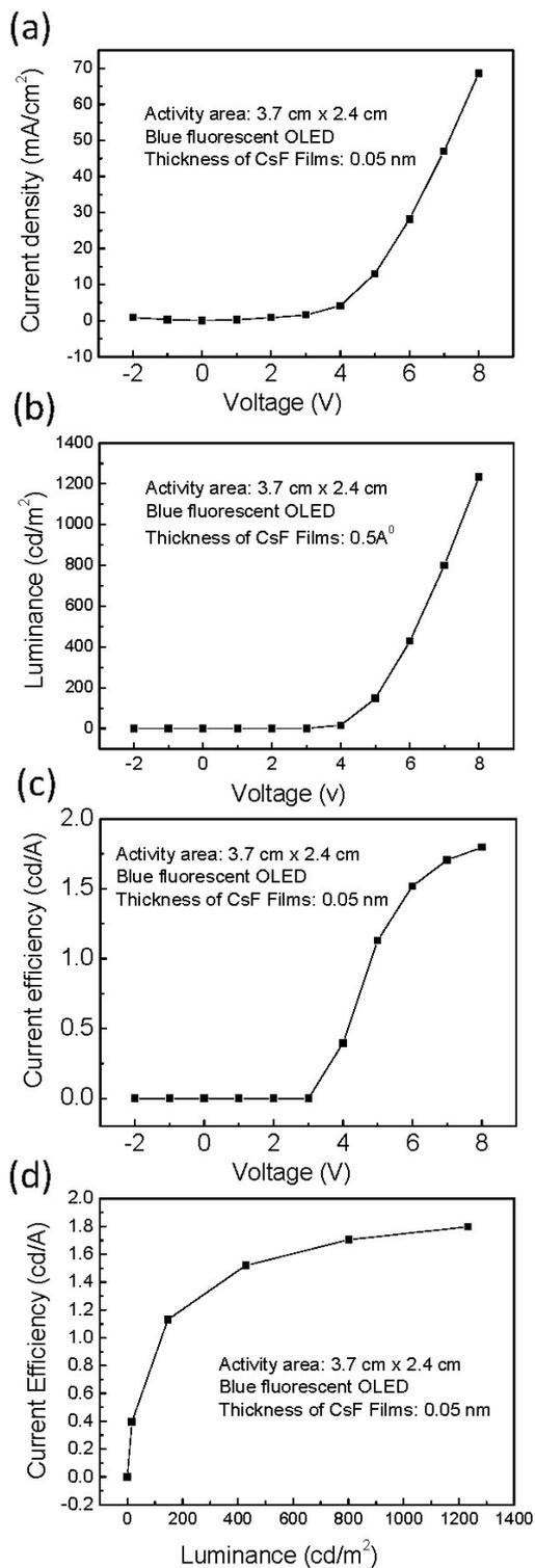
Figure S7 The current density versus voltage, the luminance versus voltage, current efficiency versus voltage, and the current efficiency versus luminance of blue OLED devices with 0.05 nm CsF.
