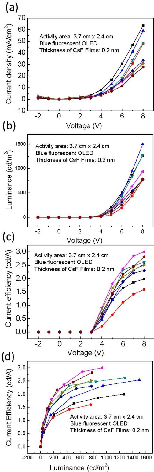
Figure S9 The current density versus voltage, the luminance versus voltage, current efficiency versus voltage, and the current efficiency versus luminance of blue OLED devices with 0.2 nm CsF.
