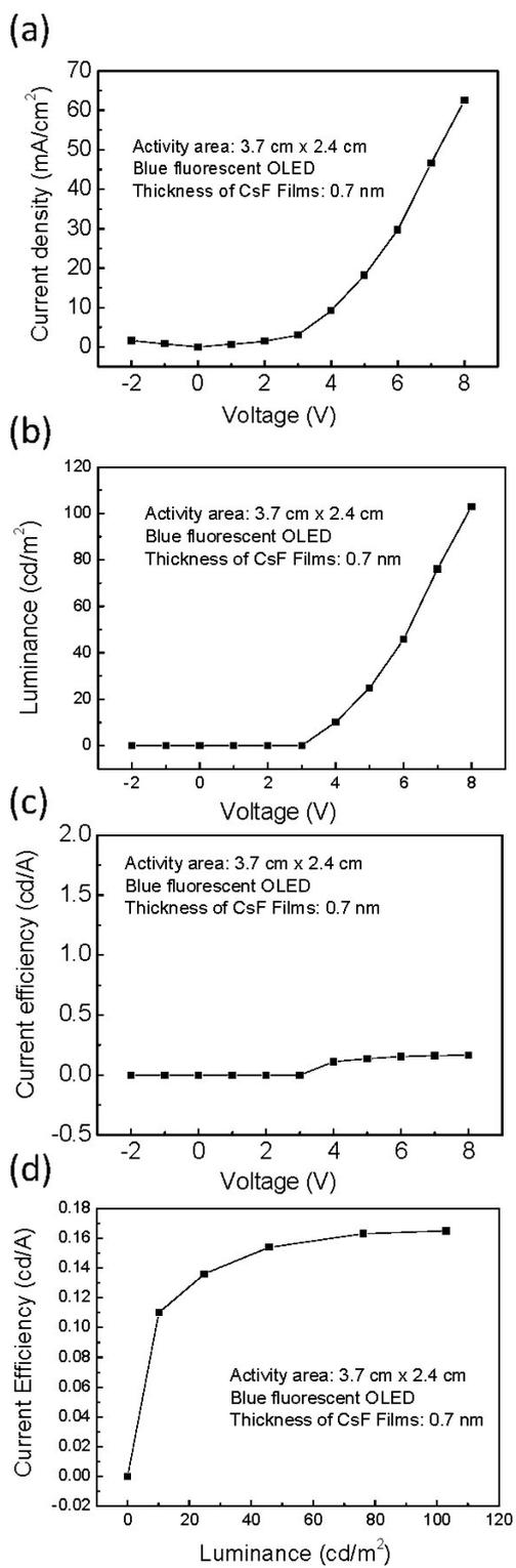
Figure S13 The current density versus voltage, the luminance versus voltage, current efficiency versus voltage, and the current efficiency versus luminance of blue OLED devices with 0.7 nm CsF.
