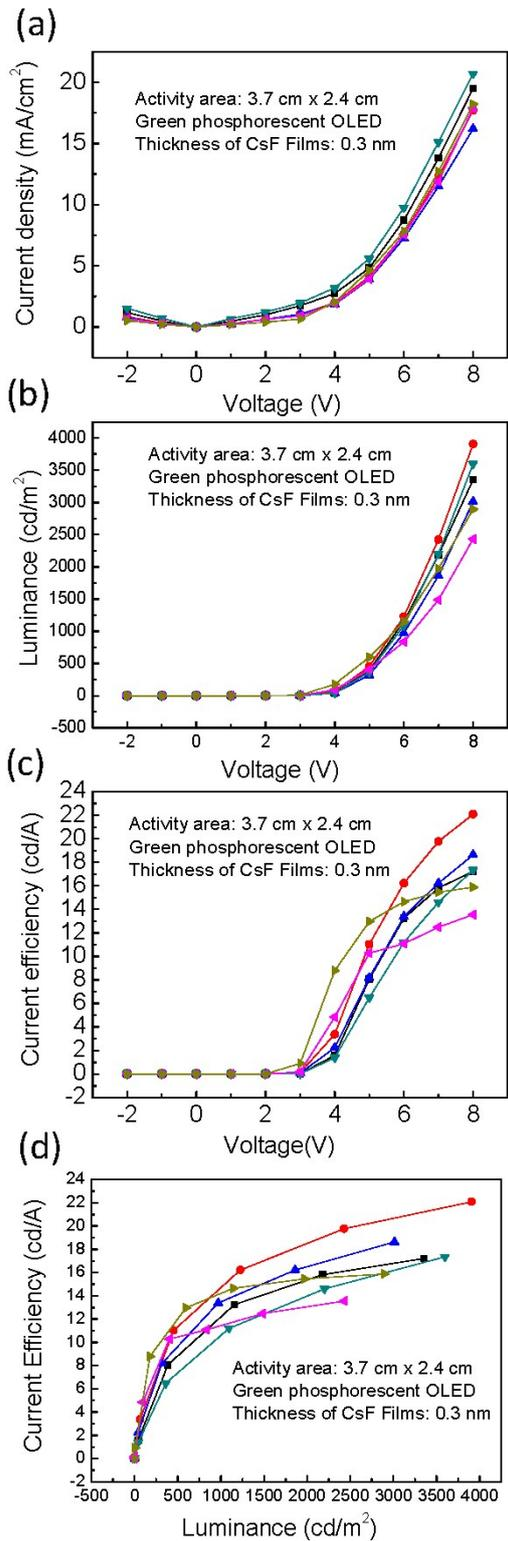
Figure S4 The current density versus voltage, the luminance versus voltage, current efficiency versus voltage, and the current efficiency versus luminance of green OLED devices with 0.3 nm CsF.
