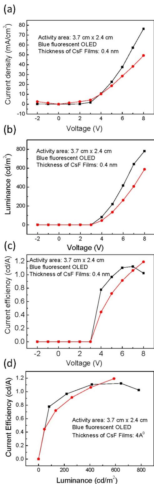
Figure S11 The current density versus voltage, the luminance versus voltage, current efficiency versus voltage, and the current efficiency versus luminance of blue OLED devices with 0.4 nm CsF.
