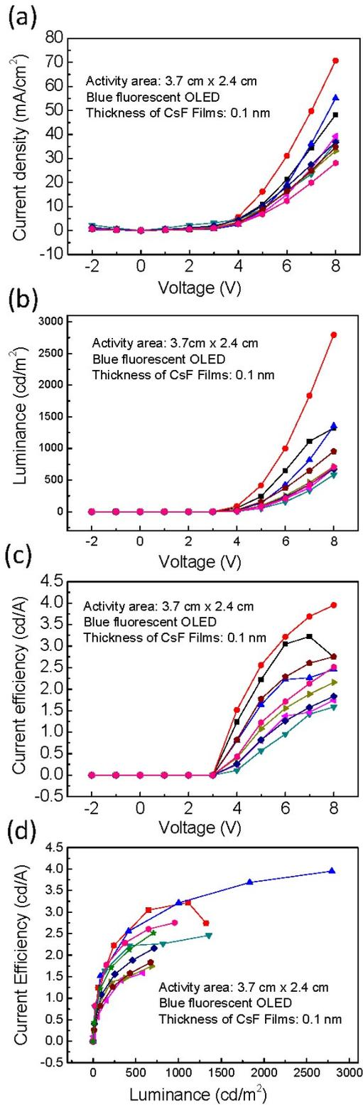
Figure S8 The current density versus voltage, the luminance versus voltage, current efficiency versus voltage, and the current efficiency versus luminance of blue OLED devices with 0.1 nm CsF.
