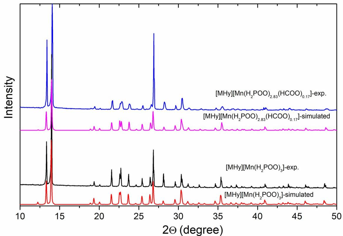
Figure S1. Room-temperature powder XRD pattern for the obtained samples together with the calculate ones based on the RT single crystal structure.
