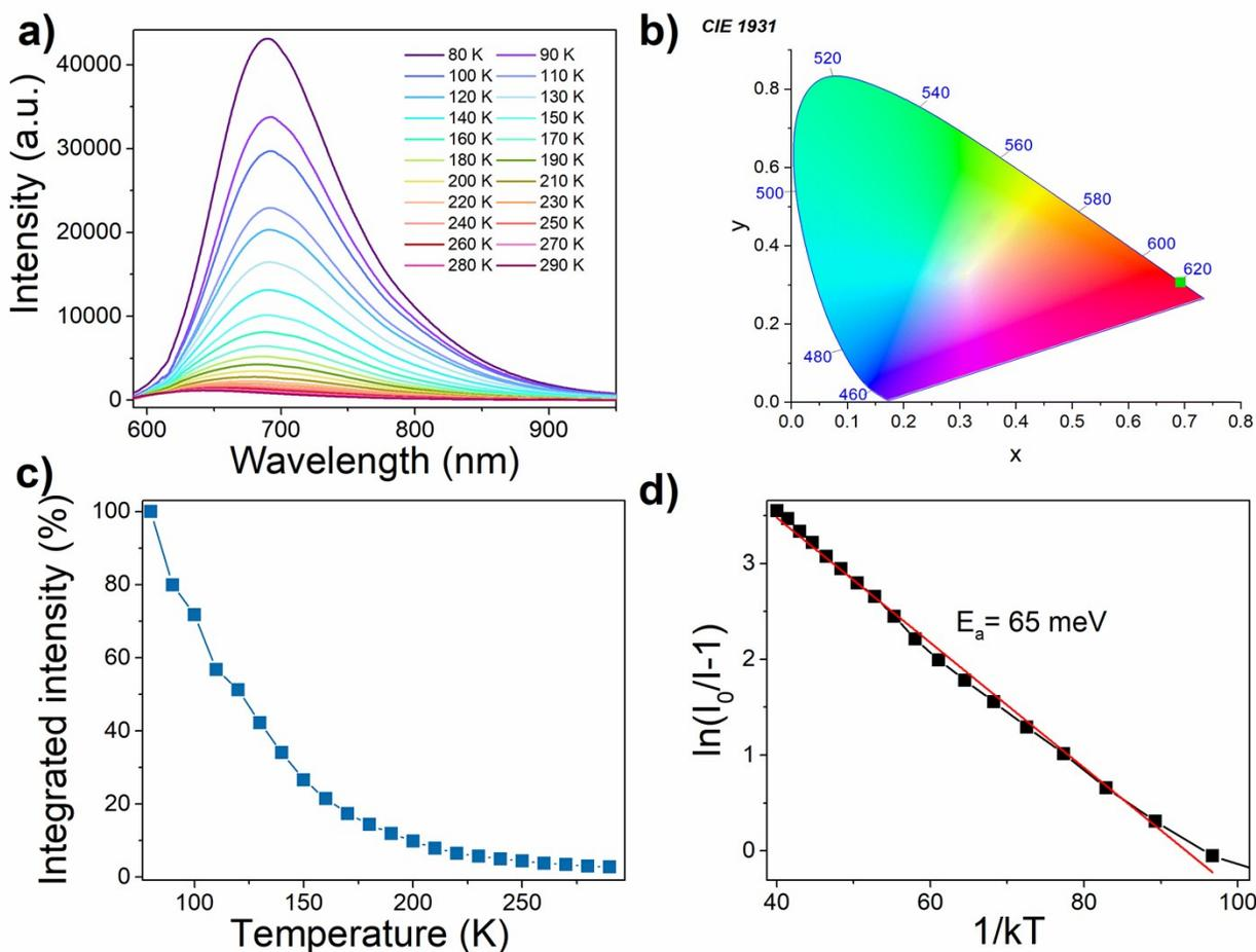
Figure S7. a) The temperature-dependent emission spectra of  $[\text{MHy}][\text{Mn}(\text{H}_2\text{POO})_{2.83}(\text{HCOO})_{0.17}]$  excited at 266 nm, b) CIE coordinate at 80 K, c) integrated emission intensity as a function of temperature and d) activation energy of the thermal quenching.
