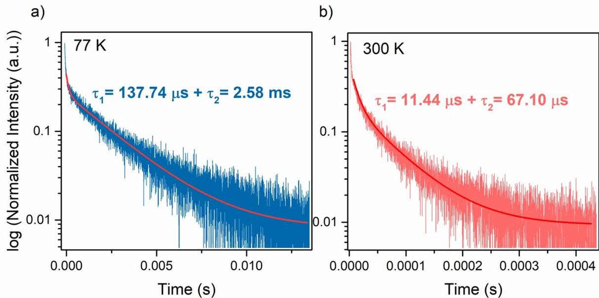
Figure S8. Emission decay curves of  $[\text{MHy}][\text{Mn}(\text{H}_2\text{POO})_{2.83}(\text{HCOO})_{0.17}]$  at a) 77 K and b) 300 K.
