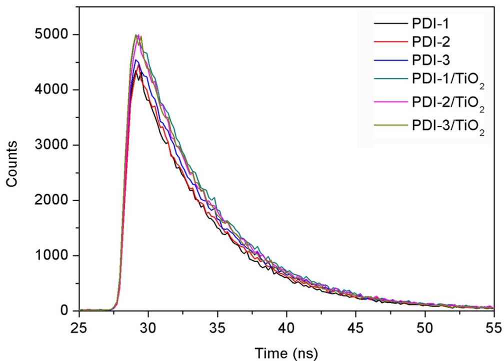
**Figure S13.** Fluorescence decay transients measured at 493 nm PDI-1, PDI-2, PDI-3, PDI-1/TiO<sub>2</sub>, PDI-2/TiO<sub>2</sub>, and PDI-3/TiO<sub>2</sub>.
