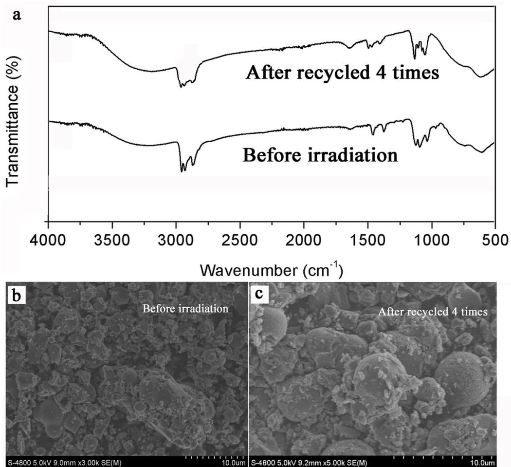
**Figure S15.** FT-IR spectra (a) and SEM images (b, c) of PDI-1/ $\text{TiO}_2$  photocatalyst before and after 4 cyclic runs.
