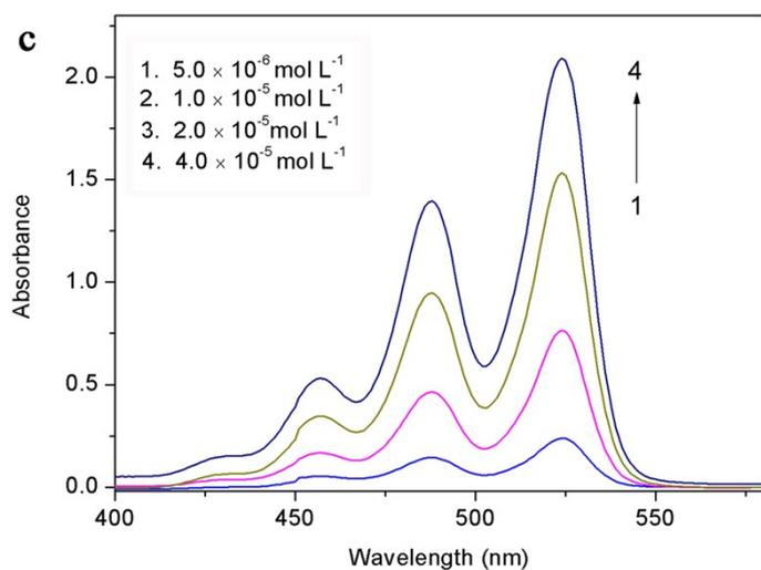
**Figure S10** Absorption spectra of PDI-1 (a), PDI-2 (b) and PDI-3 (c) in dichloromethane at various concentrations.
