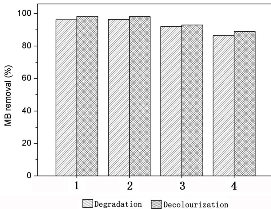
**Figure S14.** Catalyst reusability with PDI-1/TiO<sub>2</sub> catalysts under visible light; [MB] = 10 mg/L,
