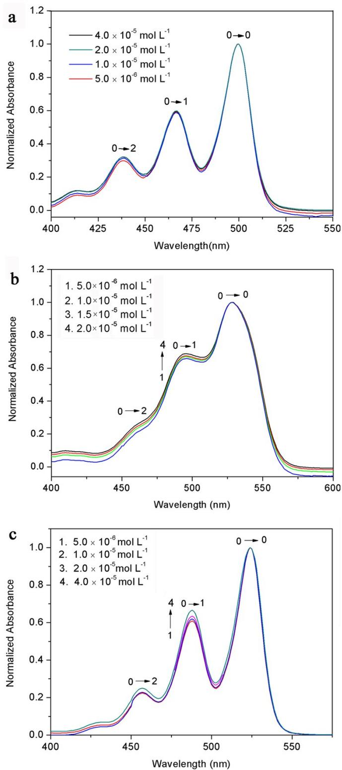
**Figure S11** Normalized absorption spectra of PDI-1 (a), PDI-2 (b) and PDI-3 (c) in dichloromethane at various concentrations.
