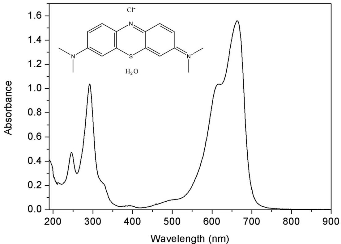
Figure S9. Dye MB structure and UV-visible absorption spectrum.
