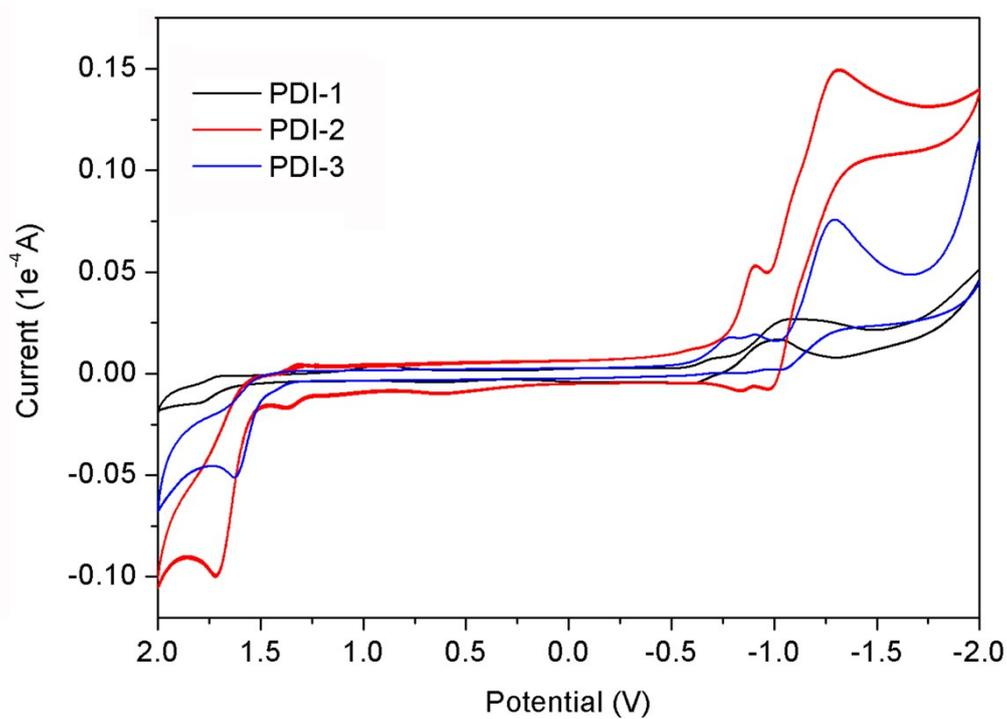
**Figure S12.** Cyclic voltammogram of PDI-1, PDI-2 and PDI-3 in dichloromethane.
