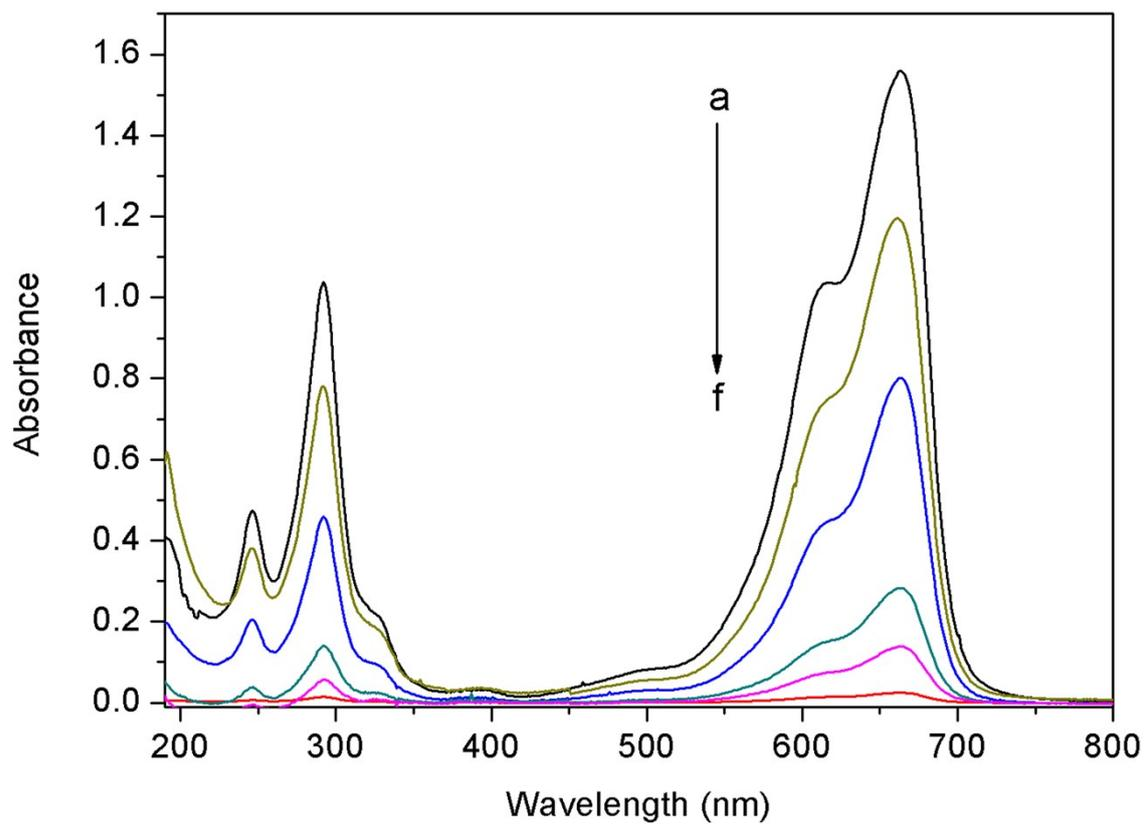
**Figure S16.** The changes in UV-vis spectra of MB on irradiation with visible light in the presence of PDI-1/TiO<sub>2</sub>. a) 0 min, b) 20 min, c) 40 min, d) 60 min, e) 80 min and f) 120 min. [MB] = 10 mg/L, pH = 7, catalyst suspended = 1g/L.
