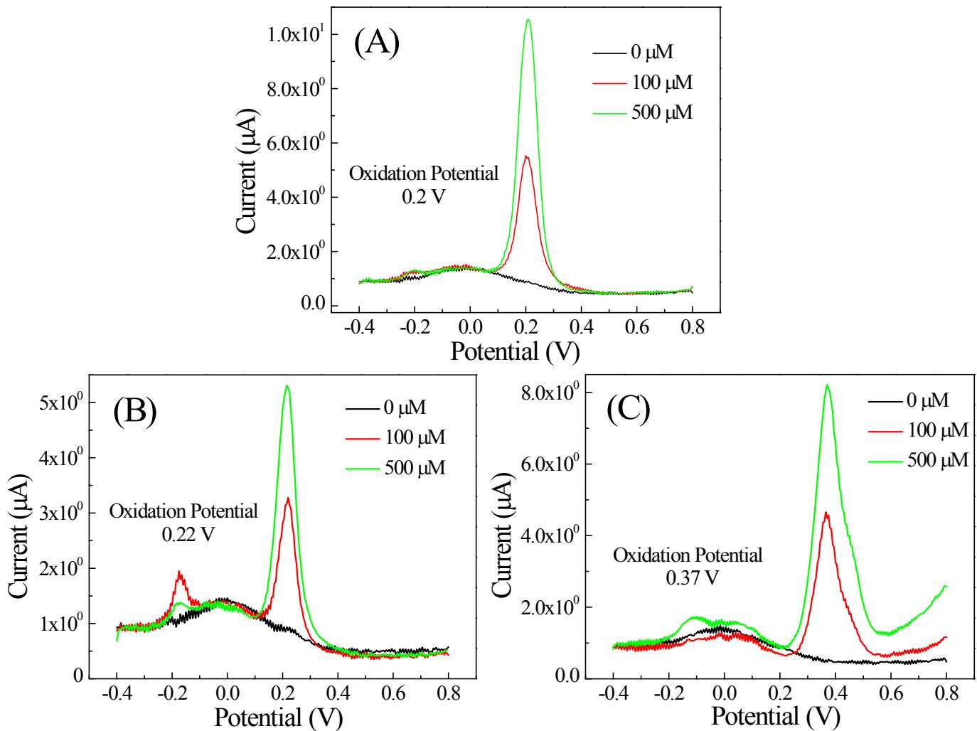
**Fig. S2** Differential pulse voltammograms of (A) dopamine; (B) epinephrine; and (C) serotonin in PBS (50 mM, pH 7.0, 0.9% NaCl).
