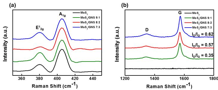
**Fig. S1.** Raman spectra of (a)  $\text{MoS}_2$  and (b) carbon in  $\text{MoS}_2$ -only,  $\text{MoS}_2/\text{GNS}$  9:1,  $\text{MoS}_2/\text{GNS}$  8:2, and  $\text{MoS}_2/\text{GNS}$  7:3.
