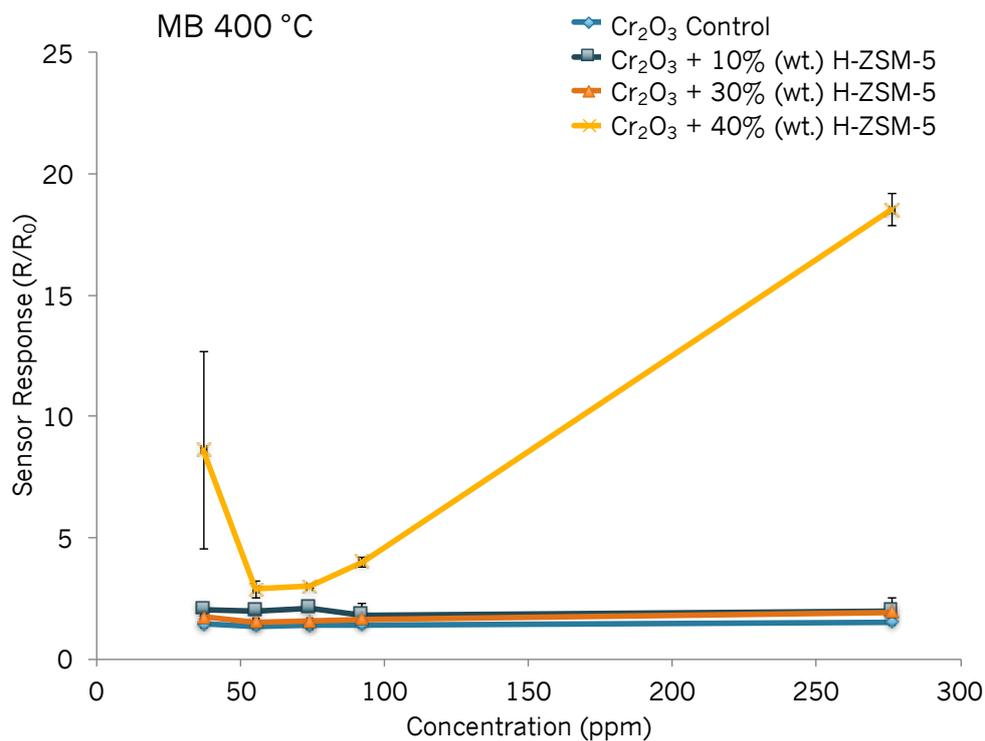
Figure S9. Sensor responses to different concentrations of MB at 400 °C of a Cr<sub>2</sub>O<sub>3</sub> control sensor and those modified by 10% (wt.), 30 % (wt.) and 40% (wt.) of zeolite H-ZSM-5. The results correspond to the average of 3 repeat tests.
