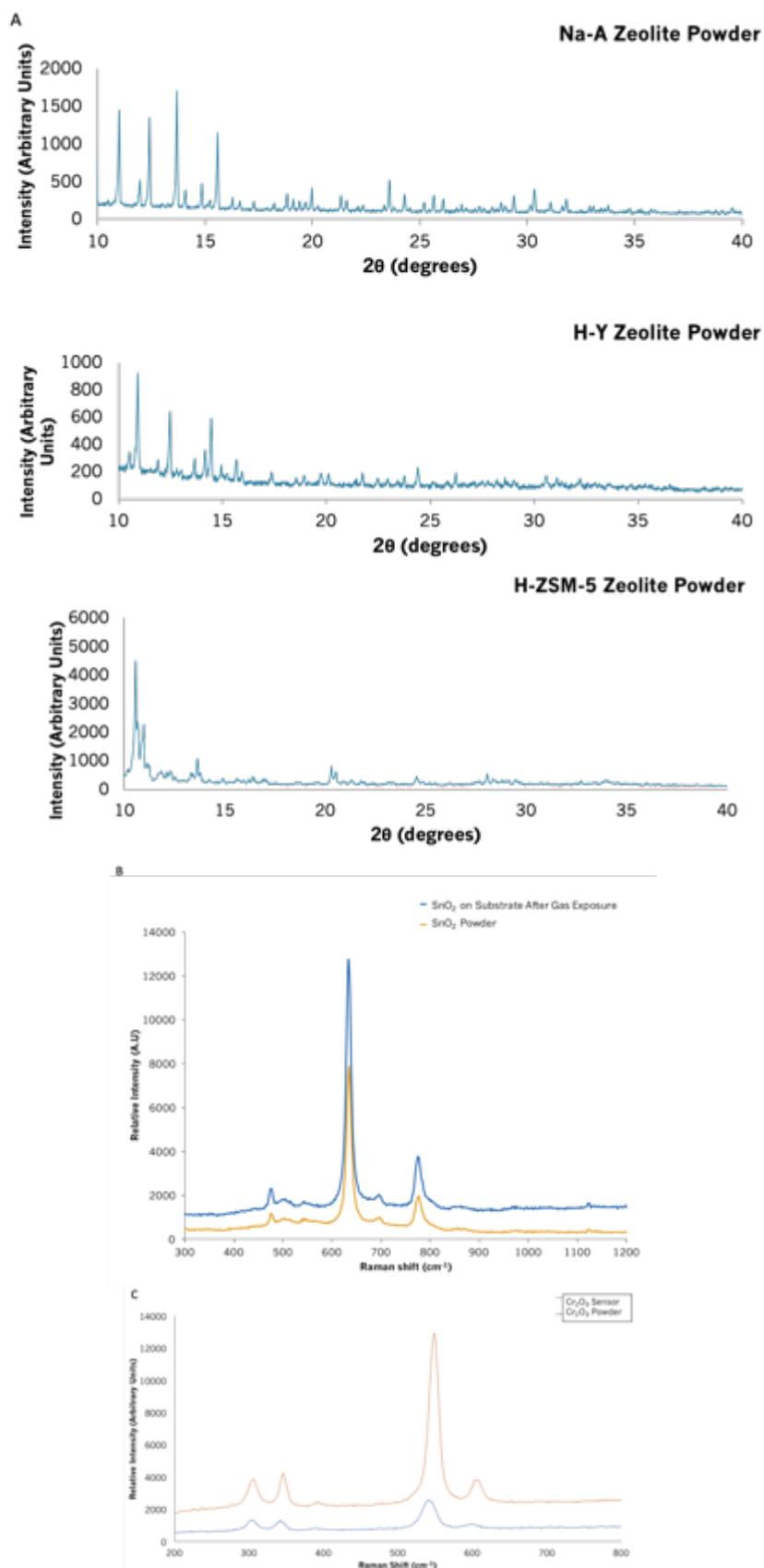
Figure S13 – Physicochemical characterization of sensing materials before and after gas sensing tests. A) XRD patterns of Na-A, H-Y, and H-ZSM-5 zeolite powders. B) Raman spectra of SnO<sub>2</sub> sensing material on substrate and SnO<sub>2</sub> powder. C) Raman spectra of Cr<sub>2</sub>O<sub>3</sub> sensing material on substrate and Cr<sub>2</sub>O<sub>3</sub> powder.
