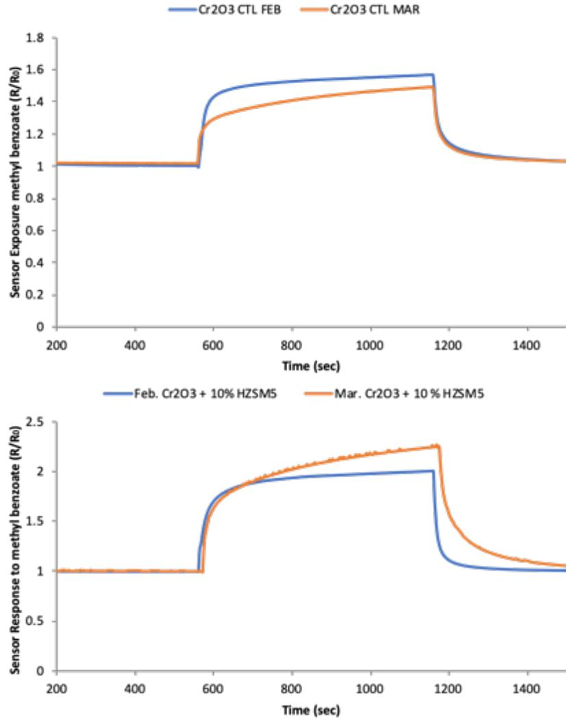
Figure S12 – Cr<sub>2</sub>O<sub>3</sub>-based sensor responses to 275 ppm MB after continuous use for 23 days.
