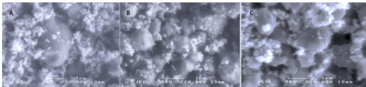
Figure S3. SEM images of A)  $\text{SnO}_2$  admixed with 10% (wt.) H-ZSM-5, B)  $\text{SnO}_2$  admixed with 30% (wt.) H-ZSM-5, and C)  $\text{SnO}_2$  admixed with 50% (wt.) H-ZSM-5.
