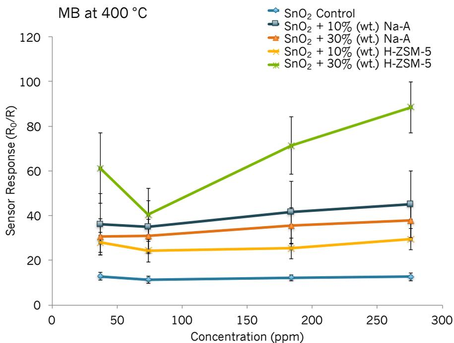
Figure S7. Sensor responses to different concentrations of methyl benzoate at 400 °C of a control SnO<sub>2</sub> sensor, a SnO<sub>2</sub> sensor modified by 10% (wt.) Na-A zeolite, another modified by 30% (wt.) Na-A, another by 10% (wt.) H-ZSM-5 and one modified by 30% (wt.) H-ZSM-5. Error bars corresponding to three repeat tests included.
