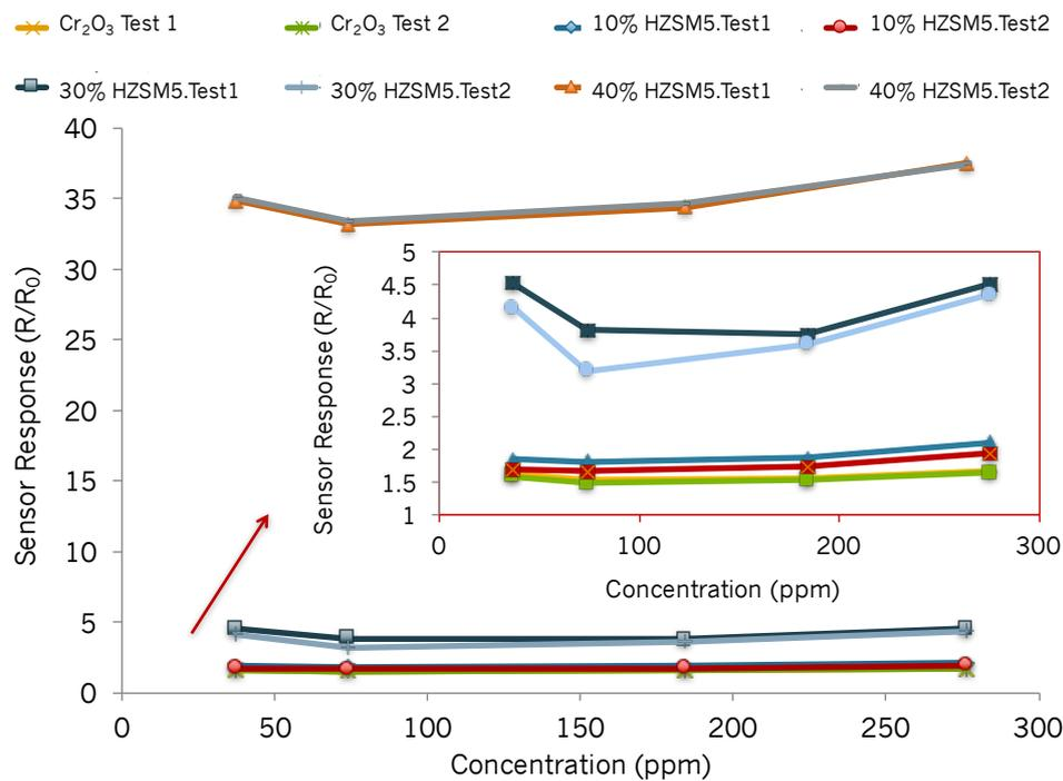
Figure S8. Sensor responses to different concentrations of MB at 350 °C of a Cr<sub>2</sub>O<sub>3</sub> control sensor and those modified by 10% (wt.), 30 % (wt.) and 40% (wt.) zeolite H-ZSM-5. The inset corresponds to the lower sensor responses, which were difficult to see. The graph includes results of two repeat tests for each sensor. The inset has been provided for clarification.
