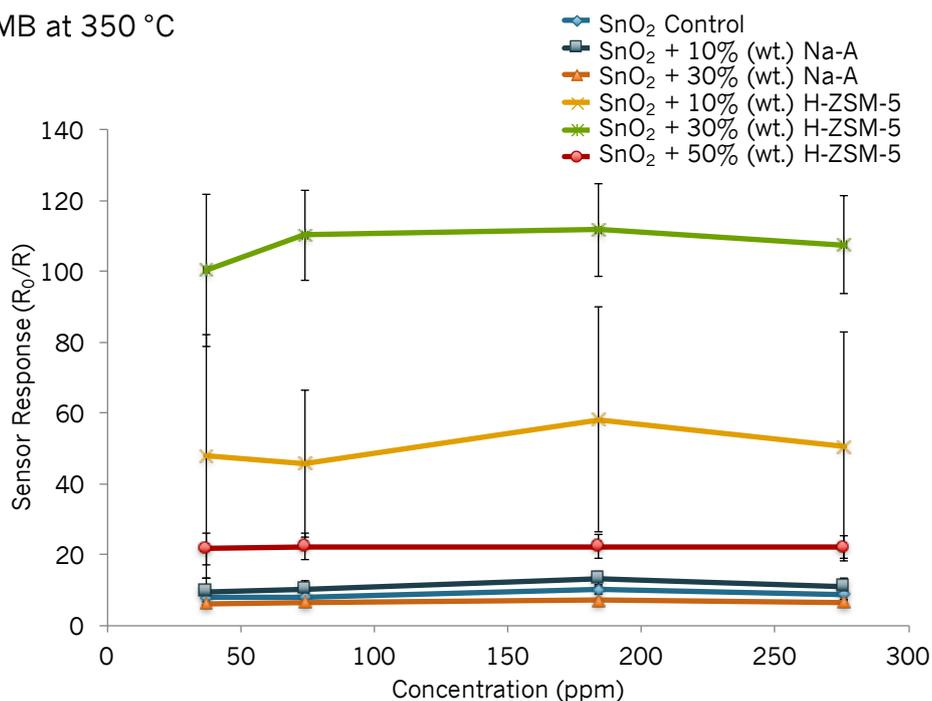
Figure S6. Sensor responses to different concentrations of methyl benzoate at 350 °C of a control SnO<sub>2</sub> sensor, a SnO<sub>2</sub> sensor modified by 10% (wt.) Na-A zeolite, another modified by 30% (wt.) Na-A, another by 10% (wt.) H-ZSM-5 and one modified by 30% (wt.) H-ZSM-5. Error bars corresponding to three repeat tests included.
