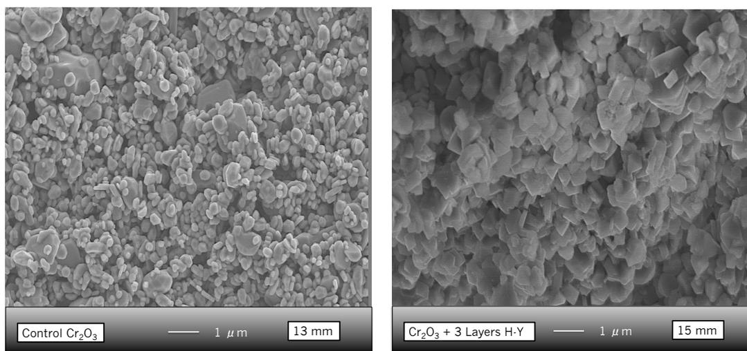
Figure S4. SEM images of a control  $\text{Cr}_2\text{O}_3$  sensor (left) and a  $\text{Cr}_2\text{O}_3$  sensor coated with three layers of zeolite H-Y (right).
