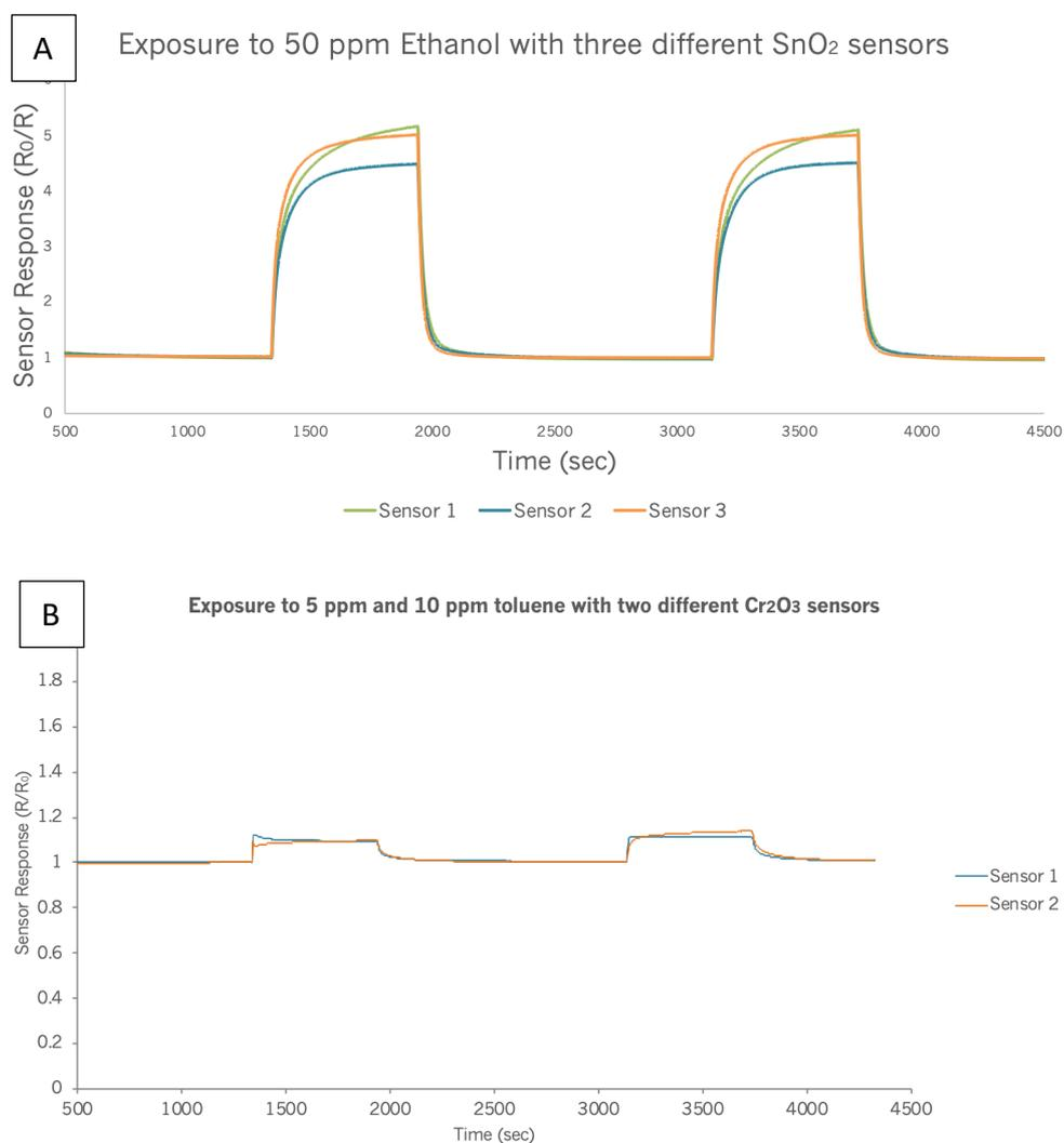
Figure S5. Sensor responses of three different  $\text{SnO}_2$  sensors to two pulses of 50 ppm ethanol at  $400\ ^\circ\text{C}$  (A).  $\text{Cr}_2\text{O}_3$  sensor responses to 5 and 10 ppm toluene, respectively, at  $400\ ^\circ\text{C}$  (B). This test was performed to understand repeatability from one device to another.
