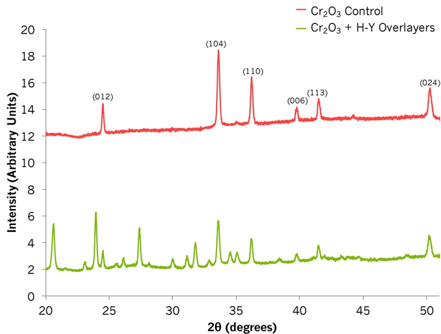
Figure S2. XRD patterns of a control  $\text{Cr}_2\text{O}_3$  sensor and a  $\text{Cr}_2\text{O}_3$  sensor modified by screen-printed layers of zeolite H-Y on top of it. Peaks have been indexed according to the literature.<sup>(1)</sup>
