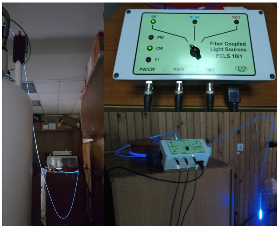
Fig. S IV 1. LED source and optical fiber to the NMR test tube used for “in situ” UV-irradiation NMR spectroscopy.
