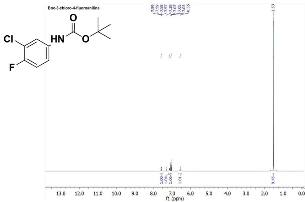
**Figure S7:**  $^1\text{H}$  NMR spectrum of *tert*-butyl *N*-(3-chloro-4-fluorophenyl)carbamate (Entry 4a) in  $\text{CDCl}_3$
