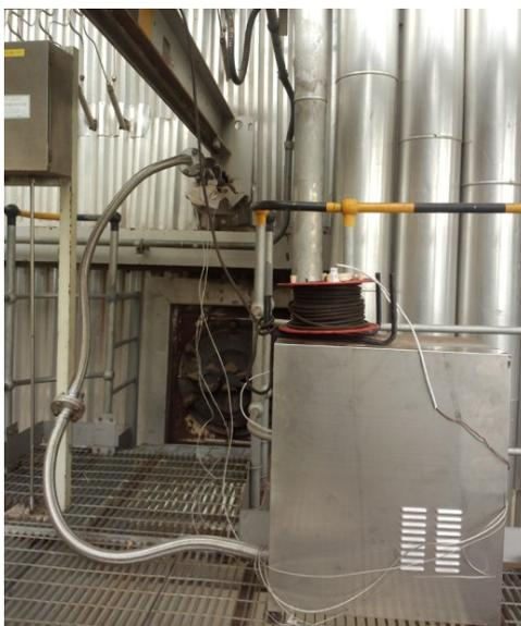
Fig. 1 the temperature-controlled ash deposition probe
