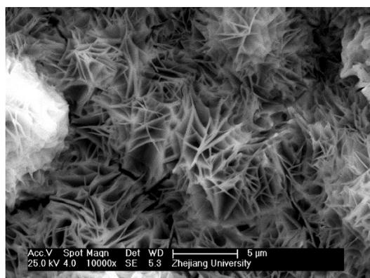
Fig. 3 corrosion on the surface of the sampling ring
