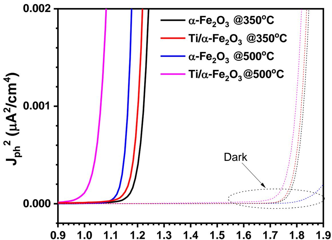
**Figure S3:** Butler plots under dark and 1 Sun illumination for  $\alpha\text{-Fe}_2\text{O}_3$  thin films annealed at 350°C and 500°C and Ti doped  $\alpha\text{-Fe}_2\text{O}_3$  annealed at 350 and 500°C under dark and 1 Sun illumination, in which the turn-on potential is defined as the value at which the extrapolation of the linear relationship between  $(\text{current density})^2$  and applied potential intercepts with  $(\text{current density})^2 = 0$ .
