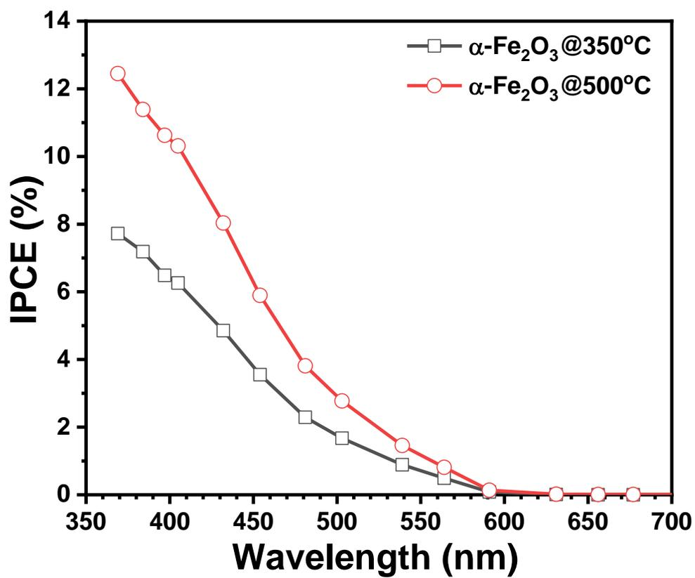
**Figure S4:** IPCE curves for  $\alpha\text{-Fe}_2\text{O}_3$  thin films annealed at 350°C (black) and 500°C (red) measured at 1.23V vs.  $V_{\text{RHE}}$ .
