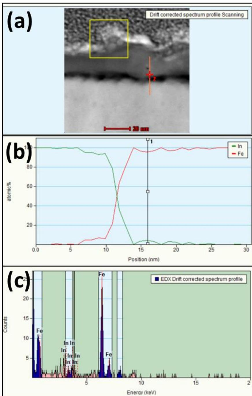
**Figure S1:** (a) STEM images for EDX line scan (b) respective EDX line scan clearly shows the distribution of Fe and In element in cross-section of  $\alpha$ -Fe<sub>2</sub>O<sub>3</sub> annealed at 500°C (c) EDX spectra reveal that Fe and In are the main elements present within the selected line scan.
