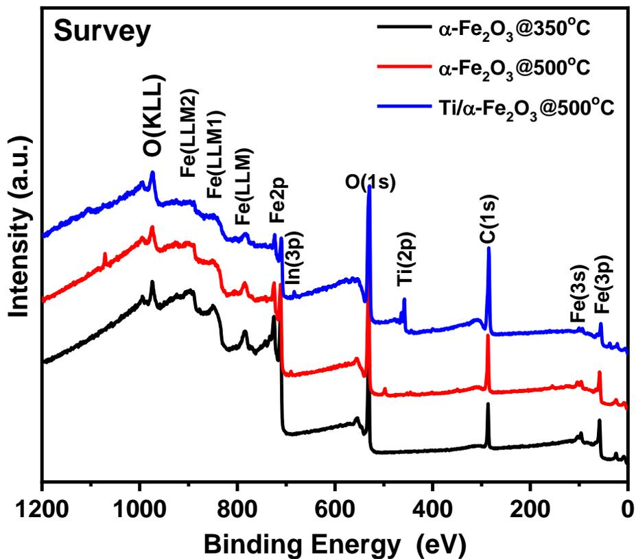
**Figure S2:** XPS survey scan recorded on  $\alpha\text{-Fe}_2\text{O}_3$  thin films annealed at  $350^\circ\text{C}$  and  $500^\circ\text{C}$  and Ti doped  $\alpha\text{-Fe}_2\text{O}_3$  annealed  $500^\circ\text{C}$
