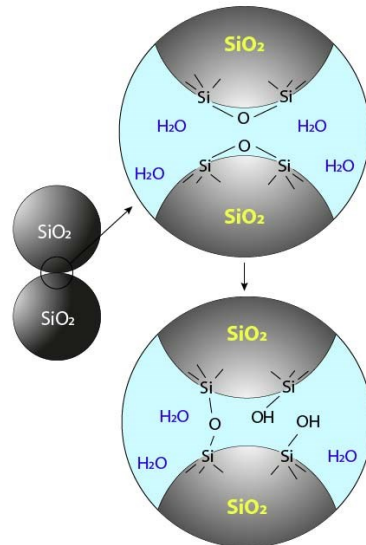
Fig. S4. Proposed sintering mechanism of two SiO 2 nanoparticles
