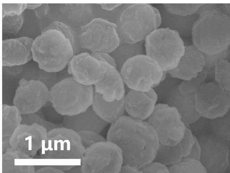
**Figure S4.** SEM image of sulfur spheres.
