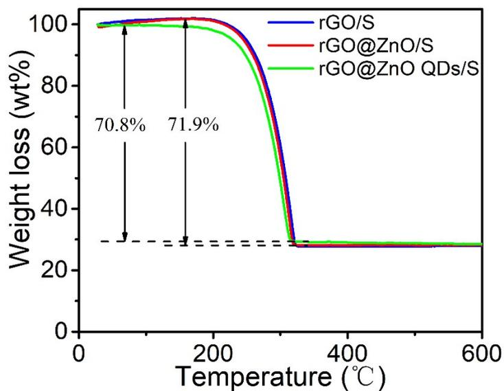
**Figure S7.** TGA curves of composites rGO/S, rGO@ZnO/S, and rGO@ZnO
