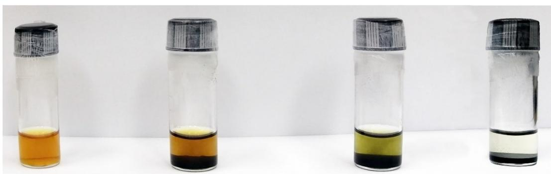
**Figure S9.** Visualized polysulfides adsorption experiments. The samples from left to right are pure  $Li_2S_6$ , rGO, rGO@ZnO, and rGO@ZnO QDs in  $Li_2S_6$ , which were kept still at room temperature for 6 hours before taking photographs.
