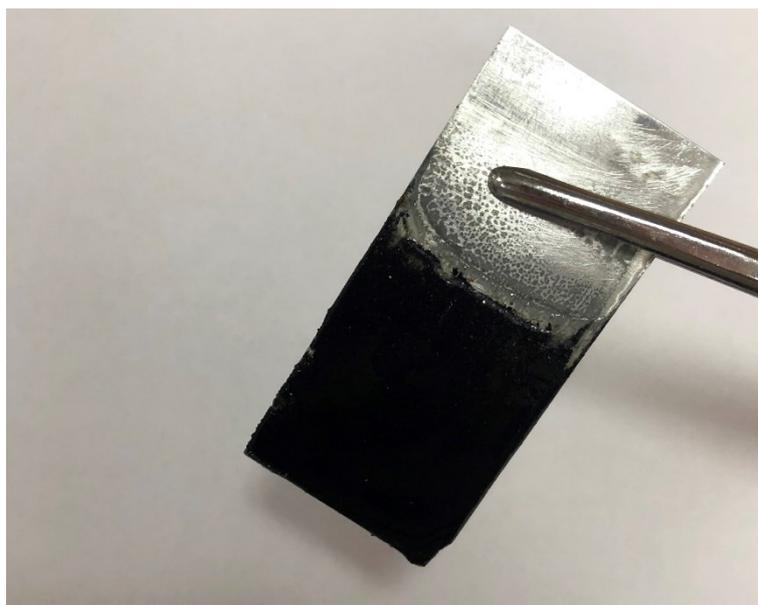
**Figure S1.** Photograph of Zn foil after being immersed in GO solution for 4 hours, with a layer of GO@ZnO attaching on its surface.
