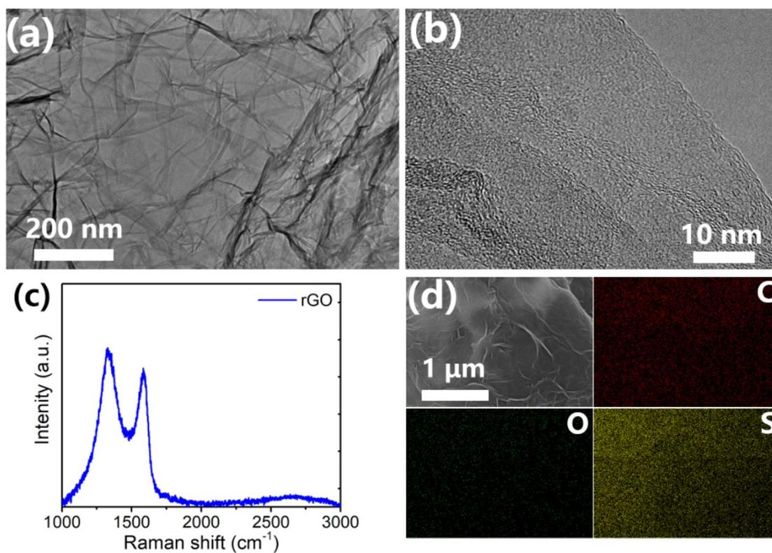
**Figure S6.** (a) TEM and (b) HRTEM image of rGO; (c) Raman spectrum of rGO; (d) EDS elemental mappings of rGO/S.
