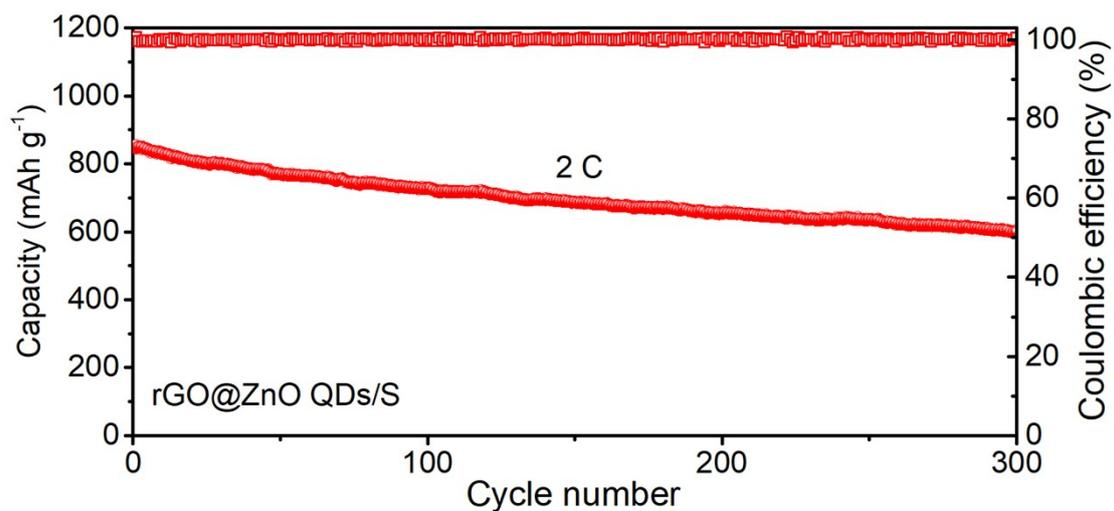
**Figure S10.** Cycling performance of rGO@ZnO QDs/S at a high rate of 2 C.
