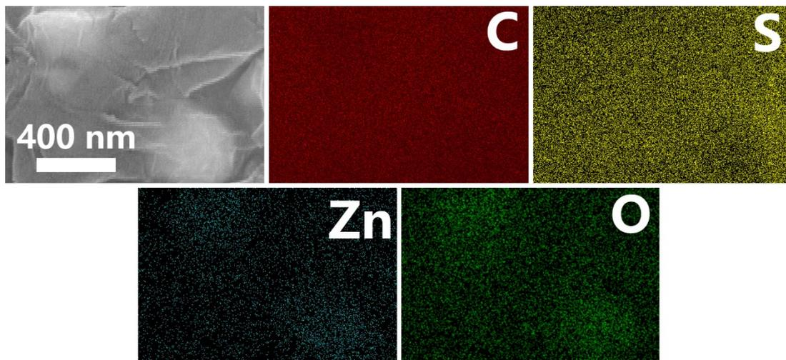
**Figure S5.** EDS elemental mappings of rGO@ZnO/S composite.
