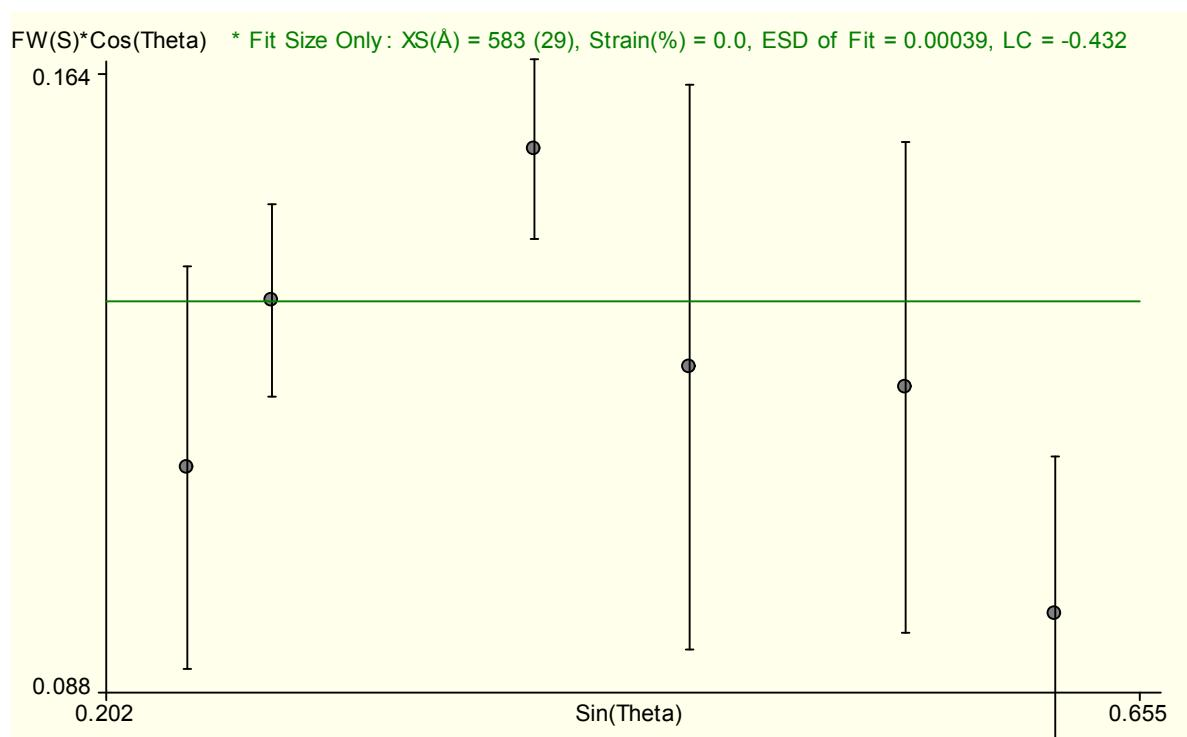
Figure S1: Williamson hull plot to estimate size of Ag-NiMn<sub>2</sub>O<sub>4</sub> nanocomposite.
