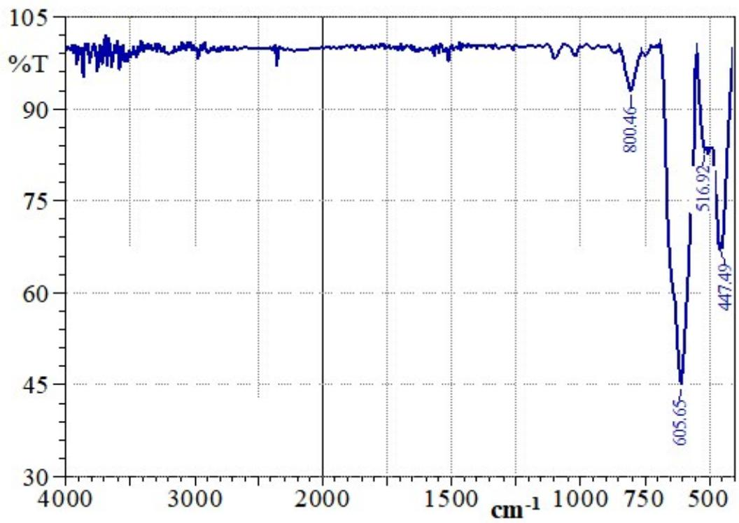
**Figure S3:** FTIR spectra of  $\text{Ag}\cdot\text{NiMn}_2\text{O}_4$  nanocomposite calcined at  $950\text{ }^\circ\text{C}$
