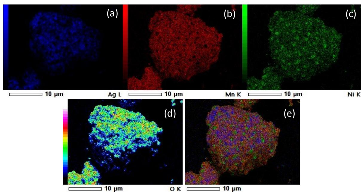
Figure S2: SEM-EDS mapping of (a) Silver, (b) Manganese, (c) Nickel, (d) Oxygen, and (e) is their Overlap
