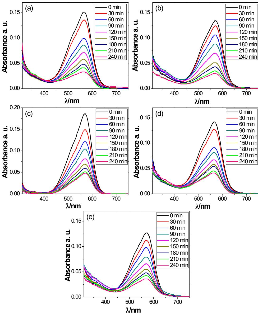
Figure S9: (a-e) Recycle and reuse of photocatalyst for MV degradation (MV concentration:  $5\text{mgL}^{-1}$ ), Photocatalyst dosage:  $0.4\text{ gL}^{-1}$ , in the presence of catalyst  $\text{Ag}\cdot\text{NiMn}_2\text{O}_4$  at pH-9 (irradiation time 4h).
