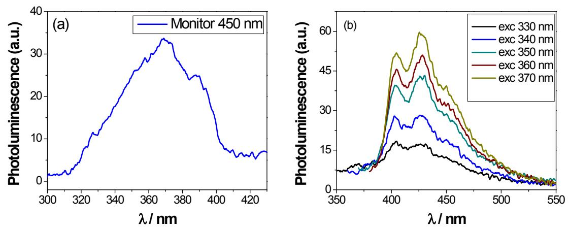
**Figure S7:** PLE (a) and PL (b) spectra of single metal oxide ( $\text{MnO}$ ) nanocomposites heated at  $950\text{ }^{\circ}\text{C}$
