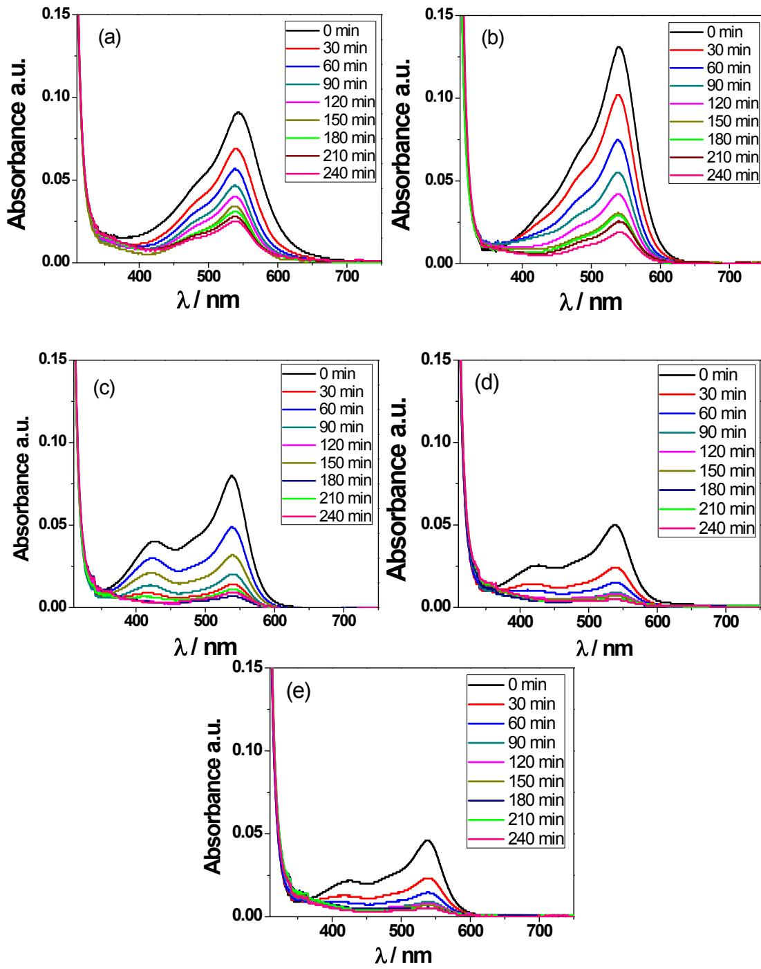
Figure S8: Effect of catalyst amount of  $\text{Ag}\cdot\text{NiMn}_2\text{O}_4$  on degradation efficiency of MV under visible light (a)  $0.3 \text{ g L}^{-1}$ , (b)  $0.4 \text{ g L}^{-1}$ , (c)  $0.5 \text{ g L}^{-1}$ , (d)  $0.6 \text{ g L}^{-1}$ , (e)  $0.7 \text{ g L}^{-1}$ , and (f) % of efficiency comparison (MV concentration:  $5 \text{ mg L}^{-1}$ ; pH-4; irradiation time 4h)
