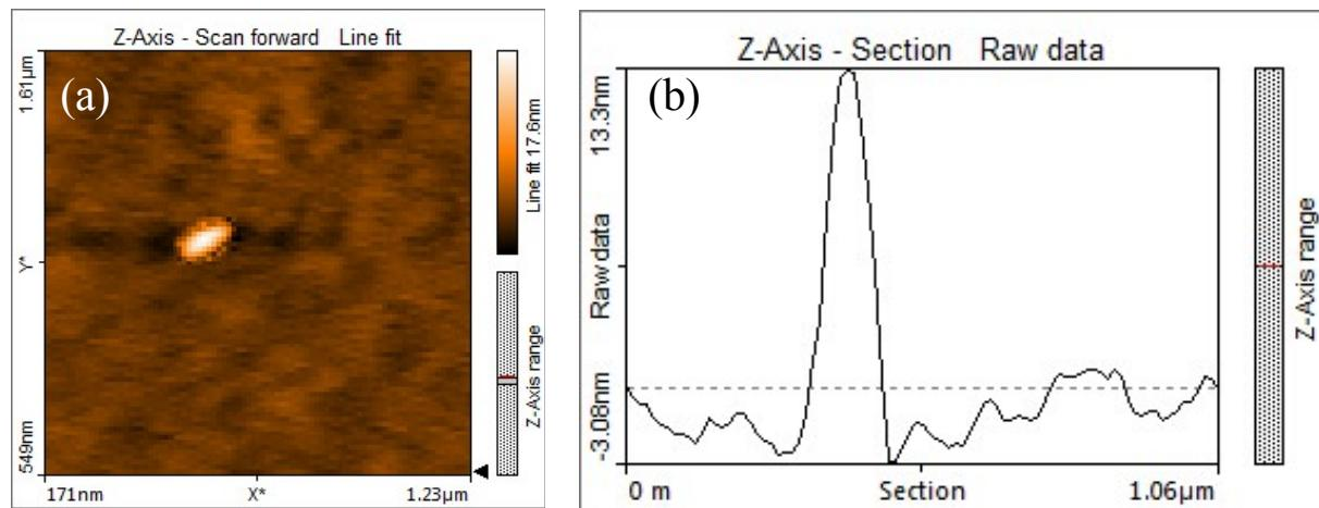
**Figure S4:** Atomic Force Microscopy: (a) image of  $\text{Ag}\cdot\text{NiMn}_2\text{O}_4$  nanocomposite and (b) linear surface roughness analysis
