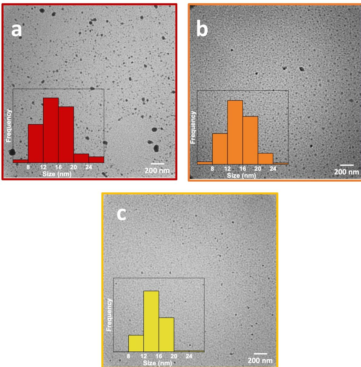
**Figure S4.** TEM images of L-cysCDs at different precursor ratios. TEM images of cysCDs synthesized at 160 °C and 5 mins with 1 L-CYS : 1 CA ratio(a), 1 L-CYS : 2 CA ratio (b), and 2 L-CYS : 1 CA ratio (c). The cysCDs seem to be stagnant in size as a function of reaction precursor.
