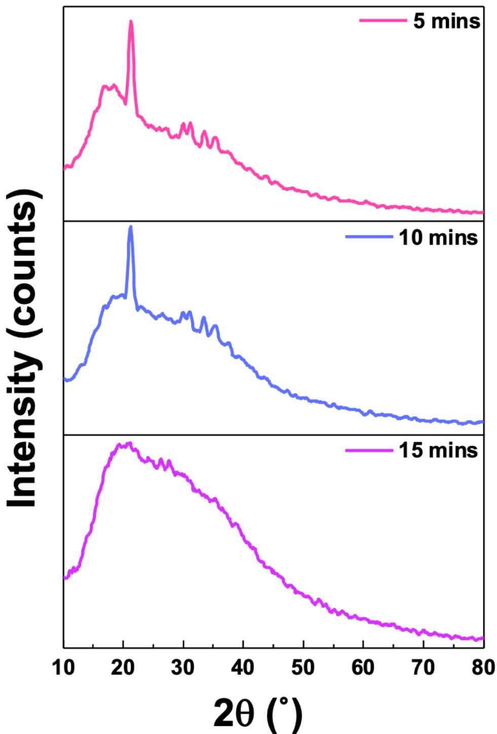
**Figure S13.** XRD spectra of L-cysCDs prepared at different synthesis times at an optimized reaction temperature of  $160^\circ\text{C}$ . The appearance of amorphous halo at  $17^\circ 2\theta$  is indicative of the (002) plane of graphene and the sharp reflections at  $21^\circ$ ,  $30^\circ$ ,  $31^\circ$ ,  $33^\circ$  and  $35^\circ 2\theta$  indicate semi crystalline states present on the CDs. As reaction time is increased at  $160^\circ\text{C}$ , the CDs become increasingly amorphous.
