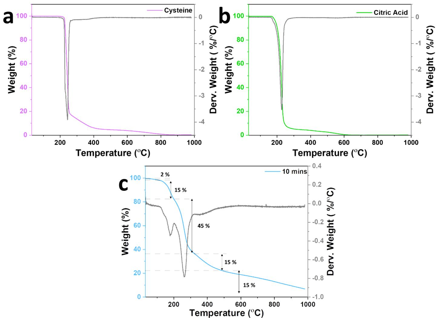
**Figure S7.** TGA spectra precursors cysteine (a) and citric acid (b) with cysCDs (c). The precursors cysteine (a) and citric acid (b) have a sharp and single weightloss occurring at 200°C; however, the cysCDs (c) has several weight loss steps indicating surface functionalities and an amorphous carbon core decomposition at higher temperature.
