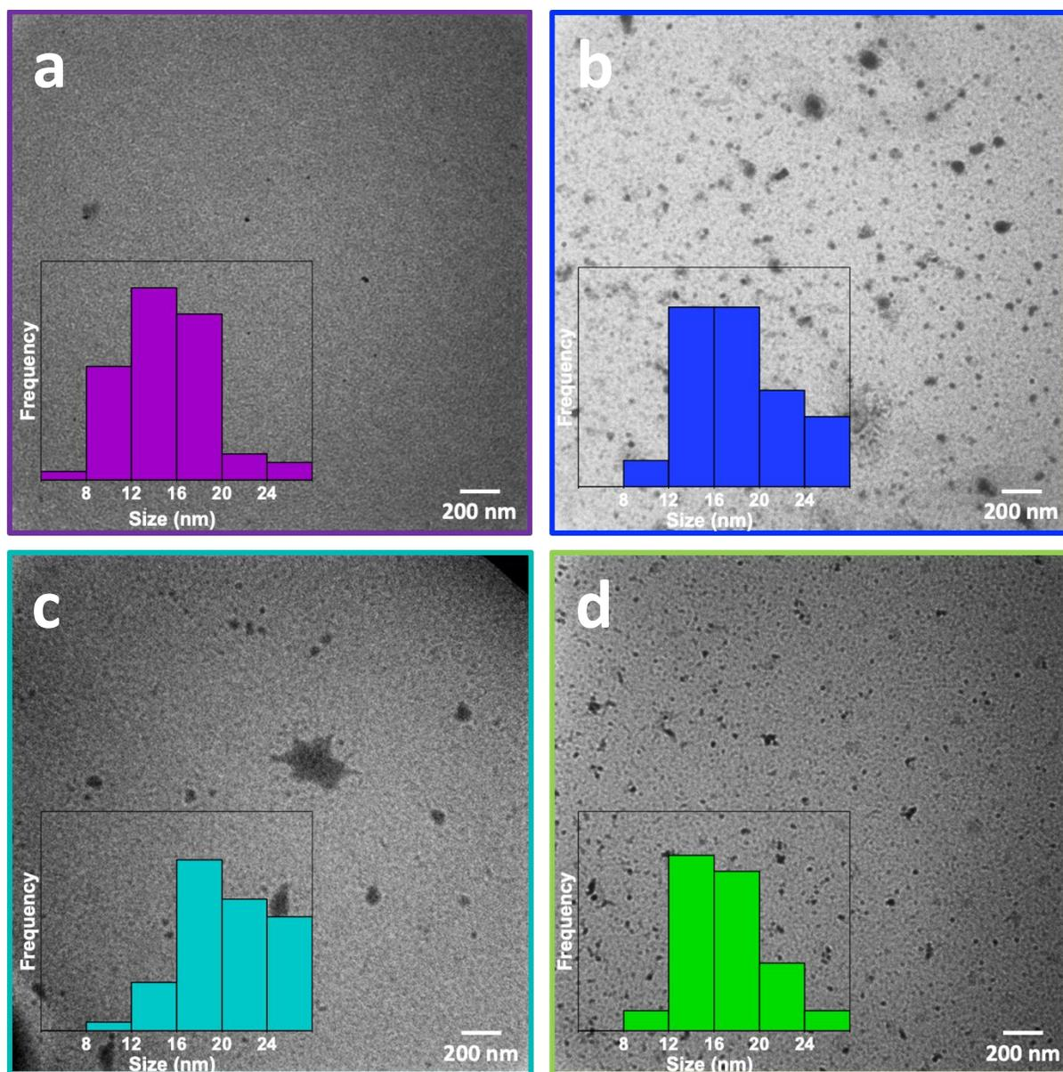
**Figure S2.** TEM images of cysCDs at different reaction temperatures. TEM images of cysCDs synthesized at 5mins different reaction temperature at 160 °C (a), 180 °C (b), 200 °C (c), and 220 °C (d). The cysCDs seem to slightly increase in size as a function of synthesis temperature.
