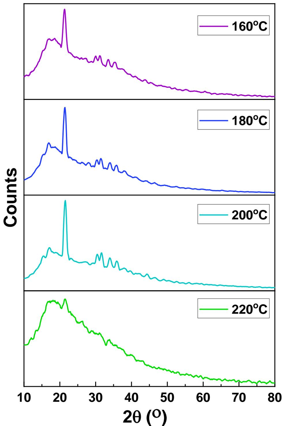
**Figure S9.** XRD spectra of L- cysCDs at different synthesis temperatures. The appearance of amorphous halo at  $17^\circ 2\theta$  is indicative of the (002) plane of graphene and the sharp reflections at  $21^\circ$ ,  $30^\circ$ ,  $31^\circ$ ,  $33^\circ$  and  $35^\circ 2\theta$  indicate a semi-crystalline state present in the cysCDS. However, as synthesis temperature is increased the cysCDs become more disordered.
