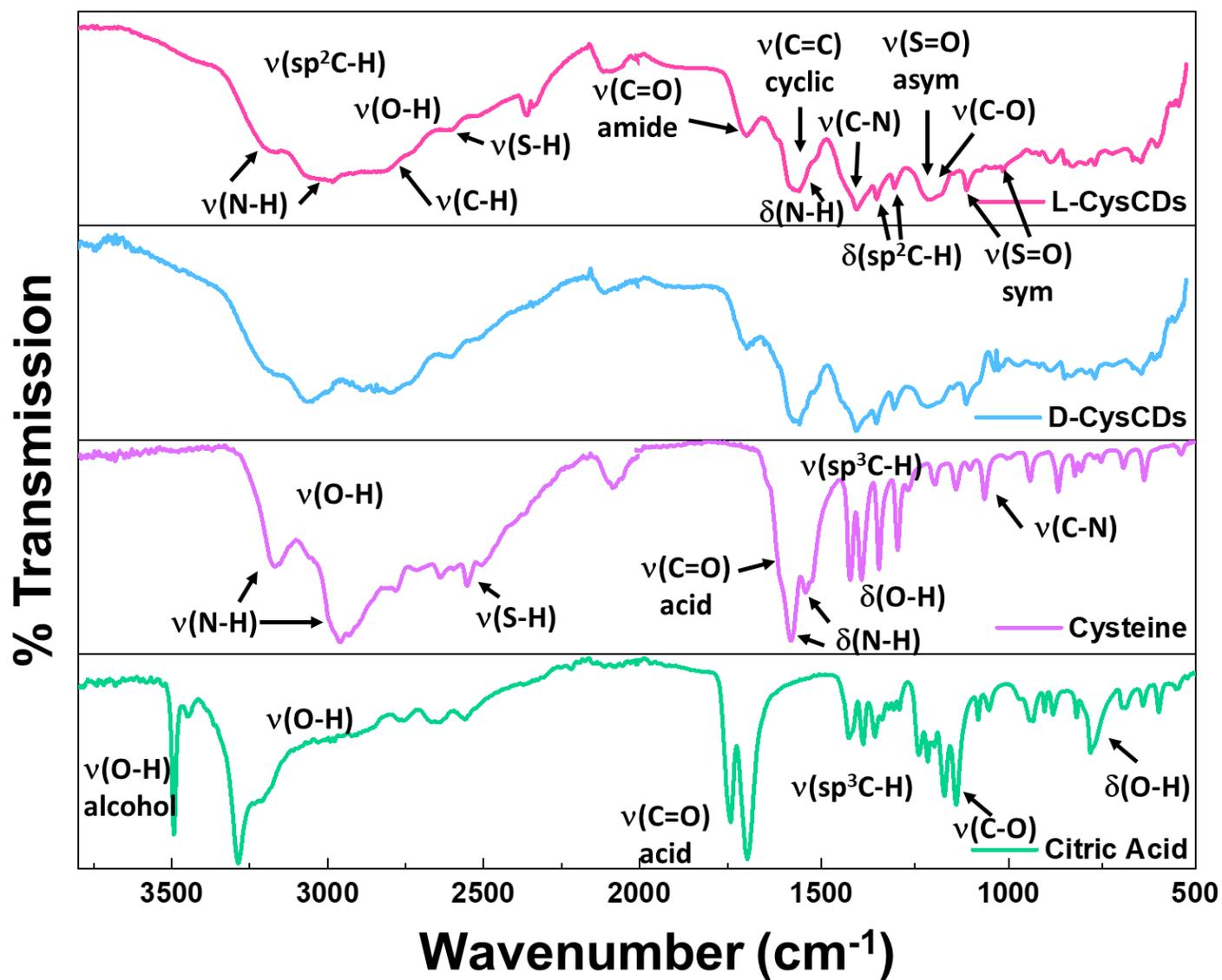
**Figure S8.** FTIR spectra of L- and D-cysCDs with precursors cysteine and citric acid. It is evident that the precursors have decomposed and formed a new system, namely the cysCDs. There is a transformation in the functional groups observed in the precursors and the nanoparticles as such as the presence of amide C=O, and S=O, and the changes observed in the fingerprint region of the spectra (highlighted in the L-cysCDs FTIR spectra).
