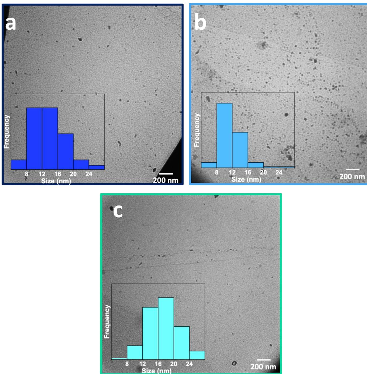
**Figure S5.** TEM images of D-cysCDs at different precursor ratios. TEM images of cysCDs synthesized at 160 °C and 5 mins with 1 D-CYS : 1 CA ratio(a), 1 D-CYS : 2 CA ratio (b),and 2 D-CYS : 1 CA ratio (c).The cysCDs seem to be stagnant in size as a function of reaction precursor.
