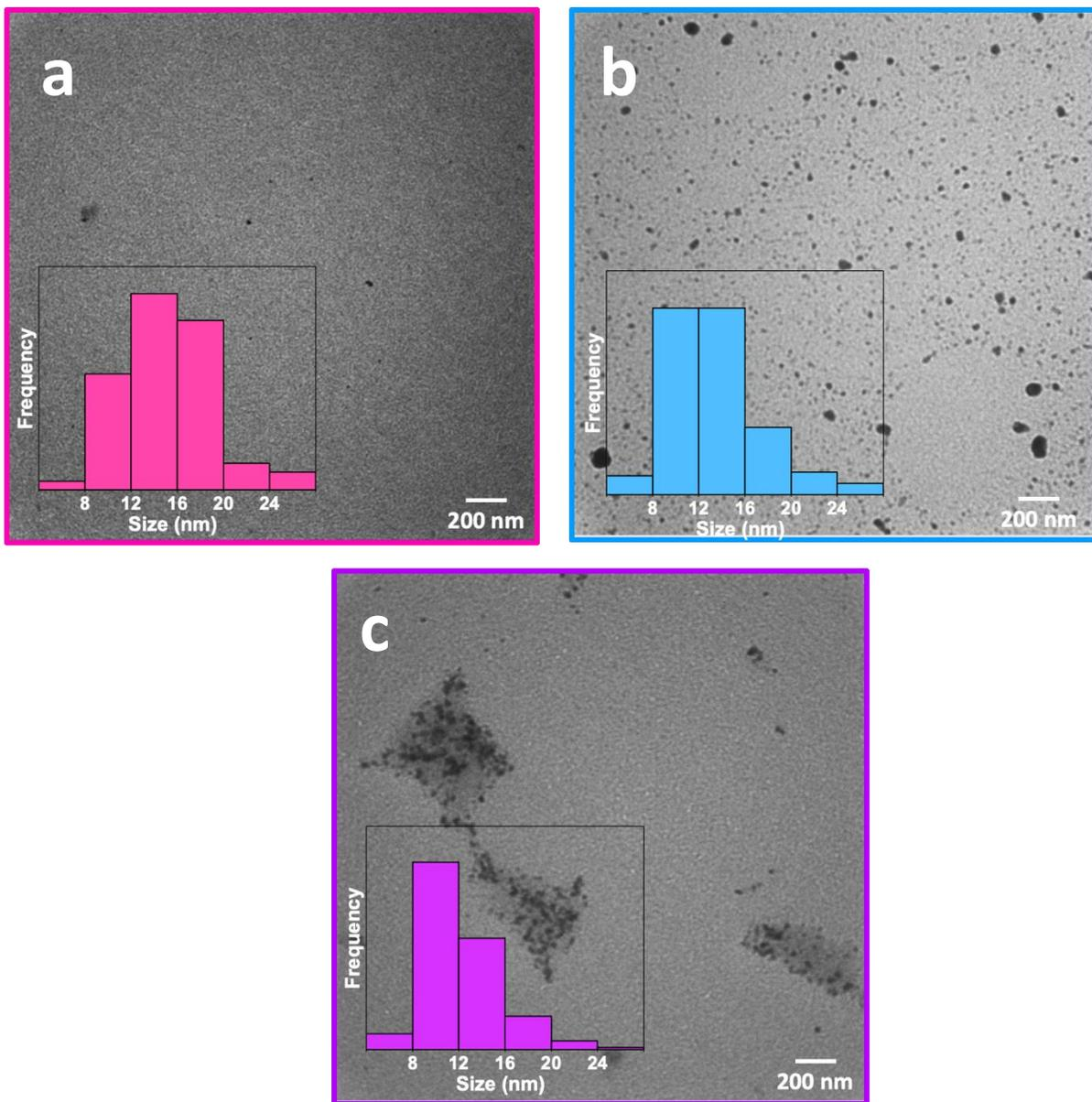
**Figure S3.** TEM images of cysCDs at different reaction times. TEM images of cysCDs synthesized at 160 °C and different reaction times at 5 mins (a), 10 mins (b), and 15 mins (c). The cysCDs seem to slightly increase in size as a function of synthesis time.
