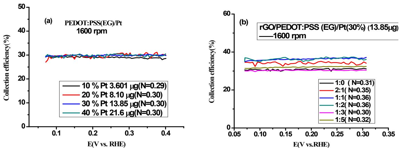
**Fig. S2** Variation of the collection efficiency with potential and catalyst loading for the different catalysts
