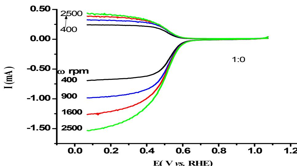
**Fig. S1** Ring ( $\text{Fe}^{2+} \rightarrow \text{Fe}^{3+} + \text{e}^-$ ) and disk ( $\text{Fe}^{3+} + \text{e}^- \rightarrow \text{Fe}^{2+}$ ) currents for the determination of the collection efficiency on 1:0 in 1 M  $\text{KNO}_3$  supporting electrolyte with 10 mM  $\text{K}_3\text{Fe}(\text{CN})_6$ . Negative sweeps at 10 mV s<sup>-1</sup>;  $E_{\text{Ring}} = 1.3$  V.
