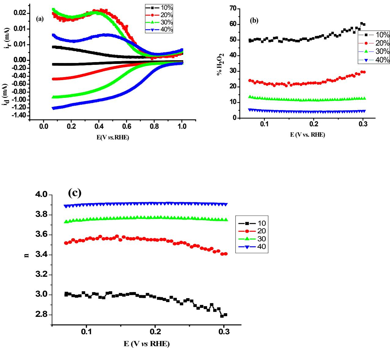
**Fig S3:**(a) RRDE volatmmograms, (b) %  $\text{H}_2\text{O}_2$  formation and (c) electron transfer number ( $n$ )as a function of the disk potential for various platinum loadings PEDOT:PSS(EG) at 1600 rpm in 0.1 M  $\text{HClO}_4$  solution.
