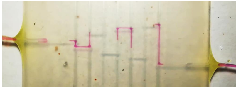
Figure S3: Image of droplets passing through the concatenated flow cell chip (shown schematically in Fig. 3 in the main manuscript). Droplets flowed through without breakup. Here a droplet can be seen filling the entire volume of the largest (10 mm path length) flow cell.
