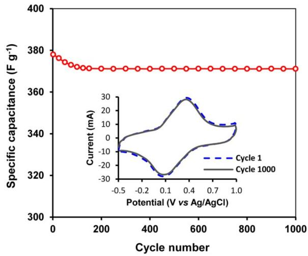
Fig. S6 The dependence of the specific capacitance of the PEDOT-NQS/MWCNT composite on CV cycle numbers within a potential window from  $-0.5$  to  $1.0$  V at a potential scan rate of  $100$  mV s<sup>-1</sup>. The inset exhibits the CV curves at cycle 1 and cycle 1000.
