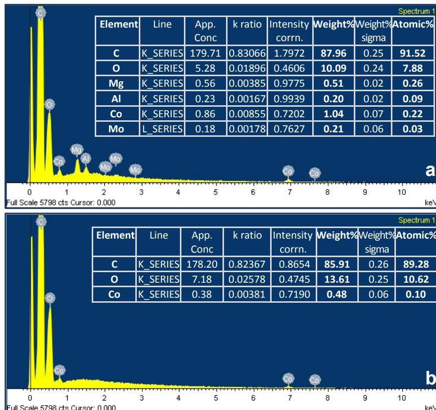
Fig. S1 EDX spectra of untreated (a) and acid-treated (b) MWCNTs.
