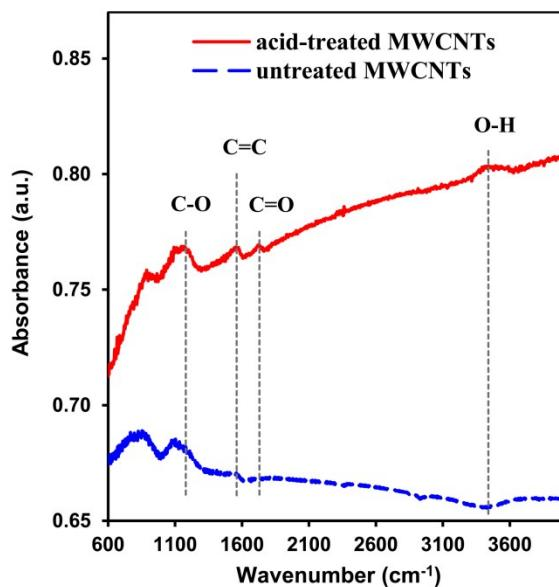
Fig. S2 FTIR spectra of untreated and acid-treated MWCNTs.
