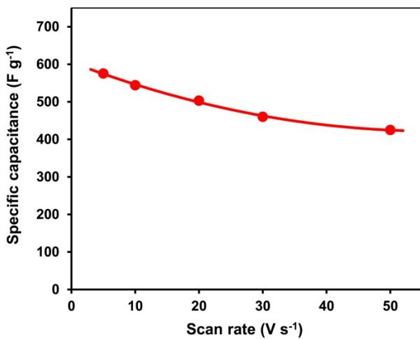
Fig. S5 The specific capacitance of the PEDOT-NQS/MWCNT composite as a function of the potential scan rate.
