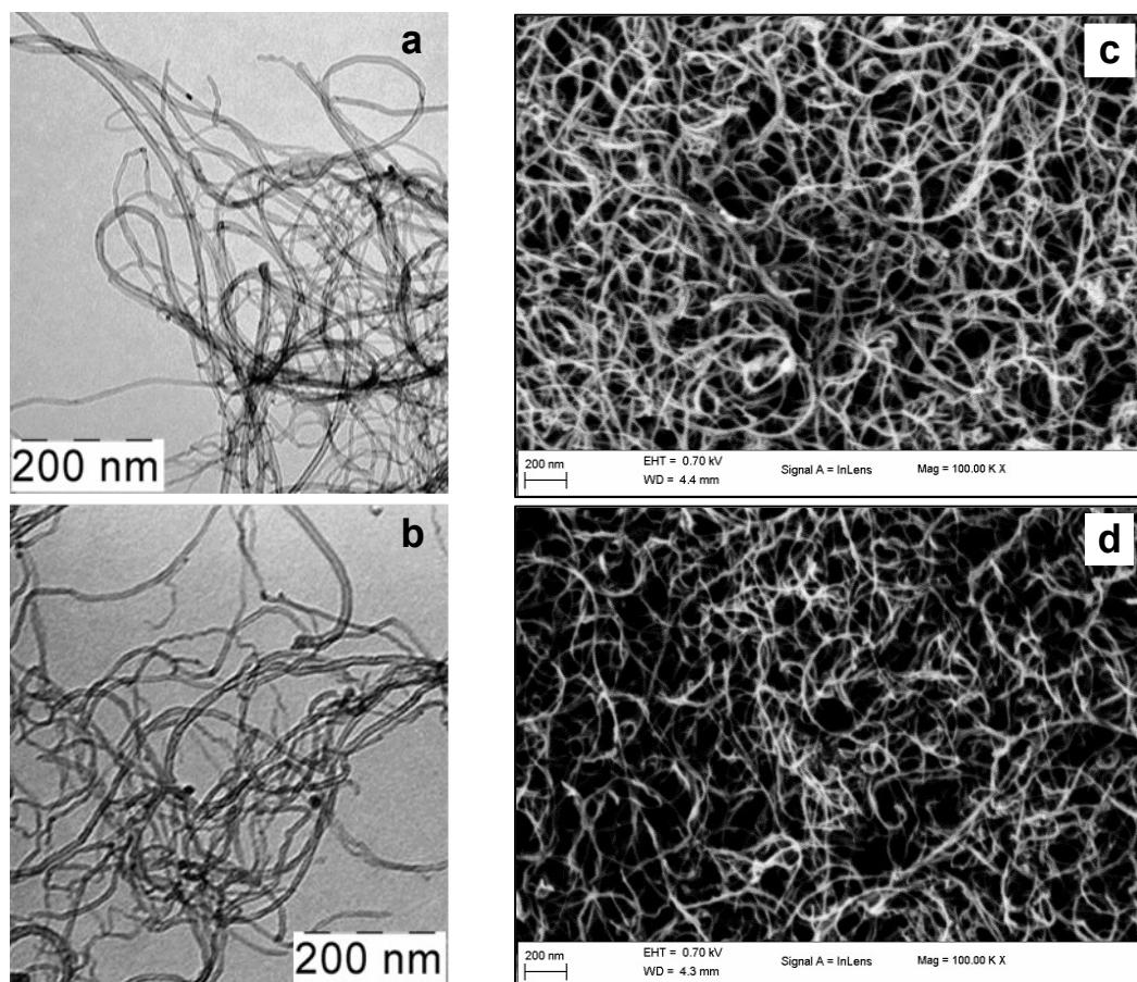
Fig. S3 TEM and SEM images of untreated (a,c) and acid-treated (b,d) MWCNTs.
