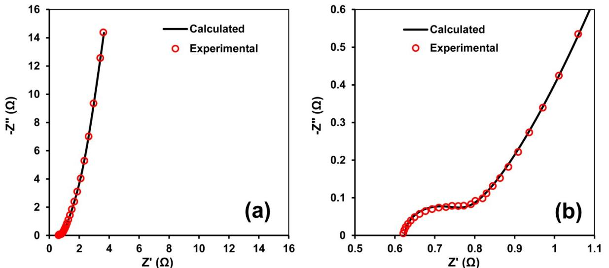
Fig. S7 (a) Comparison of the experimental EIS spectrum at  $0.235$  V (hollow circles) and the spectrum calculated by the equivalent circuit (solid line). (b) The plot shows the extended high-frequency region.
