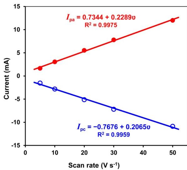
Fig. S4 The linear dependence of the cathode and anode currents of couple II of redox peaks on the scan rate.
