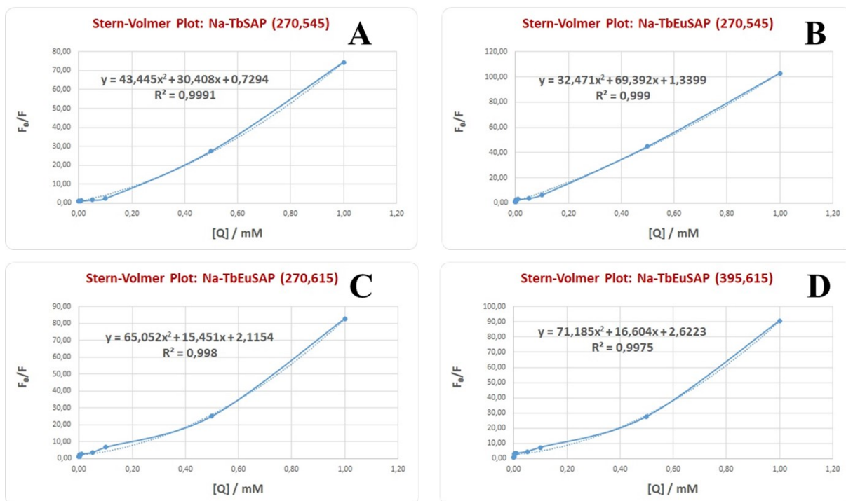
Fig. S7. Non-linear Stern-Volmer plots of F_0/F vs \text{CrO}_4^{2-} concentrations for: A) Na-TbSAP ( \lambda_{\text{exc}} = 270 nm, \lambda_{\text{em}} = 545 nm), B) Na-TbEuSAP ( \lambda_{\text{exc}} = 270 nm, \lambda_{\text{em}} = 545 nm), C) Na-TbEuSAP ( \lambda_{\text{exc}} = 270 nm, \lambda_{\text{em}} = 615 nm) and D) Na-TbEuSAP ( \lambda_{\text{exc}} = 395 nm, \lambda_{\text{em}} = 615 nm). The curves fitting is reported for each graph, together with their second-order polynomial (quadratic) equations and R^2 .
