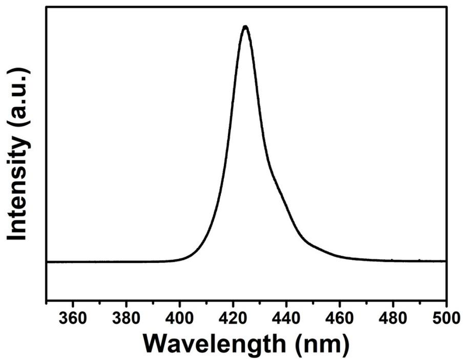
Fig. S1. The light spectrum of LED lamp (30 W).
