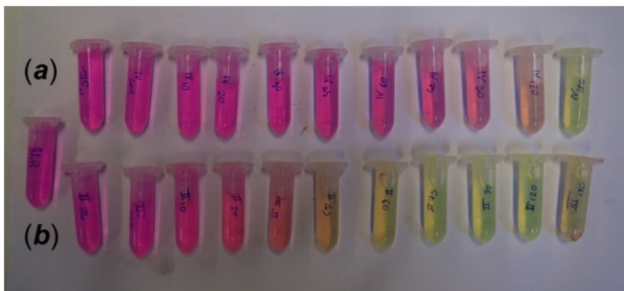
Figure S21: Image of the appearance of Rhodamine solution samples following degradation experiments performed using selected FMS TiO 2 sub-microspheres under visible light: (a) 0.5M HNO 3 /160 mM TTIP and (b) 1M HNO 3 /40 mM TTIP. All samples were subjected to 1 min of MW irradiation time.
