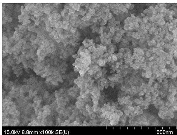
**Figure S2:** SEM image of  $SiO_2$  nanoparticles, dissolved in ethanol and dried on a substrate.
