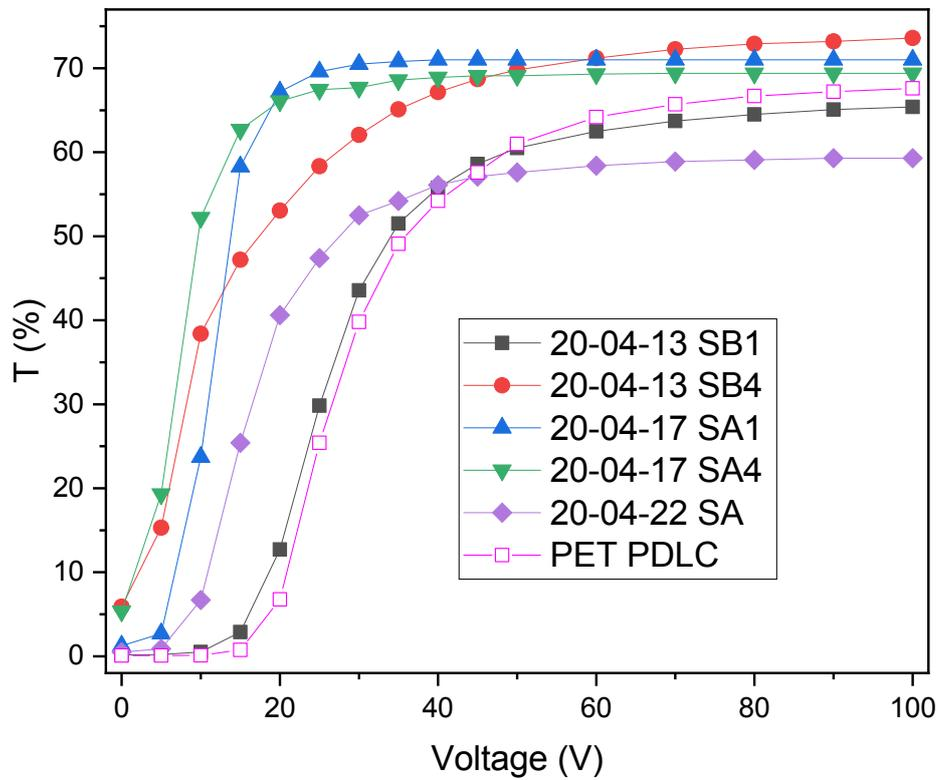
**Figure S4:** Transmittance-versus-voltage curves for various PDLC samples fabricated in different conditions, as shown in Table S1.
