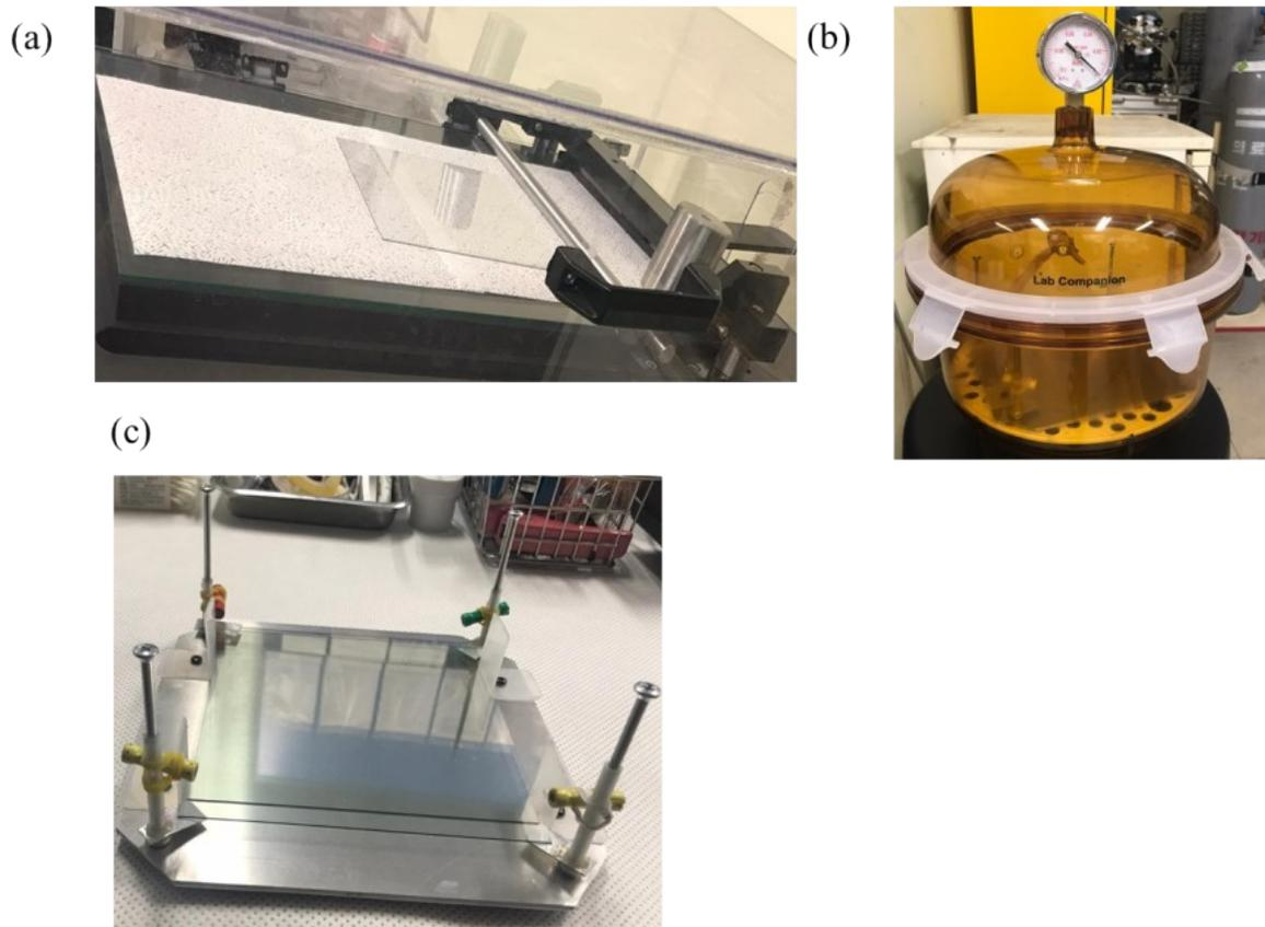
**Figure S3:** (a) Wire-bar coater was used to coat the PDLC mixture. (b) In a vacuum chamber a vacuum assembly holds the top and bottom glasses for vacuum coupling. (c) Vacuum assembly was designed to hold the top and bottom glasses for vacuum coupling.
