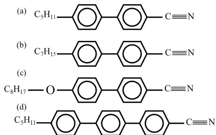
**Figure S1:** Chemical Structure of LC E7 where (a) 4-pentyl-4'-cyanobiphenyl (51%), (b) 4-heptyl-4'-cyanobiphenyl (25%), (c) 4-octyloxy-4'-cyanobiphenyl (16%), and (d) 4-pentyl-4'-cyanobiphenyl (8%) are mixed.
