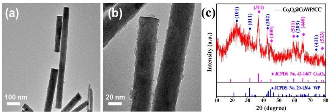
Fig. S8. (a, b) TEM and (c) XRD pattern of  $\text{Co}_3\text{O}_4@\text{CoWP}/\text{CC}$  after 24 h continuous electrolyzing at  $10 \text{ mA cm}^{-2}$  for HER.
