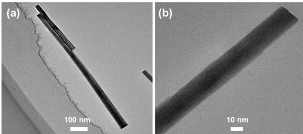
**Fig. S4.** TEM images of Co-WP/CC in (a) low magnification (b) high magnification.
