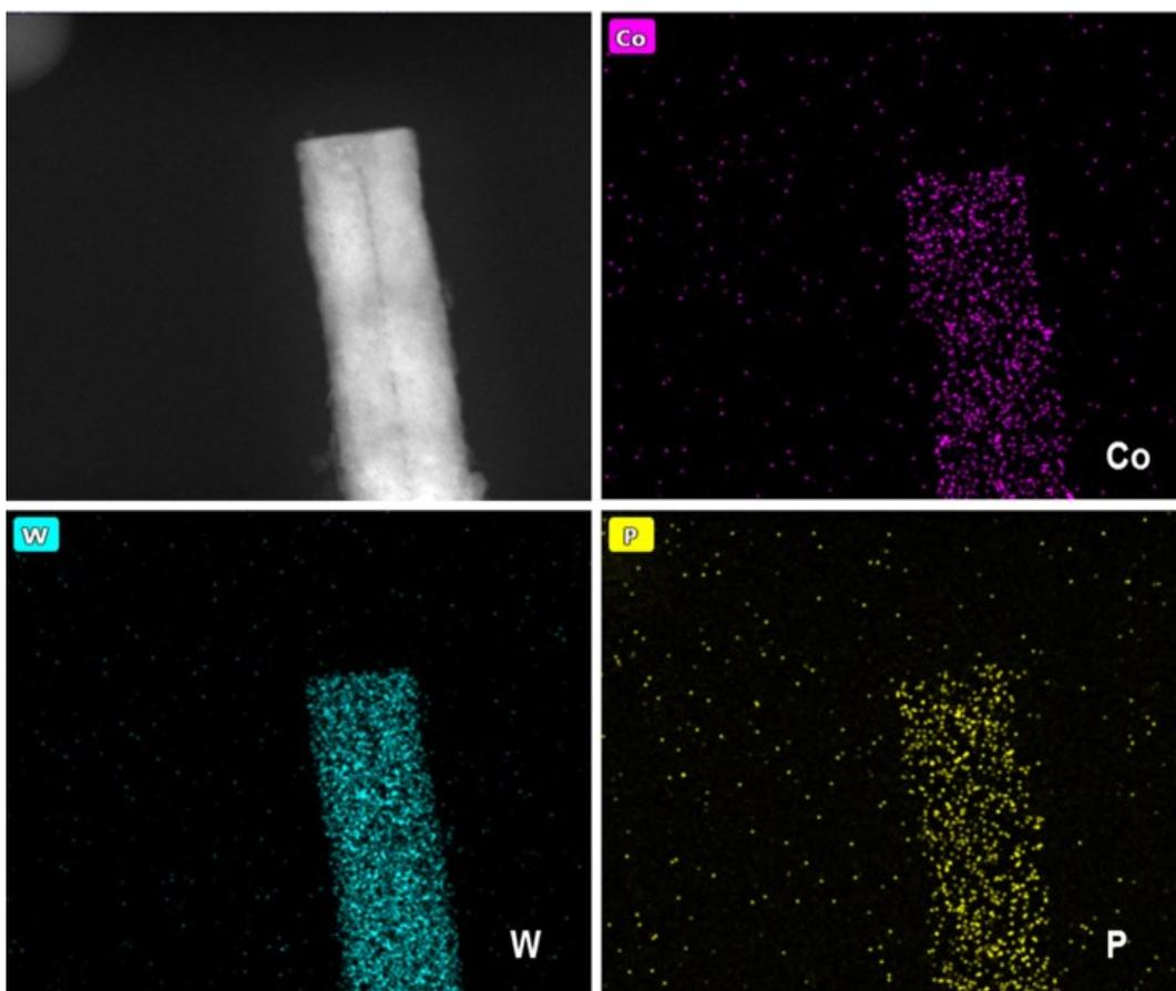
**Fig. S5.** HAADF-STEM image and its corresponding element mapping images of the CoWP/CC.
