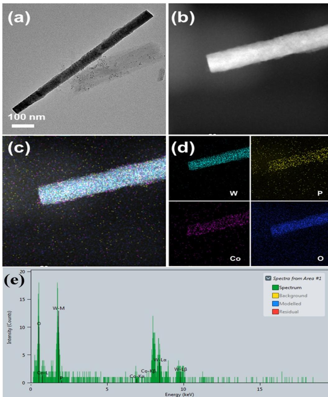
**Fig. S9.** (a) TEM image, (b-d) HAADF-STEM images with the element mapping images, and (e) EDS spectrum of the  $\text{Co}_3\text{O}_4@\text{CoWP}/\text{CC}$  after 24 h continuous electrolyzing at  $10 \text{ mA cm}^{-2}$ .
