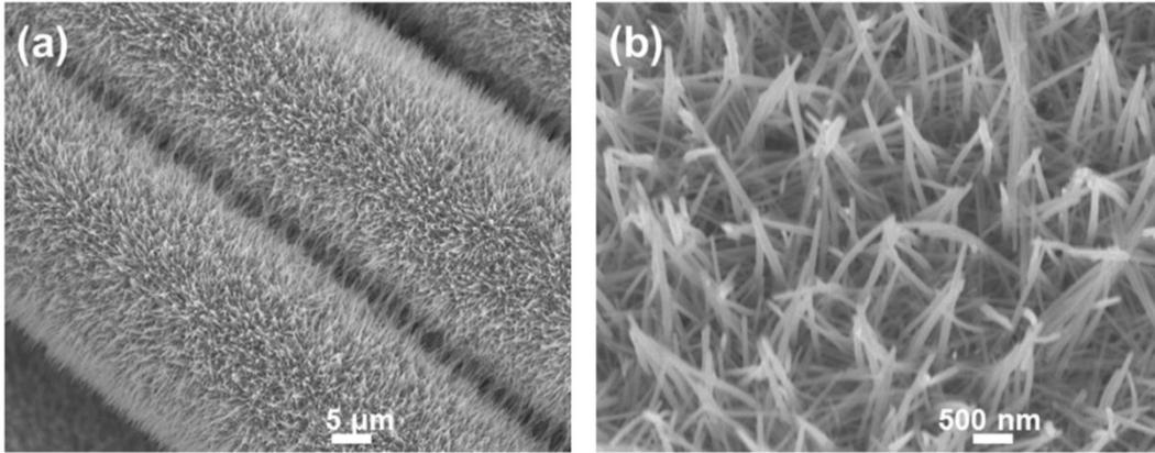
**Fig. S3.** SEM images of CoWO/CC (a) the whole morphology, (b) enlarged image.
