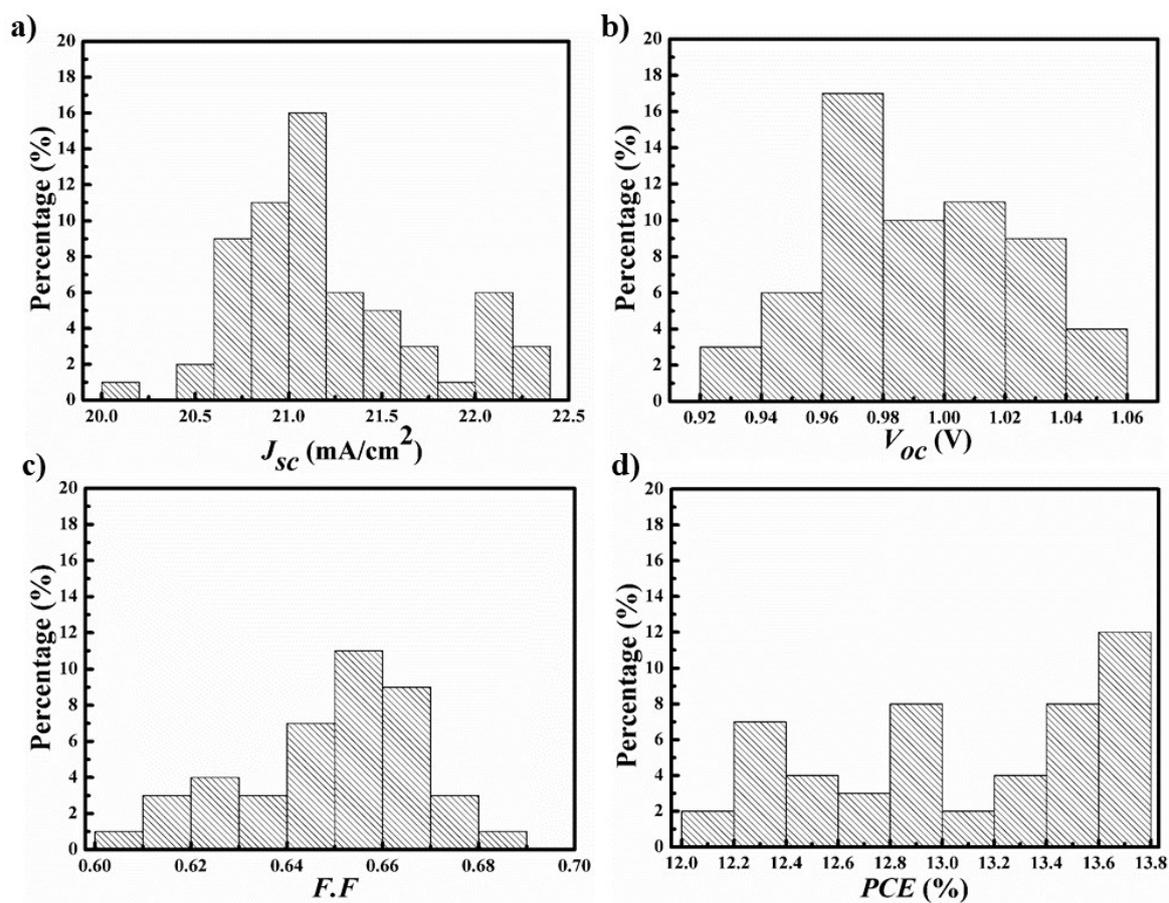
**Figure S7:** Device performances statistics based on more than 200 individuals with  $\text{MAPbI}_{3-x}\text{Cl}_x$  perovskite layers fabricated via a simple all-dip-coating approach in 0.90-MACl/MAI under the optimized conditions.
