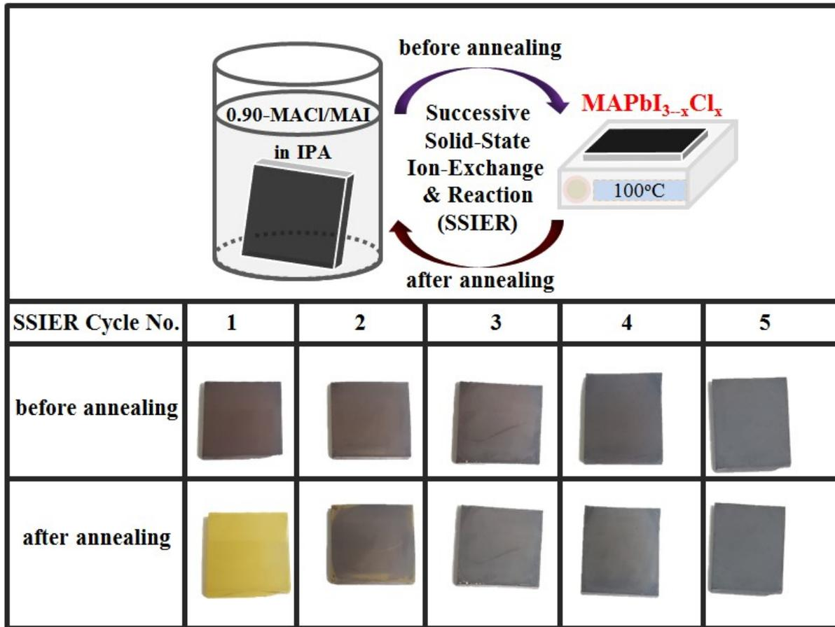
**Figure. S4:** Photographic images of  $\text{MAPbI}_{3-x}\text{Cl}_x$  perovskite material deposited by sequentially dipping a ZnO-covered  $\text{TiO}_2/\text{FTO}$  substrate in aqueous  $\text{Pb}(\text{NO}_3)_2$  and 0.90-MACI/MAI mixed solutions followed by repetition of the SSIER process before/after annealing at  $100^\circ\text{C}$ .
