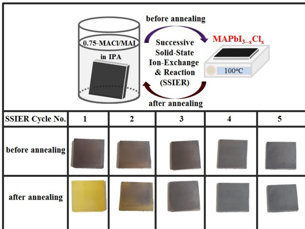
**Figure. S3:** Photographic images of  $\text{MAPbI}_{3-x}\text{Cl}_x$  perovskite material deposited by sequentially dipping a ZnO-covered  $\text{TiO}_2/\text{FTO}$  substrate in aqueous  $\text{Pb}(\text{NO}_3)_2$  and 0.75-MACI/MAI mixed solutions followed by repetition of the SSIER process before/after annealing at  $100^\circ\text{C}$ .
