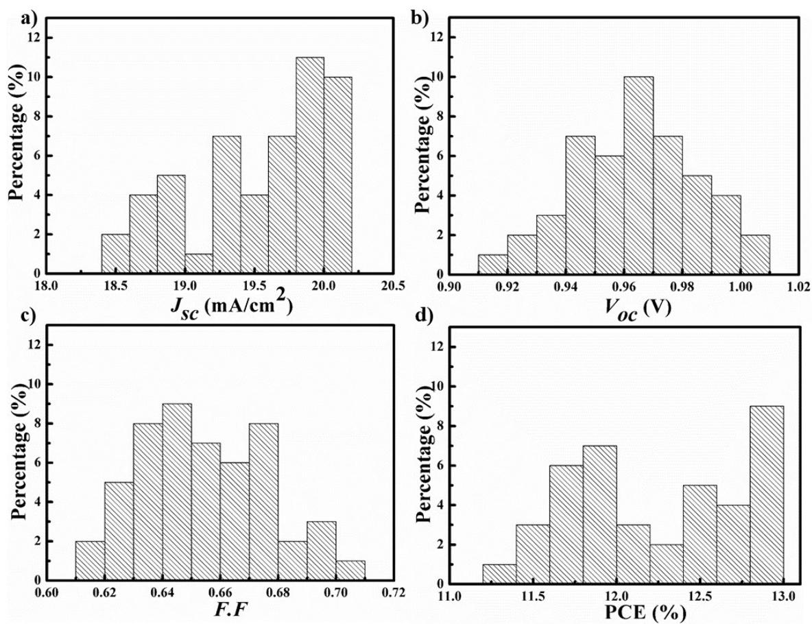
**Figure S5:** Device performances statistics based on more than 200 individual with  $\text{MAPbI}_{3-x}\text{Cl}_x$  perovskite layers fabricated via a simple all-dip-coating approach in 0.45-MACI/MAI under the optimized conditions.
