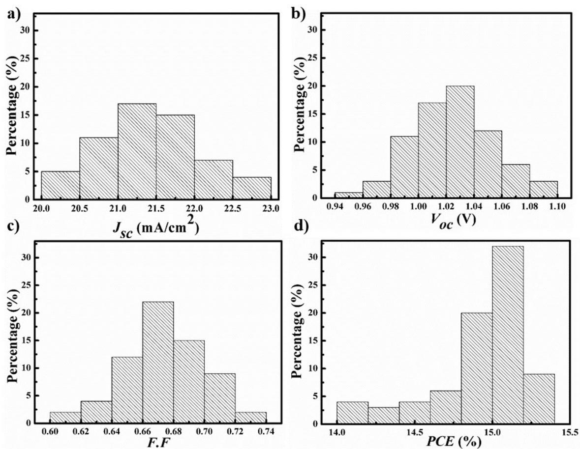
**Figure S6:** Device performances statistics based on more than 200 individuals with  $\text{MAPbI}_{3-x}\text{Cl}_x$  perovskite layers fabricated via a simple all-dip-coating approach in 0.75-MACI/MAI under the optimized conditions.
