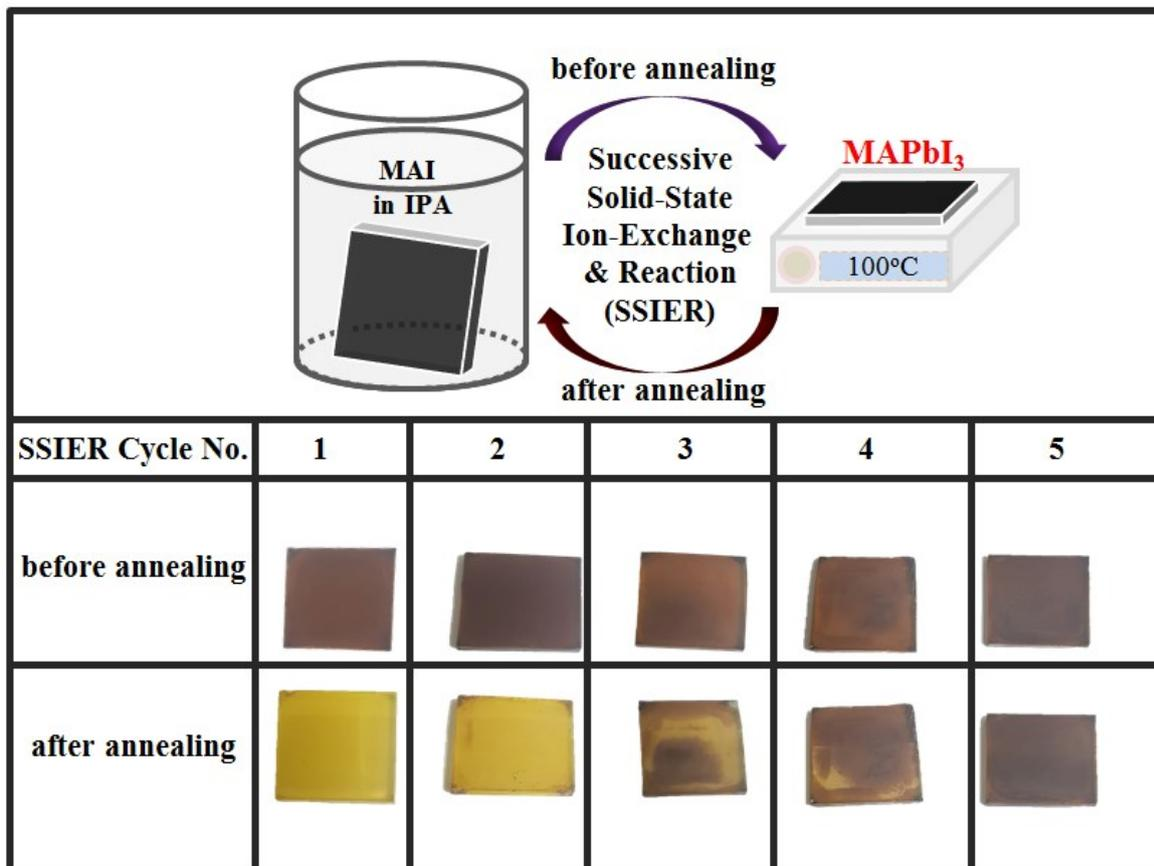
**Figure. S1:** Photographic images of MAPbI<sub>3</sub> perovskite material deposited by sequentially dipping a ZnO-covered TiO<sub>2</sub>/FTO substrate in aqueous Pb(NO<sub>3</sub>)<sub>2</sub> and MAI mixed solutions followed by repetition of the SSIER process before/after annealing at 100°C
