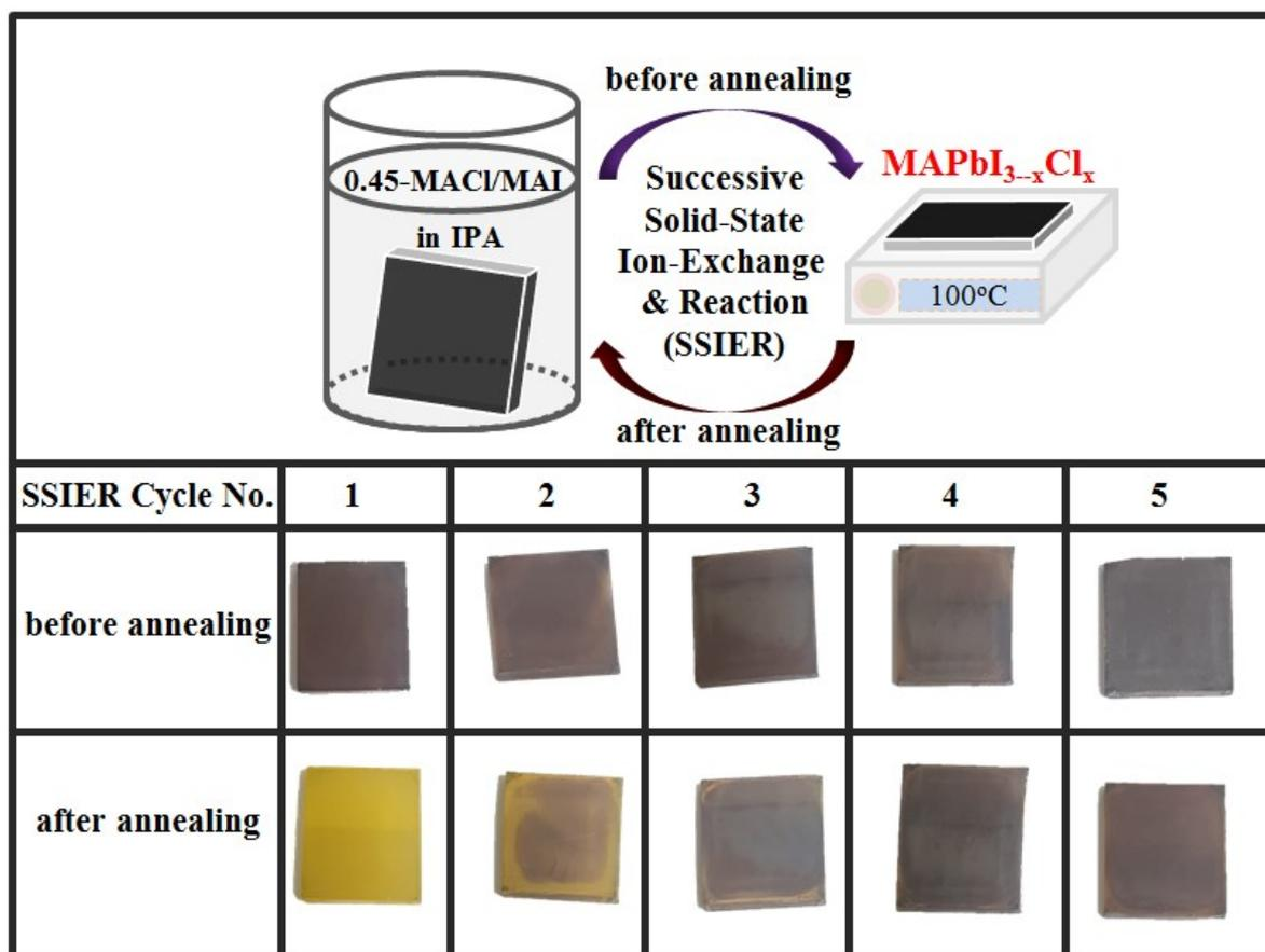
**Figure. S2:** Photographic images of  $\text{MAPbI}_{3-x}\text{Cl}_x$  perovskite material deposited by sequentially dipping a ZnO-covered  $\text{TiO}_2/\text{FTO}$  substrate in aqueous  $\text{Pb}(\text{NO}_3)_2$  and 0.45-MACI/MAI mixed solutions followed by repetition of the SSIER process before/after annealing at  $100^\circ\text{C}$ .
