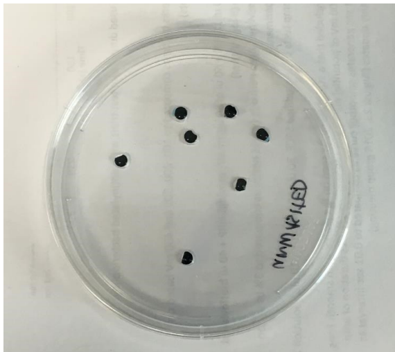
Figure S3. Agar diffusion test of bacteriophage-modified SPCE. (A) Biotinylated O179 bacteriophages were immobilized onto the surface of the trimmed activated working electrode (WE) (B) After several washing and incubation steps prior to agar diffusion assay, WE showed zone of the clearing.
