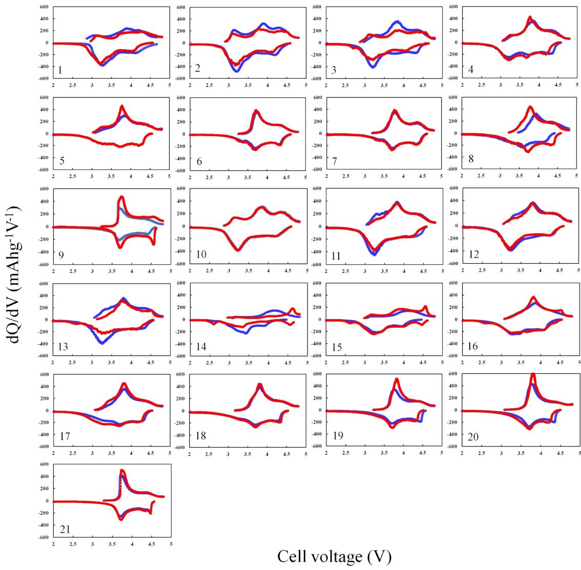
**Fig. S4**  $dQ/dV$  vs. cell voltage curves obtained from charging/discharging curves at the 10<sup>th</sup> cycle. Blue and red curves correspond to the samples prepared by the quenched cooling and slow cooling processes, respectively. The number in each figure indicates the corresponding sample number in Table 1
