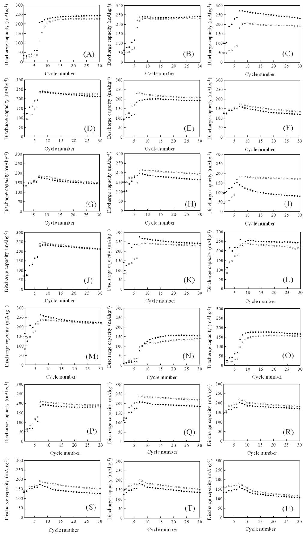
**Fig. S5** Charging/discharging cycle performance obtained at a charging/discharging current density of 0.1 C-rate for the LLO samples prepared by (●) the quenched cooling with liquid nitrogen and (○) the slow cooling in the furnace at a controlled rate of 25 °C h<sup>-1</sup>. Samples: 1 (A), 2 (B), 3 (C), 4 (D), 5 (E), 6 (F), 7 (G), 8 (H), 9 (I), 10 (J), 11 (K), 12 (L), 13 (M), 14 (N), 15 (O), 16 (P), 17 (Q), 18 (R), 19 (S), 20 (T) and 21 (U).
