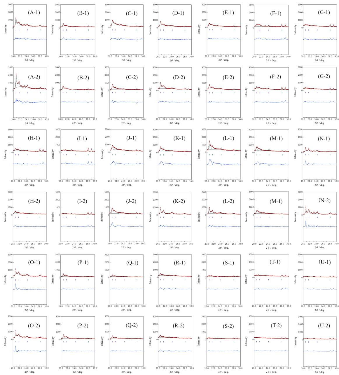
**Fig. S7** XRD Rietveld refinement profiles from 20 to 30° of the LLO samples prepared by (1) the quenched cooling with liquid nitrogen and (2) the slow cooling in the furnace at a controlled rate of 25 °C h<sup>-1</sup>. (—) observed, (—) calculated, (—) the difference of both. The vertical marks indicate the position of the Bragg reflections. (A) sample 1, (B) sample 2, (C) sample 3, (D) sample 4, (E) sample 5, (F) sample 6, (G) sample 7, (H)
