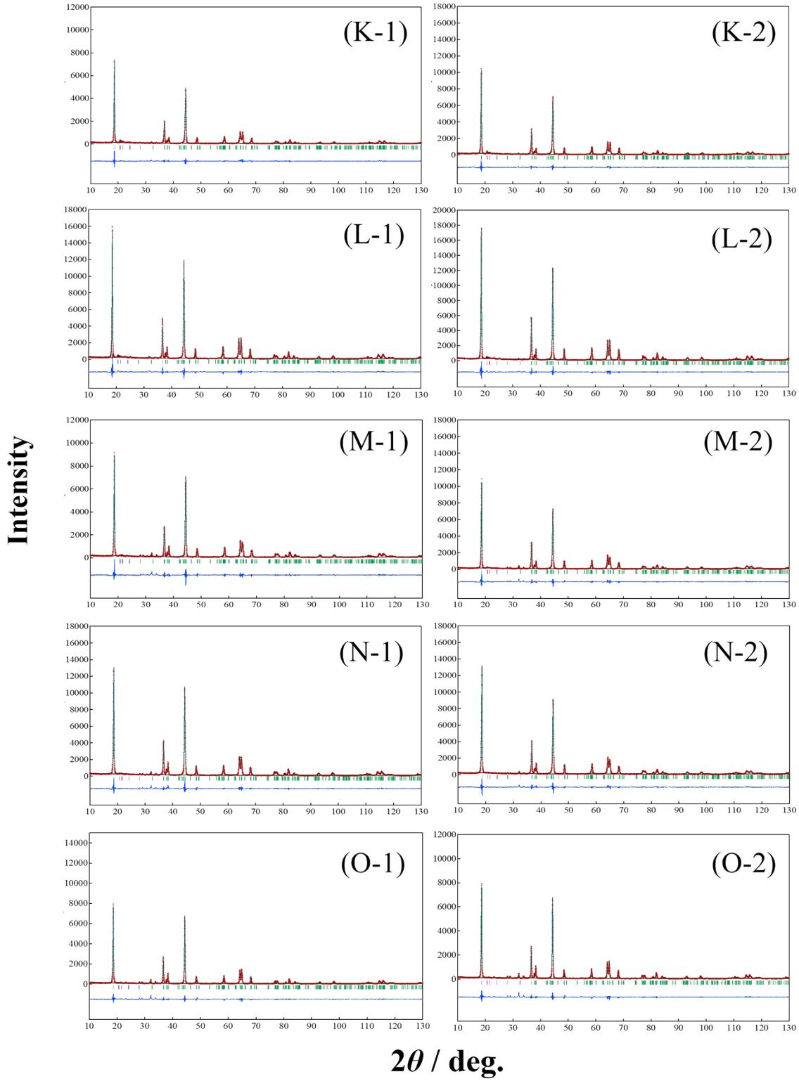
**Fig. S6** XRD Rietveld refinement profiles of samples prepared by (1) the quenched cooling with liquid nitrogen and (2) slow cooling in the furnace at a controlled rate of 25
