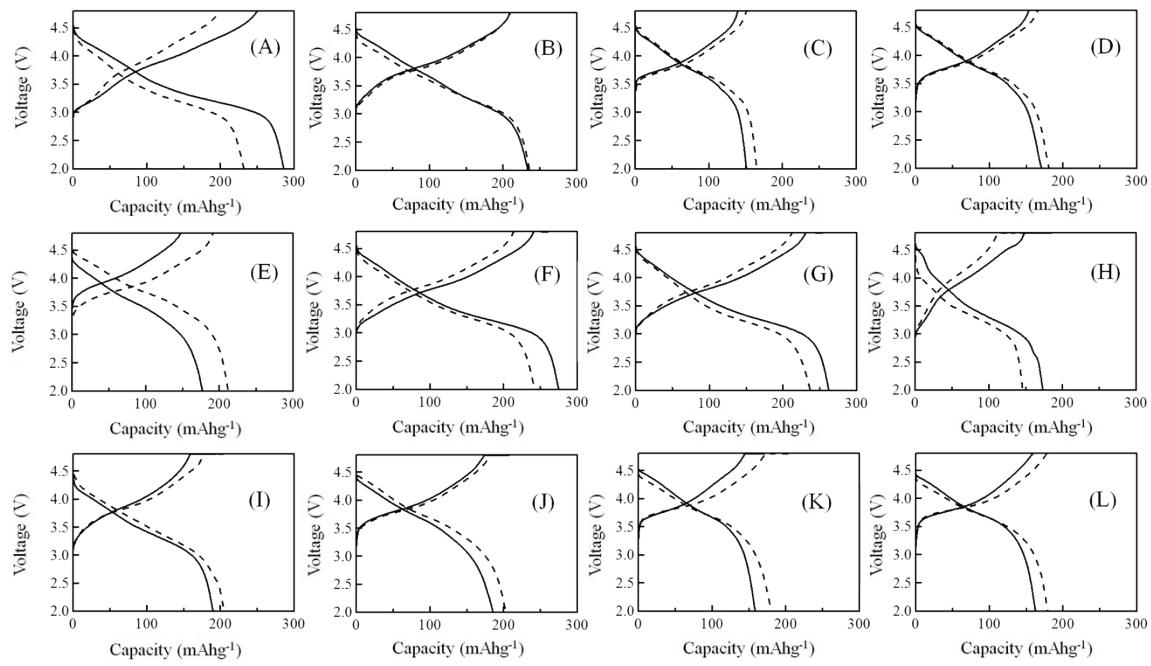
**Fig. S3** Charging/discharging voltage-capacity curves obtained at the 10<sup>th</sup> cycle with samples 2 (A), 4 (B), 6 (C), 7 (D), 8 (E), 11 (F), 12 (G), 15 (H), 16 (I), 18 (J), 19 (K), and 20 (L) prepared by the quenched cooling with liquid nitrogen (solid lines) and the slow cooling in the furnace at a controlled rate of 25 °C h<sup>-1</sup> (dotted lines). The charging/discharging rate was 0.1 C.
