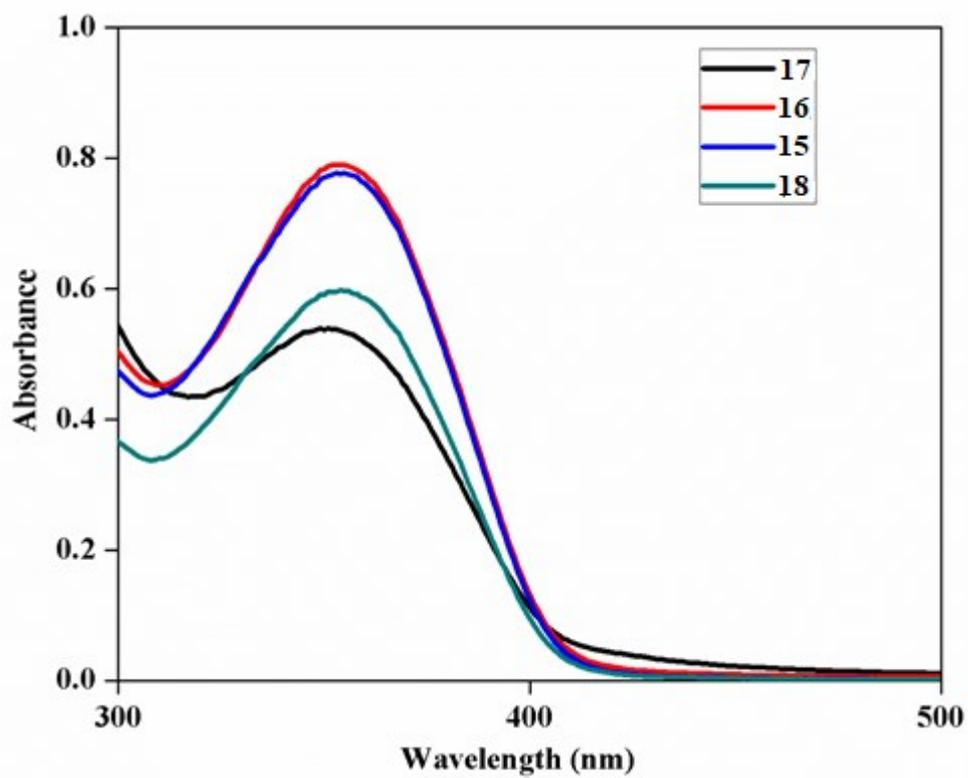
**Figure S12.** UV-vis spectra for quantification of nimodipine encapsulation in amphiphiles 15-
