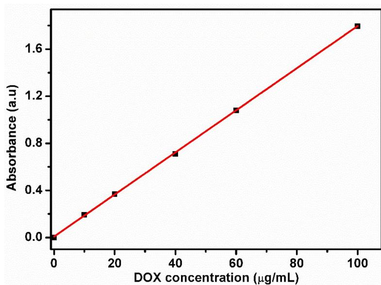
**Figure S4** Absorbance at 480 nm vs. free DOX concentration (optical path = 1 cm). Solid line is the liner fit using the analysis tool in Origin software and the  $R^2 = 0.9999$ .
