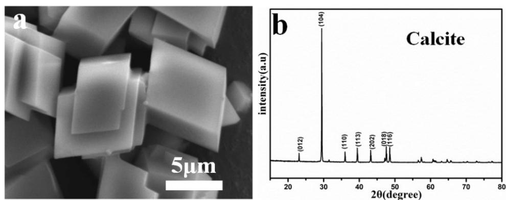
**Figure S3** The SEM and XRD of the CaCO<sub>3</sub> synthesized in the distilled water.
