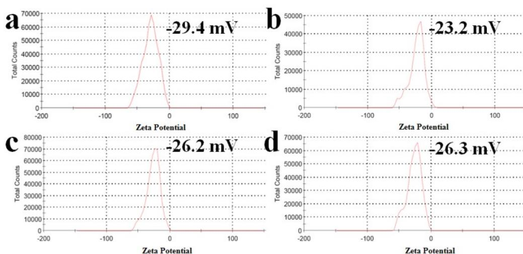
**Figure S2** The zeta potentials of the YC-CaCO<sub>3</sub> NPs with different sizes (from a to d corresponds to the size of 2.3 nm, 3.9 nm, 6.2 nm and 12.2 nm of YC-CaCO<sub>3</sub> NPs, respectively)
