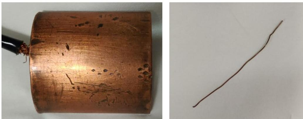
**Supplementary Fig 1:** Copper plate and copper wire used in the synthesis process
