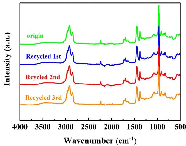
**Figure S5.** Comparison of FTIR spectra of the original and recycled XNBR-50s.
