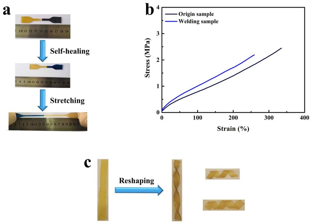
**Figure S9.** (a) Self-healing process of XNBR-50. (b) Stress-strain curves of original sample and the welding sample of XNBR-50. (c) Reshaping plots of XNBR-50.
