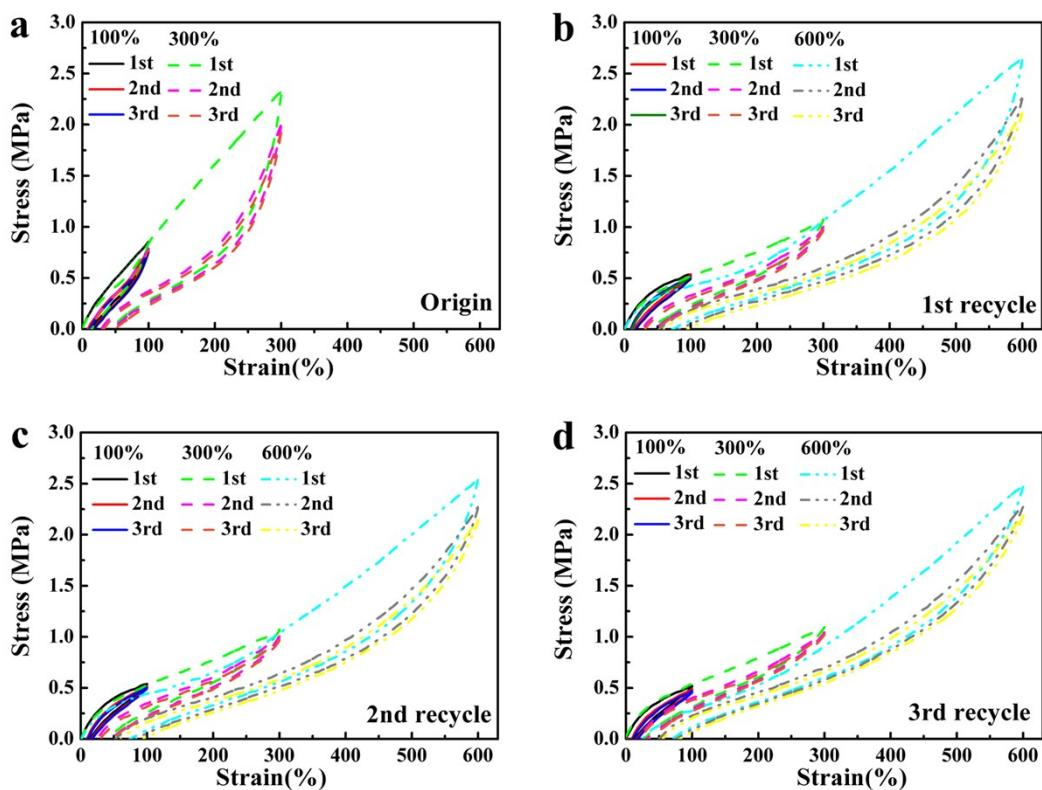
**Figure S8.** Cyclic loading-unloading curves of XNBR-50s at 100%, 300% and 600% strain. (a) Original sample. (b) First recycled sample. (c) Second recycled sample. (d) Third recycled sample.
