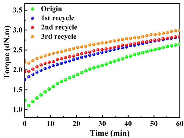
**Figure S4.** Curing curves of the original and recycled XNBR-50s.
