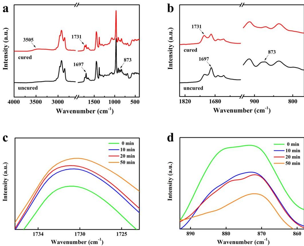
**Figure S3.** (a) FTIR spectra of uncured and cured XNBR-50. (b) Comparison of epoxy (960~700  $\text{cm}^{-1}$ ), carbonyl and carboxyl groups (1800~1550  $\text{cm}^{-1}$ ) of uncured and cured XNBR-50 in the FTIR spectra. (c) Evolution of ester groups, (d) epoxy groups of FTIR spectra during the curing of XNBR-50 at 160 °C.
