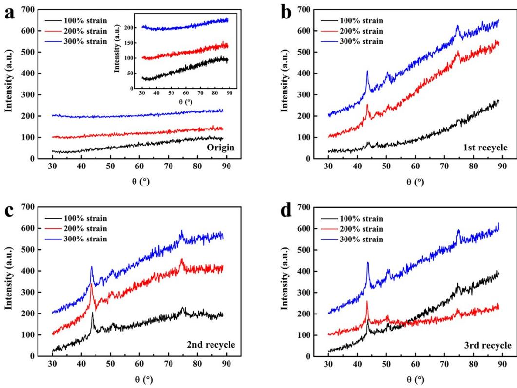
**Figure S6.** XRD curves of XNBR-50s at 100%, 200% and 300% strain. (a) Original sample. (b) First recycled sample. (c) Second recycled sample. (d) Third recycled sample.
