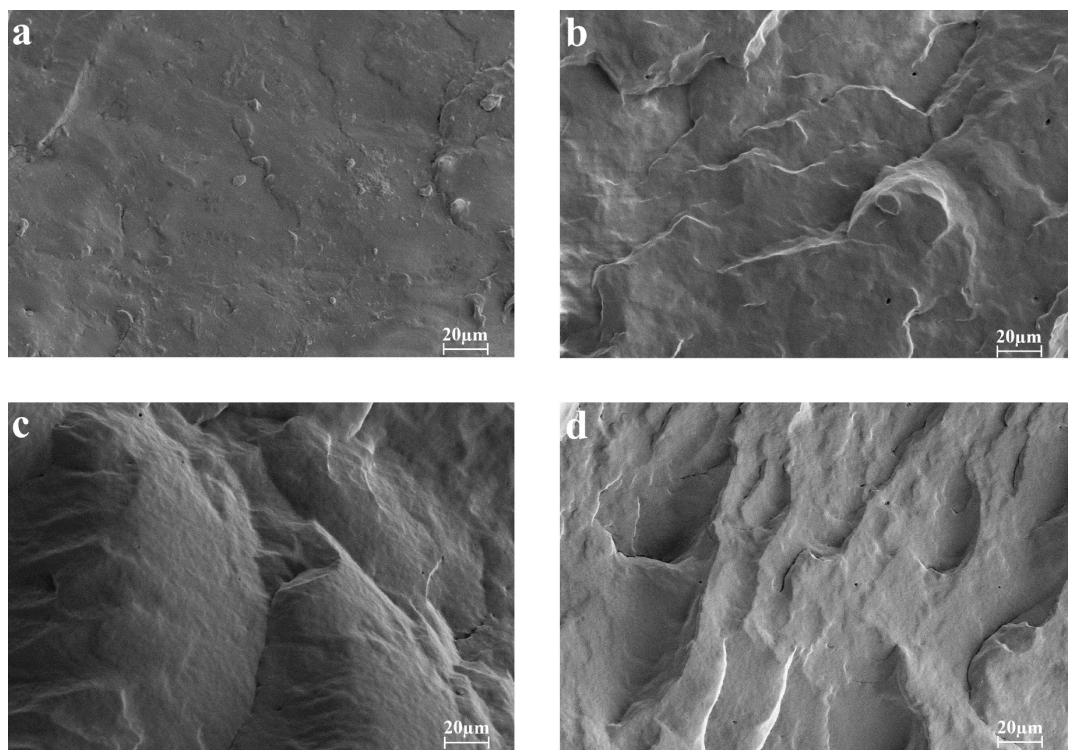
**Figure S7.** SEM images of XNBR-50s. (a) Original sample. (b) First recycled sample.
