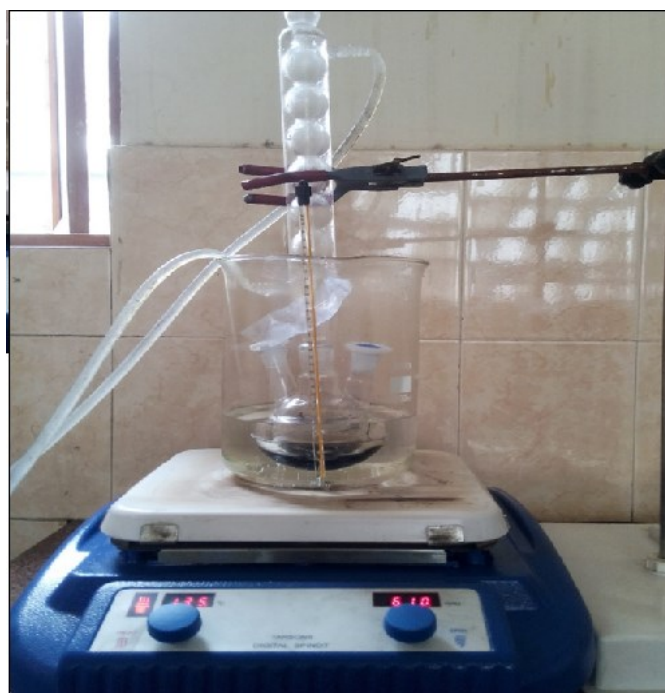
Fig. 2 Batch reactor set up for the ketalization reaction
